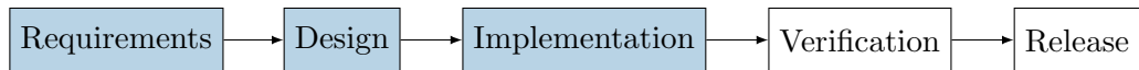
Figure 1.1: The baseline software development process that forms the basis of Microsoft’s Security Development Lifecycle [151]. We highlighted the phases that can gain from a proactive proof of security.
