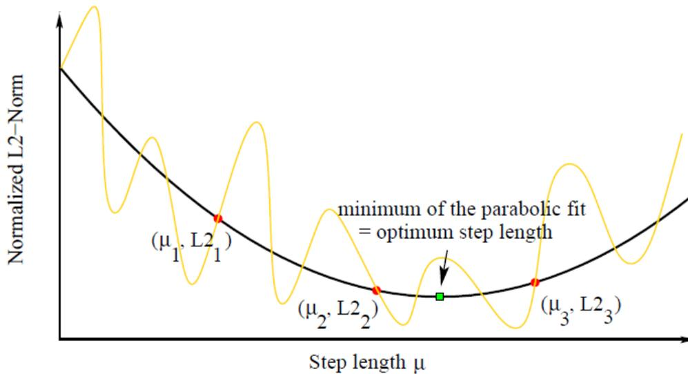
Figure 3.3.: Parabolic line search algorithm. The red dots denote the calculated misfit values as functions of the various step lengths  $\mu_1$ ,  $\mu_2$  and  $\mu_3$ . The yellow curve is a sketch of the misfit function. The green mark is the minimum of the fitted parabola. Source: (Köhn et al., 2013)
