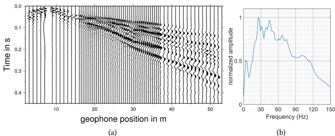
Figure 4.1.: Shot section of source number 5 showing the raw seismic traces (a) and the corresponding normalized amplitude spectrum (b). The traces are normalized by their maximum amplitude.
