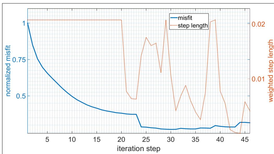
Figure 6.3.: Misfit progress during the inversion of profile one. The blue line denotes the misfit of each iteration step normalized by its maximum. The dotted brownish line defines the applied step length for each iteration step in percent as described in section 3.4.3
