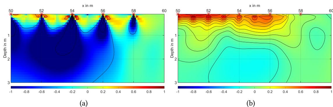
Figure 5.5.: The figure shows a section of the shear-wave gradient model without (a) and with (b) a semi-circular filter applied at the source locations. Red stars mark the locations of the shot positions. The scale is normalized by the maximum amplitude of figure (b) and kept identical in figure (a) in order to emphasize the effect. The remaining high amplitude regions are located at the receiver positions
