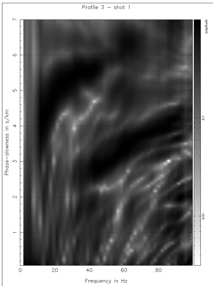
Figure 5.1.: This figure shows the dispersion curve of profile three. Two modes of the Rayleigh wave can be distinguished. The presumed fundamental Rayleigh mode arises from 5 Hz and reaches to 50 Hz. The observed phase velocities of the fundamental mode lie in between 160 and 250 meters per second. A higher mode is visible in the frequency range of 40 to 95 Hz. The phase velocities reach from 220 to 400 meters per second.
