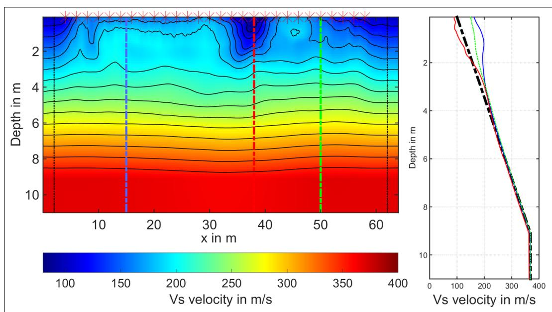
Figure 6.10.: Final S-wave velocity model and corresponding cross sections at selected positions (15 m, 38 m, 50 m). At the edges of the image are perfectly matched layers (PML) marked by a black dashed line, where the forward modeled wavefield is damped to zero. No model update is supposed to happen in this regions.
