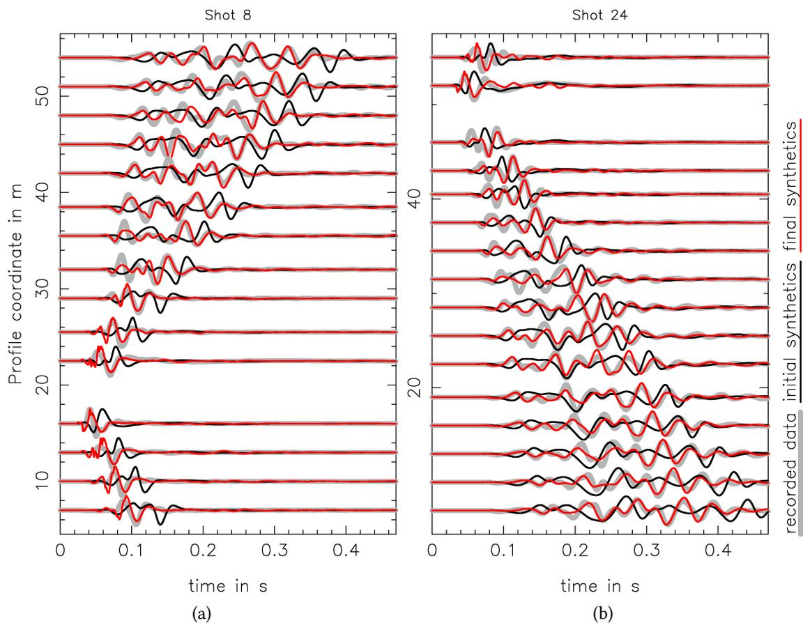
Figure 6.2.: Shot gather of two different shot locations. The grey curve represents the recorded data, black is the initial forward modeled data curve and the red line the fitted synthetic signal after 46 iterations
