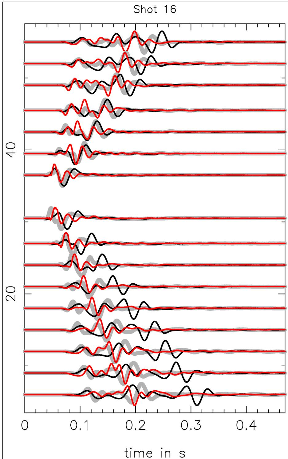
Figure A.2.: Shot gather of the initial model (black), of the inverted final model after 46 iterations (red) and the recorded, real seismograms (grey) of profile two.
