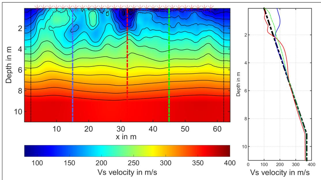
Figure 6.4.: Final model of the S-wave velocities and corresponding cross sections at selected positions (15 m, 32 m, 45 m). At the edges of the image are perfectly matched layers (PML) marked by a black dashed line, where the forward modeled wavefield is damped to zero. No model update is supposed to happen in this regions.
