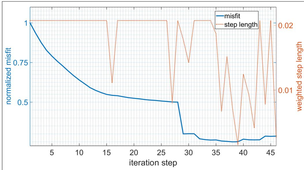
Figure 6.9.: Misfit progress during the inversion of profile two. The blue line denotes the misfit of each iteration step normalized by its maximum. The dotted brownish line defines the applied step length for each iteration step in percent as described in section 3.4.3
