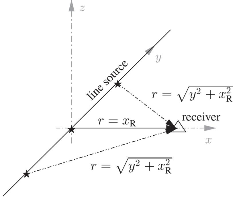
Figure 4.3.: Sketch of the geometrical illustration of the line source.  $x_r$  denotes the receiver position,  $r$  is the distance of each point of the line source to the receiver location and  $y$  denotes the point of the line source. Source: Forbriger et al. (2014)
