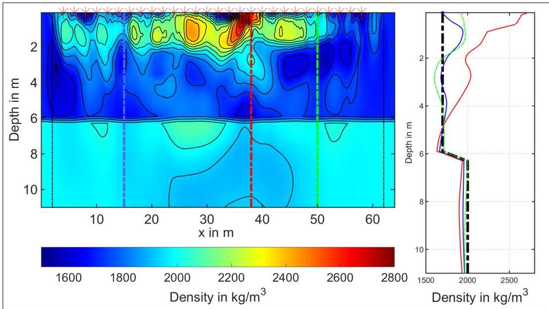
Figure 6.12.: Final density model of profile two and corresponding cross sections at selected positions (15 m, 38 m, 50 m). At the edges of the image are perfectly matched layers (PML) marked by a black dashed line, where the forward modeled wavefield is damped to zero. No model update is supposed to happen in this regions.
