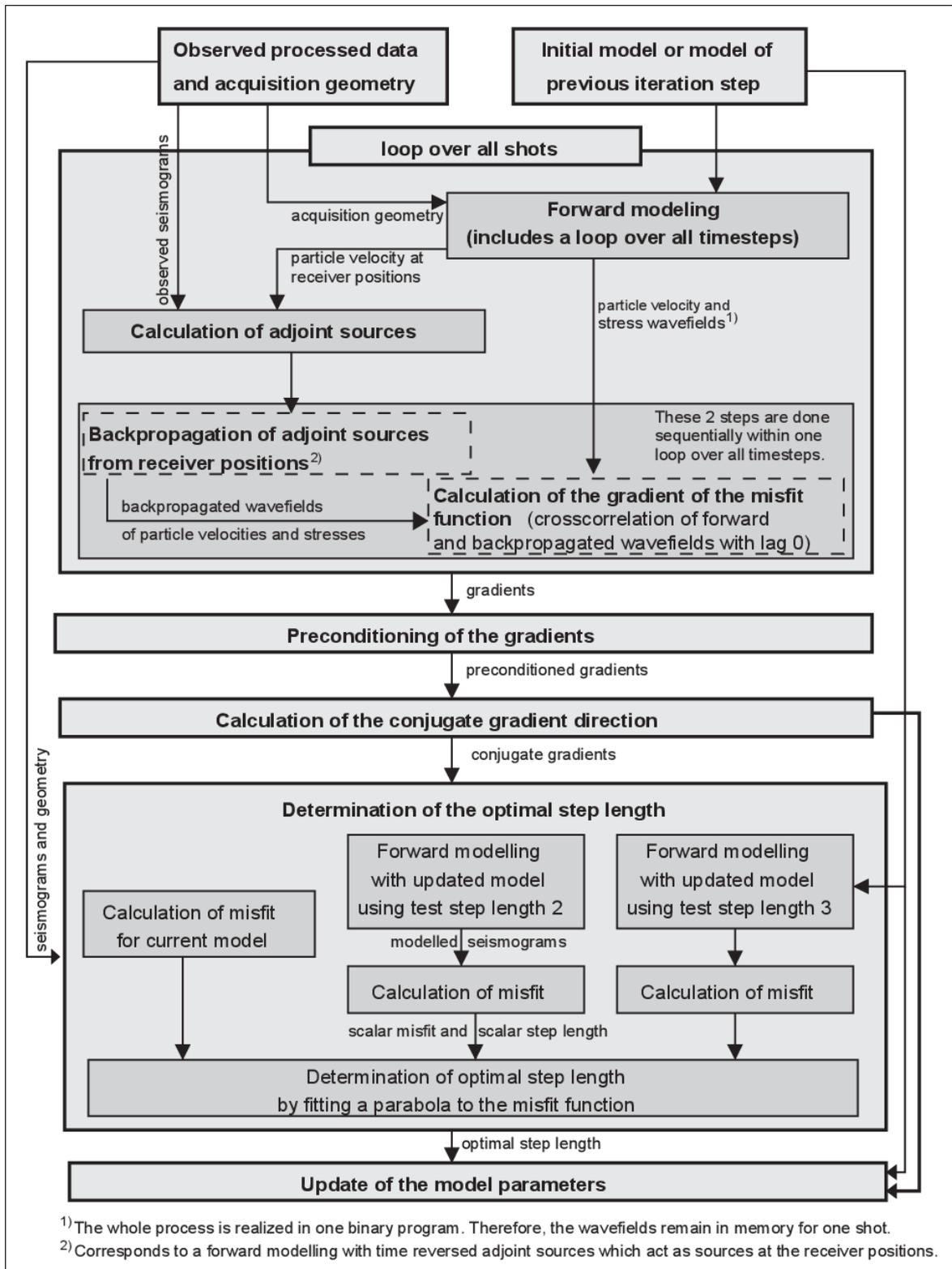
Figure 3.2.: Flow chart of the calculations performed during one iterative process in DENISE. Source:(Groos, 2013).
