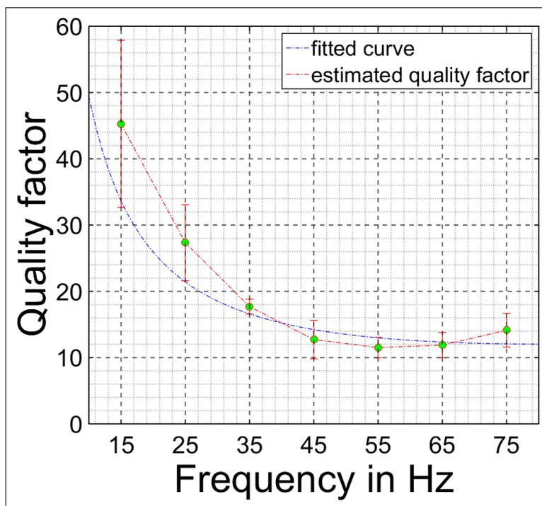
Figure 5.3.: The plot shows the result of the quality factor estimated from the observed data as well as the fitted values used for the inversion algorithm
