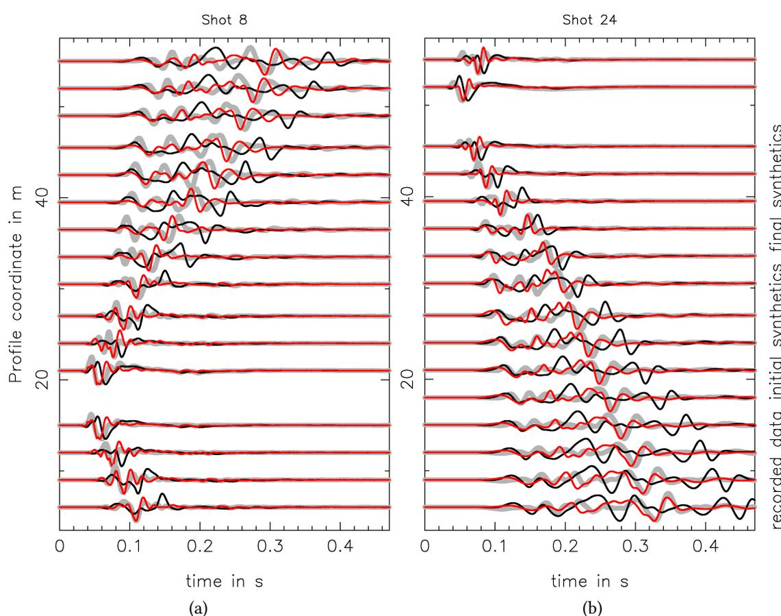
Figure 6.8.: Shot gather of two different shot locations. The grey curve represents the recorded data, black is the initial forward modeled data curve and the red line the fitted synthetic signal after 46 iterations
