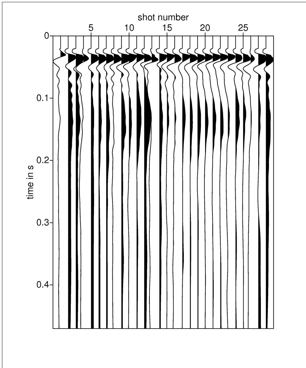
Figure 6.7.: Inverted source time functions of each source at profile 2. The shot numbers correspond to source locations in the field beginning from west to east.
