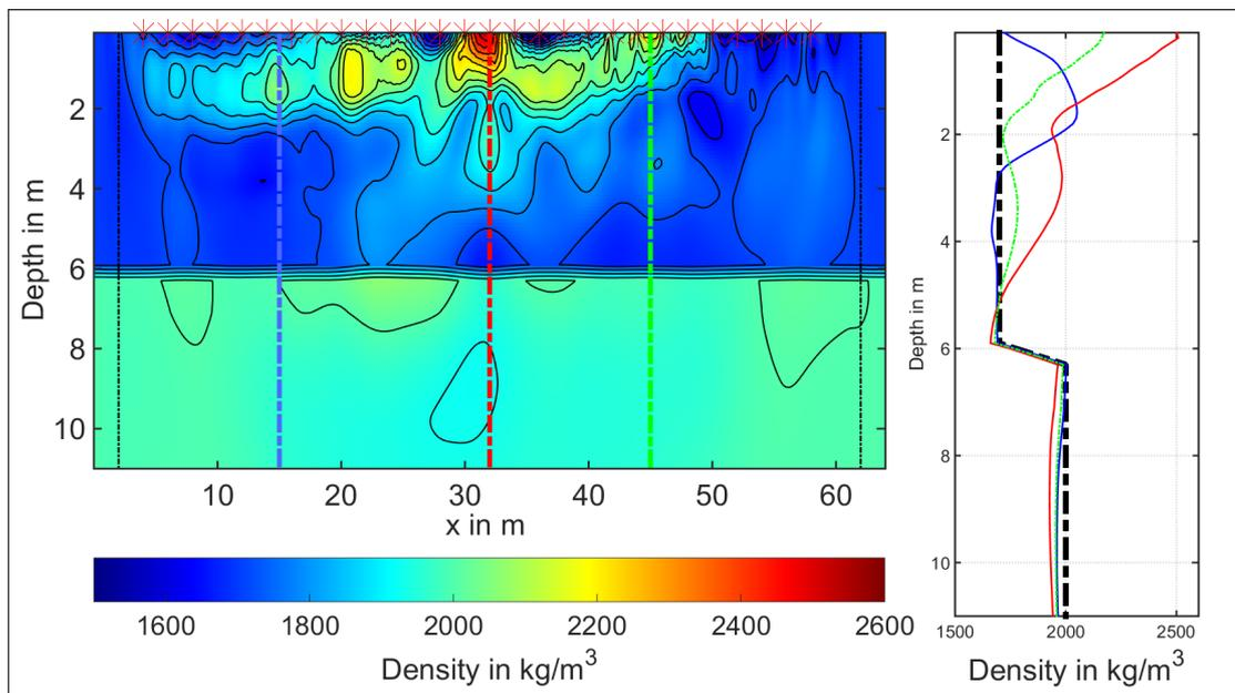
Figure 6.6.: Final model of the mass density and corresponding cross sections at selected positions (15 m, 32 m, 45 m). At the edges of the image are the perfectly matched layers (PML) marked (black dashed lines), where the forward modeled wavefield is damped to zero. No model update is supposed to happen in this areas. The peak value of the density directly at the surface of the Ettliger Linie exceeds 2500 kg per  $m^3$ .
