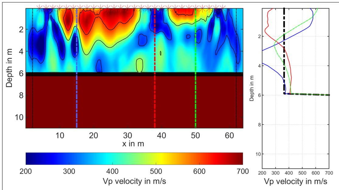
Figure 6.11.: Final P-wave velocity model of profile two and corresponding cross sections at selected positions (15 m, 38 m, 50 m). At the edges of the image are perfectly matched layers (PML) marked by a black dashed line, where the forward modeled wavefield is damped to zero. No model update is supposed to happen in this regions.
