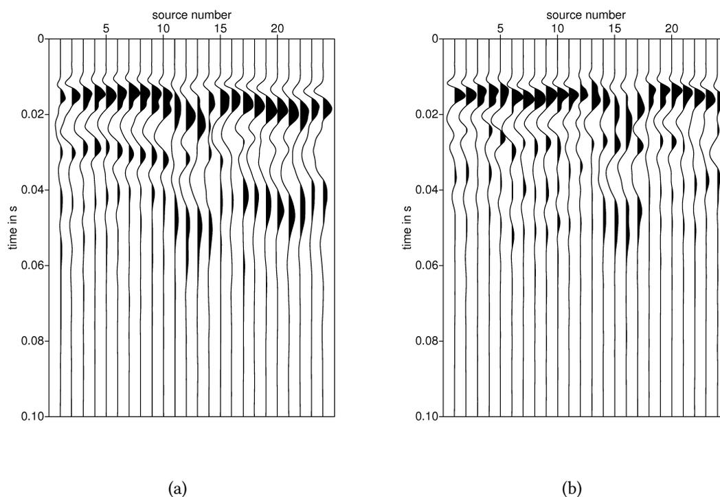
Figure 5.4.: The figure shows the seismic traces 1 meter distant from each of 24 source locations.
