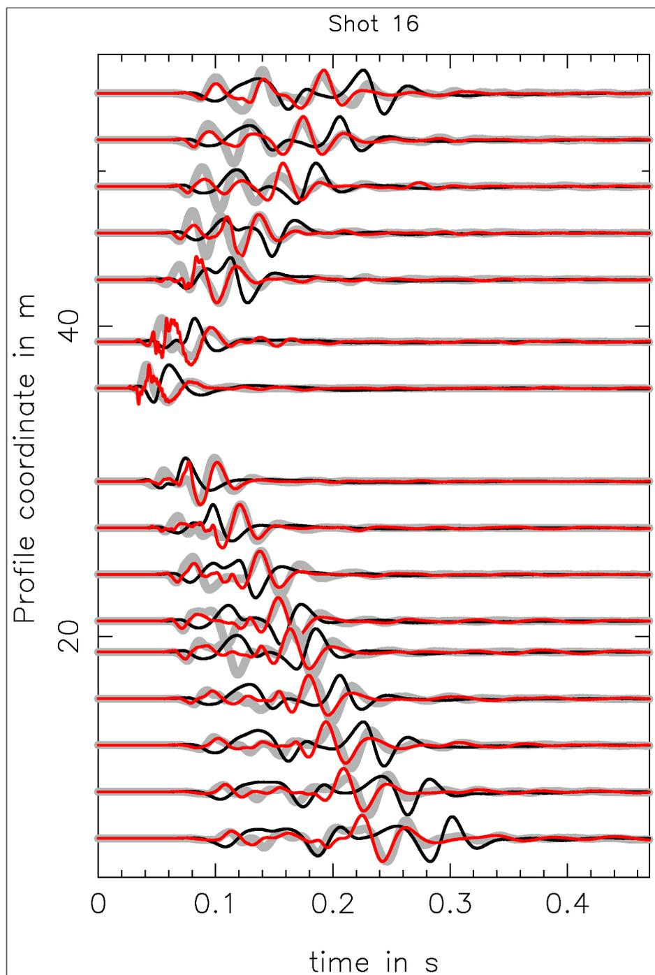
Figure A.1.: Shot gather of the initial model (black), of the inverted final model after 46 iterations (red) and the recorded, real seismograms (grey) of profile one.
