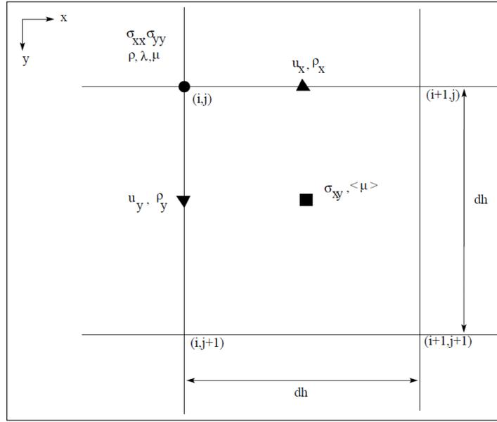
Figure 3.1.: Geometry of the standard staggered grid in two dimensions. Source: Köhn et al. (2013)
