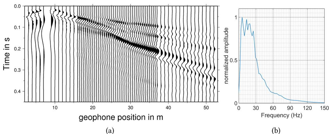
Figure 4.2.: Shot section of source number 5. The seismic traces are filtered with a second order low-pass Butterworth filter with a corner frequency of 5 Hz (a) and the corresponding normalized amplitude spectrum (b). Again, the traces are normalized by their maximum amplitude.
