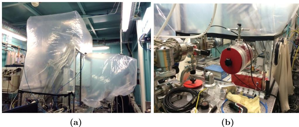
**Figure 2.16.:** He environment for the HR-XANES spectrometer at the INE-Beamline (a). Transfer lock for the He environment (b).
