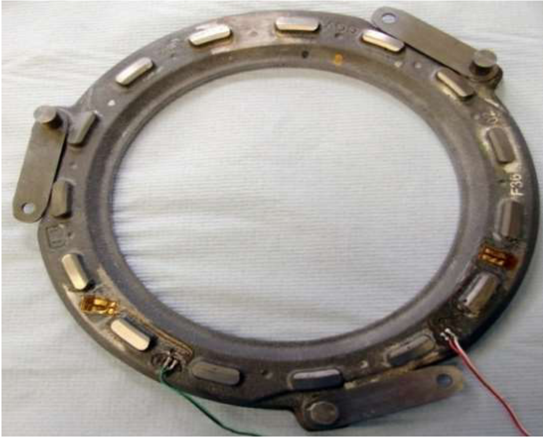
Figure 116: Sensor Positions on Pressure Plate
