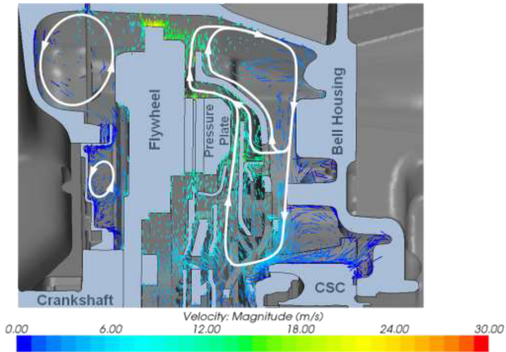
Figure 71: Flow Field Inside the Bell Housing
