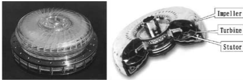
Figure 25: Modified Torque Converter 78
