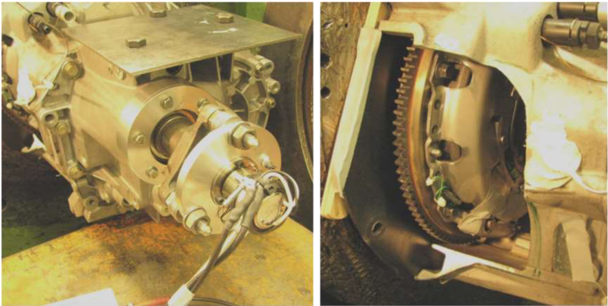
Figure 114: Rotary Transmitter (left) and Maintenance Hatch (right)
