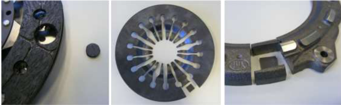
Figure 59: Sample Preparation: left: Lining; middle: Diaphragm Spring; right: Pressure Plate
