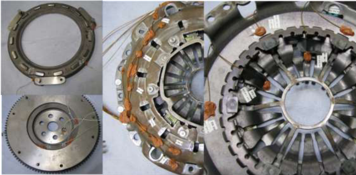
Figure 133: Temperature Measurement Positions Clutch System
