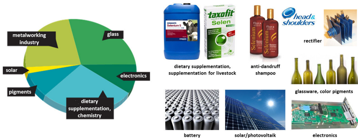
Figure 7: Industrially used Se divided into branches (left), examples of products containing Se (right) ( www.selenium.de – data from 2011) www.bembu.com , www.selenium.de (28.01.2014)).
