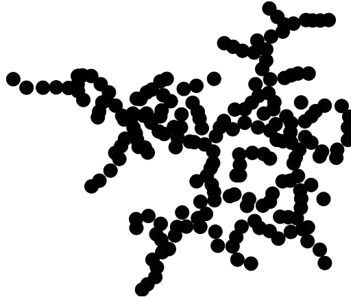
Figure 3.5: Schematic structure of a fractal floc formed by attractive spheres. If this structure spans the entire sample, the system is called a gel.
