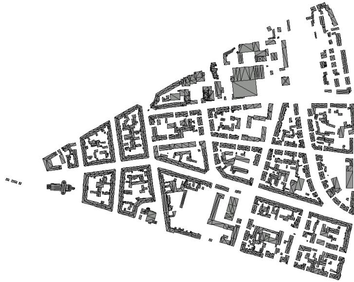
Figure 3.6: Extract of the considered ray tracing scenario, visualizing the considered building granularity and representing an inner city area in Karlsruhe, Germany. The data was provided and is copyrighted by the real estate office of the City of Karlsruhe.
