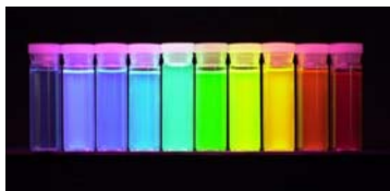
Fig. 1 Size-dependent photoluminescent properties of semiconductor cadmium Q dots [1]
