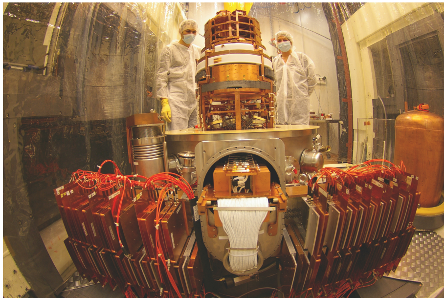
Figure 2.2. – Picture of the experimental setup with on the left and right the opened external PE and Pb shields and at the center, the cryostat and the 300 K electronics (bolometer boxes).
