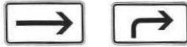
Figure 2.25.: Additional signs 1000-20 (pointing left: 1000-10) and 1000-21 (pointing left: 1000-11) which can be used to complement sign 365-65 [163]
