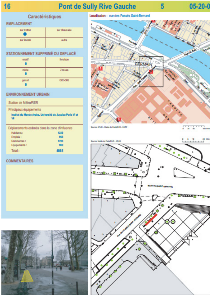
Figure 9.12.: Template used for the planning of bicycle sharing stations in Paris shown in [684]
