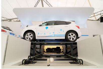
Figure 2.12.: Battery switching station from Better Place [94]
