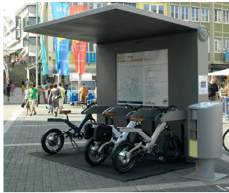
Figure 2.18.: Charging facilities for LEVs: battery switching [123]
