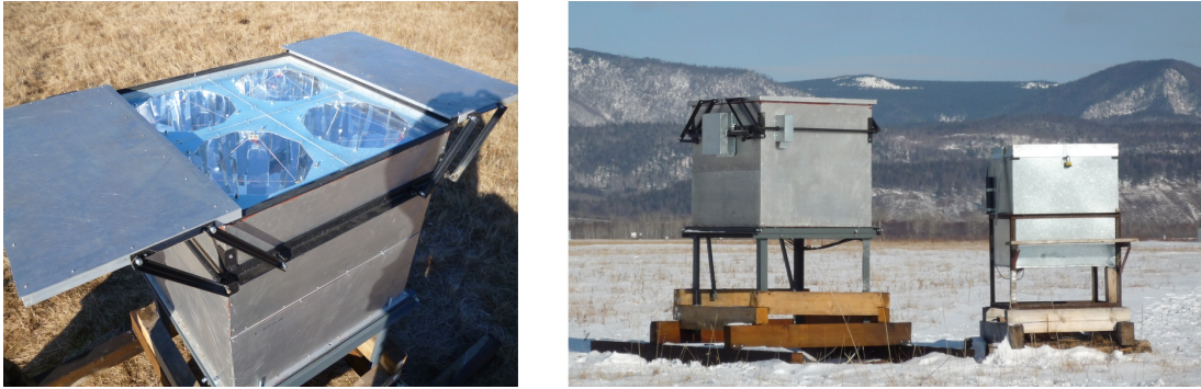
Figure 4.3.: HiSCORE station installed at the Tunka facility. Left: Single station with opened cover. Four Winston cones wrapping PMTs. Right: General view of the HiSCORE station (left) with electronic box (right).
