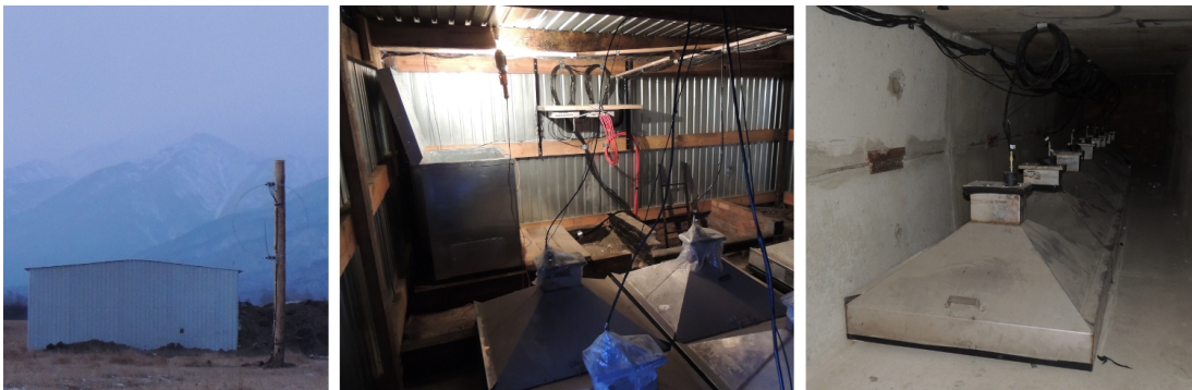
Figure 4.3.: HiSCORE station installed at the Tunka facility. Left: Single station with opened cover. Four Winston cones wrapping PMTs. Right: General view of the HiSCORE station (left) with electronic box (right).
