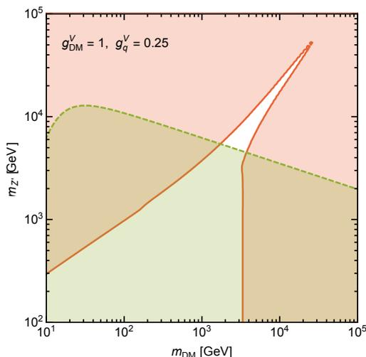
**Figure 2.** Vector(SM)–Vector(DM): parameter space excluded by the bound on the spin-independent DM-nucleon scattering cross section from LUX (green, dashed) and the parameter region where the DM annihilation cross section becomes so small that DM is overproduced in the early Universe (red, solid).
