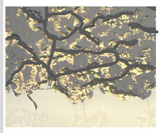
Cracks are barriers for oxygen vacancy diffusion
