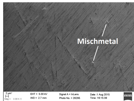
Figure 4.3.2.2-5: SEM micrograph of \text{V}_{40}\text{Fe}_8\text{Ti}_{26}\text{Cr}_{26} with addition of 6 mass% Mm in the as-cast state.
