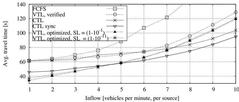
Figure 5.9: Average travel time vs. vehicle inflow. The IBD is 22 m, Tx. rate is 10 Hz, and vehicles speed is  $v = 50$  km/h. VTL includes three configurations: verified and performance optimized with two safety levels (0.9 and 0.9999999999). Confidence intervals are omitted for better visibility and are in the same order as in Figure 5.6
