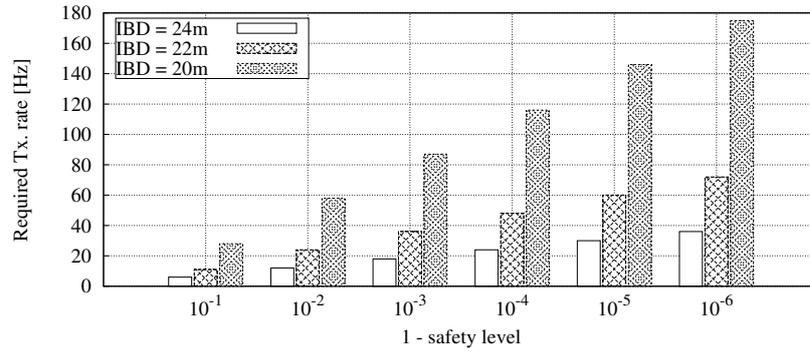
Figure 5.7: Required transmission rate vs. safety level at the safety distance  $D_{safe} = 49m$  for various IBDs, desired speed is  $v = 50$  km/h, and comfortable deceleration is  $a_{comf} = -2$  m/s<sup>2</sup>
