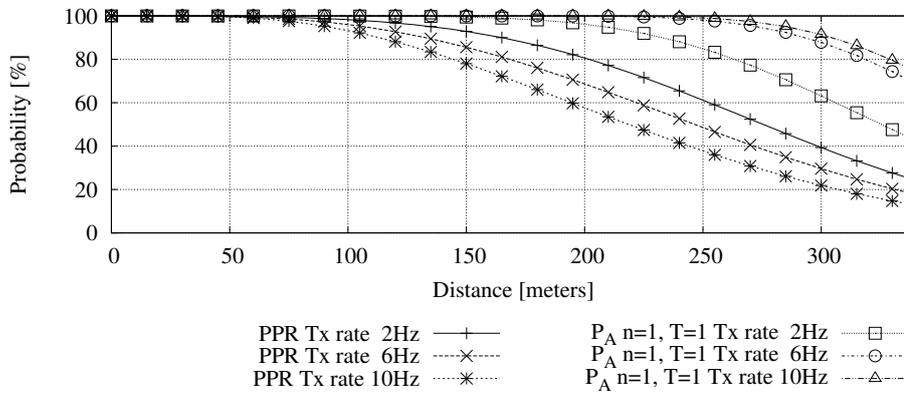
(b) The PPR for various transmission rates and the corresponding  $P_A$ . Vehicle density is 60 veh/km, transmission range is 300 m, transmission rates are 2, 6, and 10 Hz
