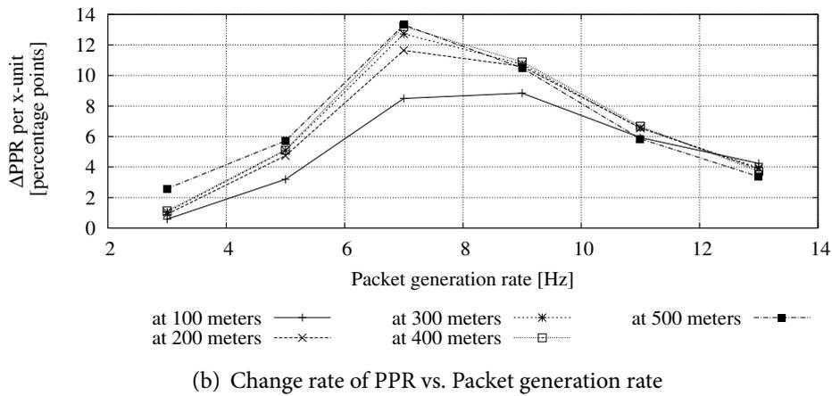
Figure 3.6: Sensitivity analysis with respect to the packet generation rate – Case 1. Packet size is 500 bytes, Tx. range is 1000 m, vehicle density is 100 veh/km, min. network load is 1.6 Mbps, max. network load is 11.2 Mbps
