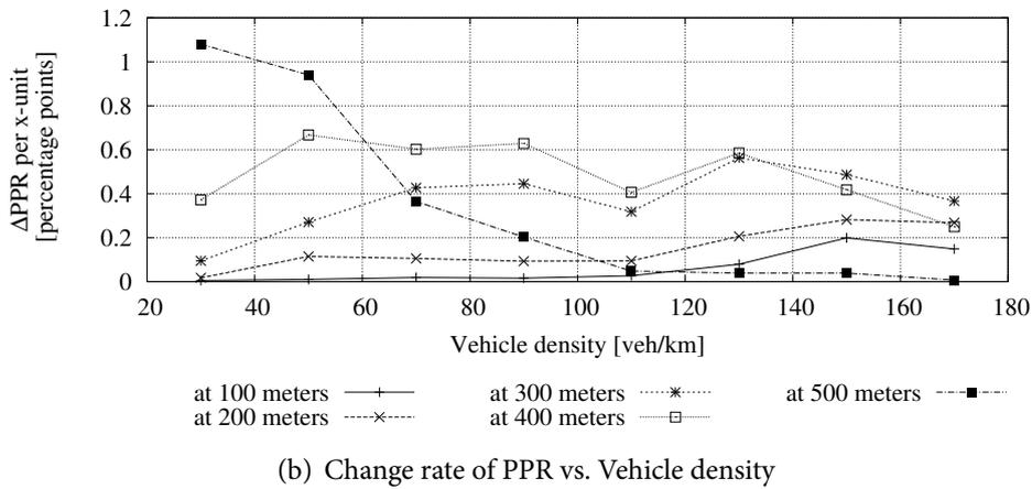
Figure 3.5: Sensitivity analysis with respect to vehicle density – Case 2. Packet size is 500 bytes, Tx. range is 500 m, PGR is 6 Hz, min. network load is 0.48 Mbps, max. network load is 4.32 Mbps
