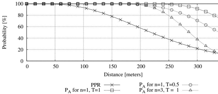
(a) The PPR and the corresponding  $P_A$  with various  $T$  and  $n$  parameters. Vehicle density is 60 veh/km, transmission rate is 10 Hz, transmission range is 300 m
