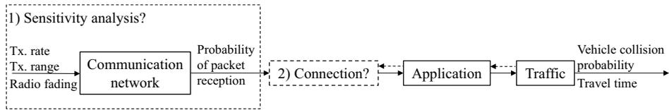
Figure 3.1: Open issues in performance evaluation of communication-based driver assistance applications: 1) The lack of sensitivity analysis that determines how factors such as radio fading, transmission range (Tx. range), and transmission rate (Tx. rate) impact the network performance, e.g., probability of packet reception. 2) The lack of bidirectional connection between network layer and application, or traffic layers
