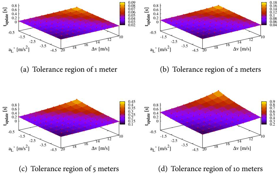
Figure 4.5: The impact of various tolerance regions on the time interval  $t_{update}$  for the “State change I-II”
