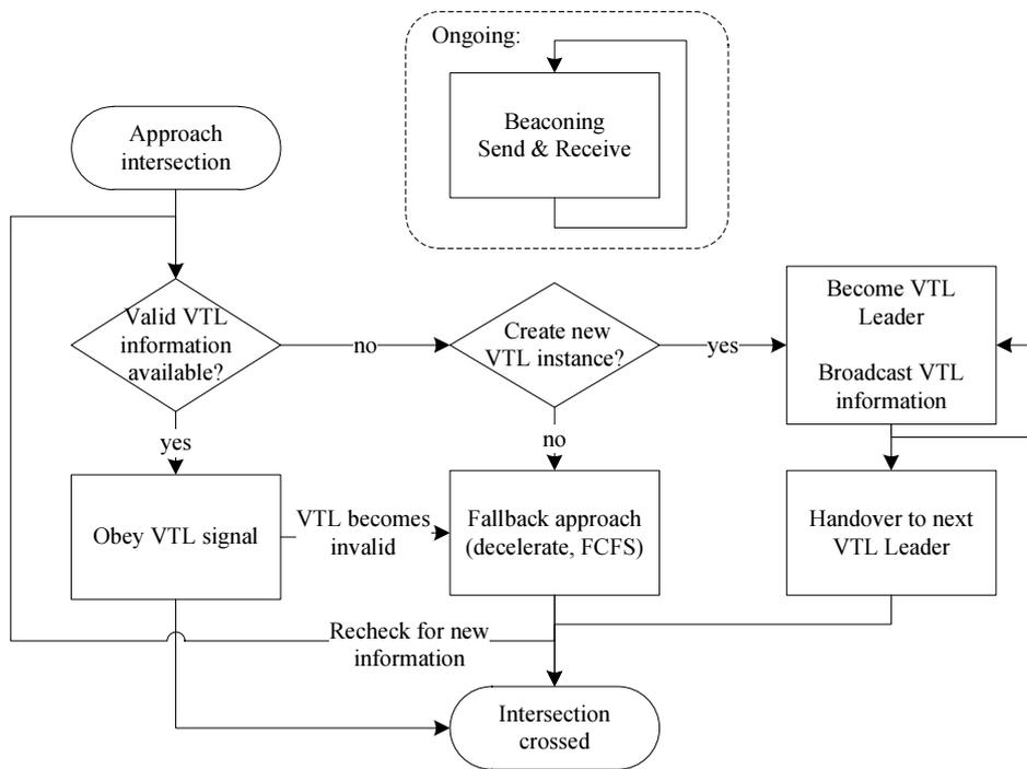
Figure 5.2: Flowchart of a fail-safe Virtual Traffic Lights application
