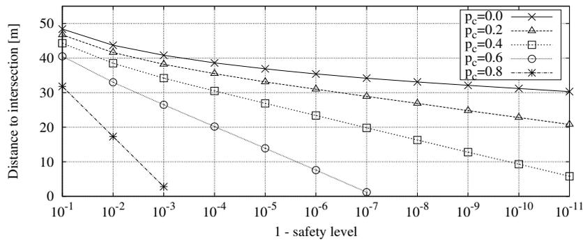
Figure 5.10: Distance to intersection at which a safety level value can be reached for various packet collision probabilities  $p_c$  for a fixed Tx. rate of 10 Hz and a constant speed 50 km/h
