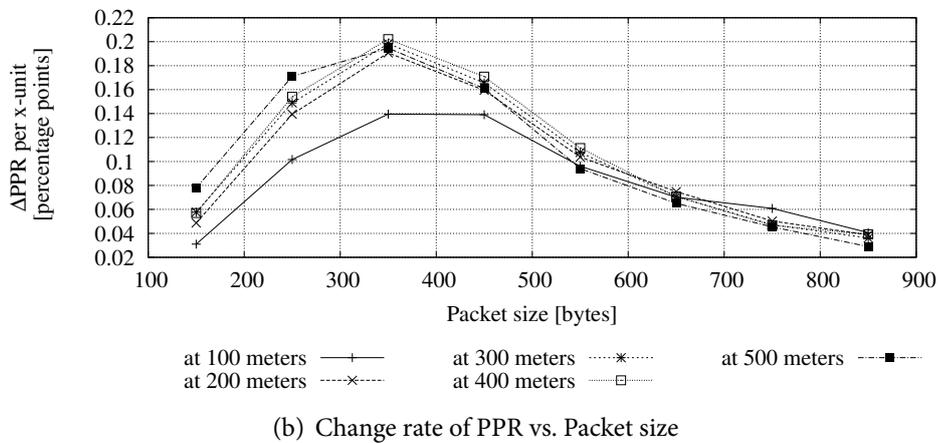
Figure 3.8: Sensitivity analysis with respect to the packet size – Case 1. Tx. range is 1000 m, vehicle density is 100 veh/km, PGR is 10 Hz, min. channel load is 0.96 Mbps, max. channel load is 8.64 Mbps
