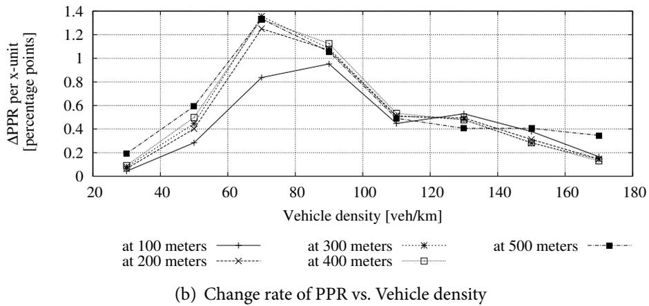
Figure 3.4: Sensitivity analysis with respect to vehicle density – Case 1. Packet size is 500 bytes, Tx. range is 1000 m, PGR is 10 Hz, min. network load is 1.6 Mbps, max. network load is 14.4 Mbps
