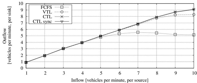
Figure 5.5: Throughput under various vehicle inflow. The IBD is 22 m, the Tx. rate is 10 Hz, and desired speed is  $v = 50$  km/h
