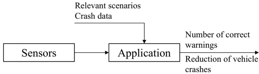
Figure 3.2: Typical process of performance evaluation for a sensor-based system
