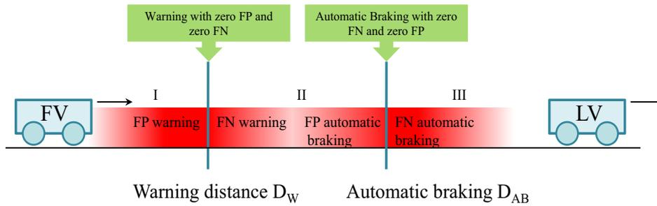
Figure 4.2: False Positive (FP) and False Negative (FN) errors
