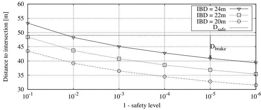
Figure 5.8: Distance to intersection at which a safety level value can be reached for a fixed Tx. rate of 10 Hz after braking at safety distance  $D_{safe}$ . The distance  $D_{brake}$  is the distance between safety distance  $D_{safe}$  and the point where a sufficient safety level is reached
