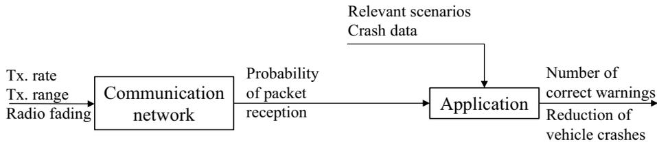
Figure 3.3: Typical process of performance evaluation for a communication-based system. Major focus is put on understanding communication network performance. The lack of bidirectional connection between network and application layers is depicted with an arrow from communication to application, but not vice versa
