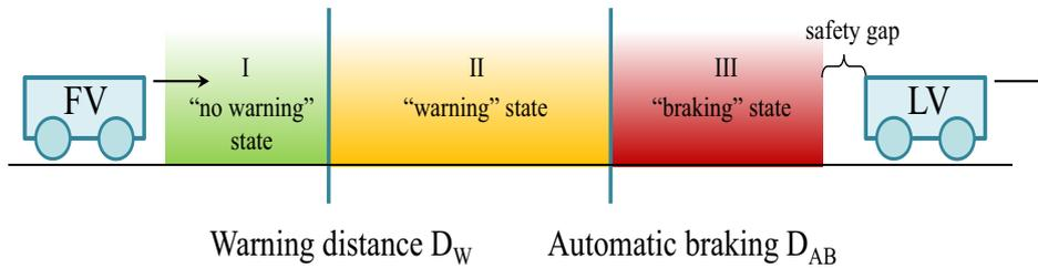
Figure 4.1: An example scenario for a Rear-End Collision Avoidance application. FV – following vehicle, LV – leading vehicle
