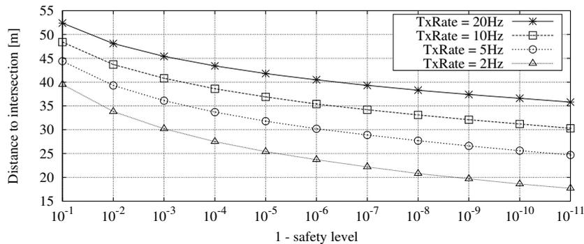
Figure 5.11: Distance to intersection at which a safety level value can be reached for various Tx. rates and a constant speed of 50 km/h and an IBD of 22 m
