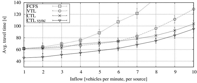
Figure 5.6: Average travel time vs. vehicle inflow with 95 % confidence interval. The IBD is 22 m, the Tx. rate is 10 Hz, and desired speed is  $v = 50$  km/h
