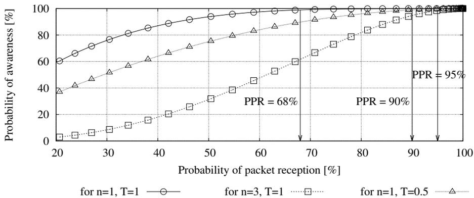
(c) Required PPR for various awareness parameters. Vehicle density is 60 veh/km, transmission rate is 4 Hz, transmission range is 300 m
