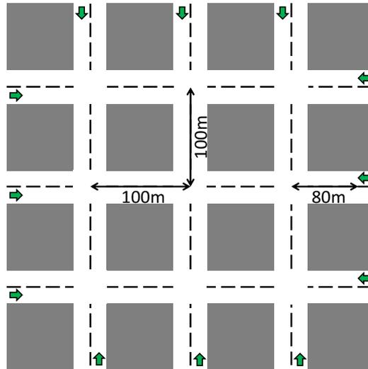
Figure 5.4: The 4x4 Manhattan grid scenario; green arrows represent vehicle sources
