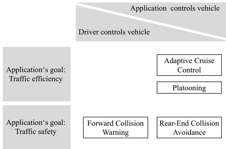
Figure 2.1: Overview of applications related to rear-end collisions
