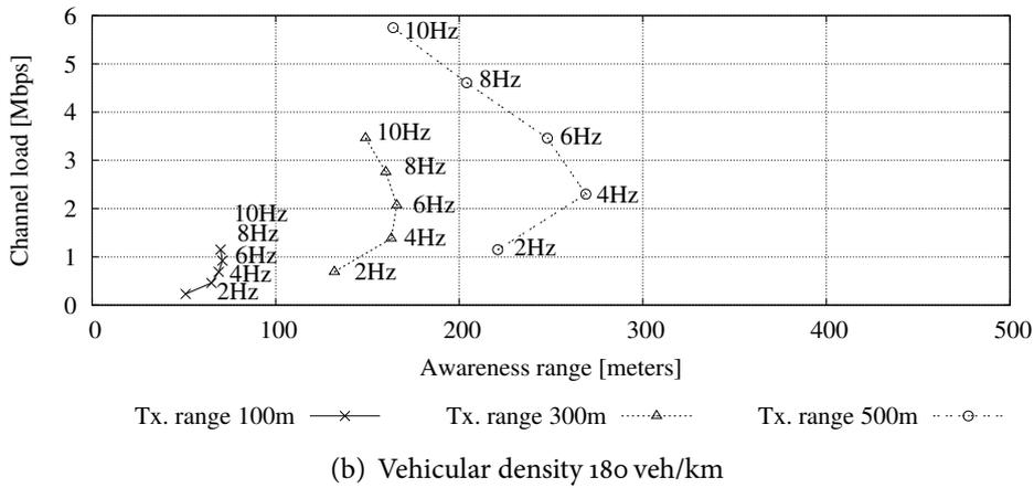
Figure 3.14: Maximum awareness range vs. channel load. Transmission rate is between 2 and 10 Hz, fading is following Nakagami- $m$  with  $m = 3$ ,  $P_A \geq 99\%$ ,  $T = 1$ , and  $n = 1$
