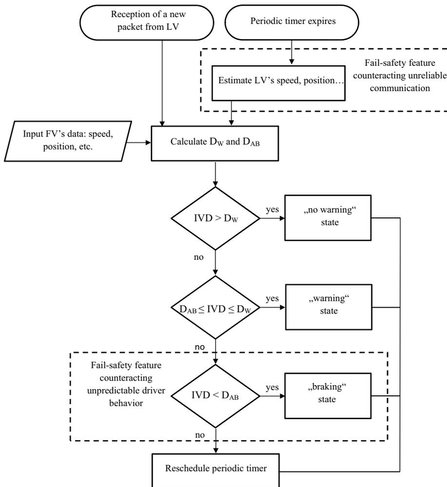
Figure 4.7: Flowchart of a fail-safe Rear-End Collision Avoidance application running on the FV. FV – following vehicle, LV – leading vehicle, IVD – inter-vehicle distance,  $D_W$  – warning distance,  $D_{AB}$  – automatic braking distance. The periodic timer refers to the internal sampling time of the application
