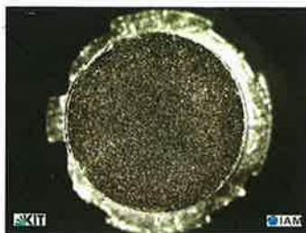
Top view on sintered stainless steel membrane (left), operation scheme of the new tool comprising embossing step (right)
