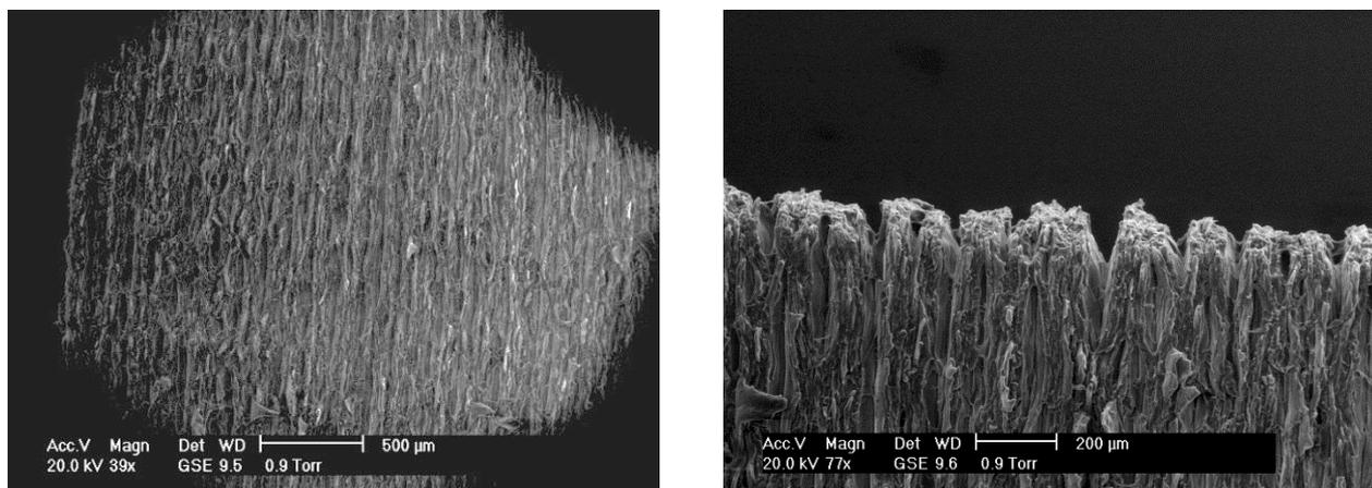
**Figure 2.** Structure of Polyjet-Modeling material Verowhite<sup>TM</sup> to visualize the thickness of the printed layers (pictures by ESEM).
