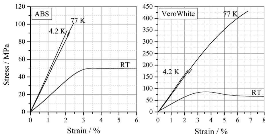
**Figure 7.** Compressive test results of ABS (left) and VeroWhite™ (right) at RT, 77 K and 4.2 K.
