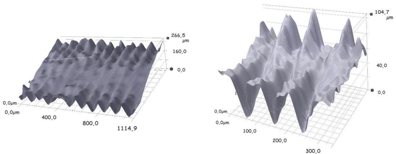
**Figure 1.** Structure of ABS to investigate the printed layer thickness using the surface profile obtained by optical microscope (left 300x and right 1000x magnification).
