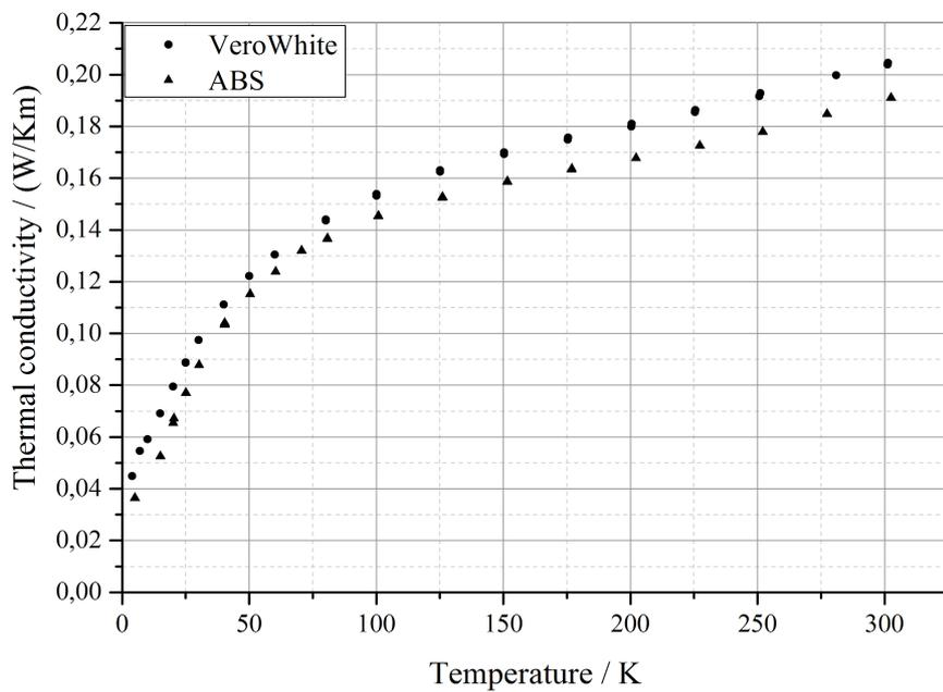
**Figure 5.** Thermal conductivity between 300K and 4.2 K of ABS and VeroWhite™.
