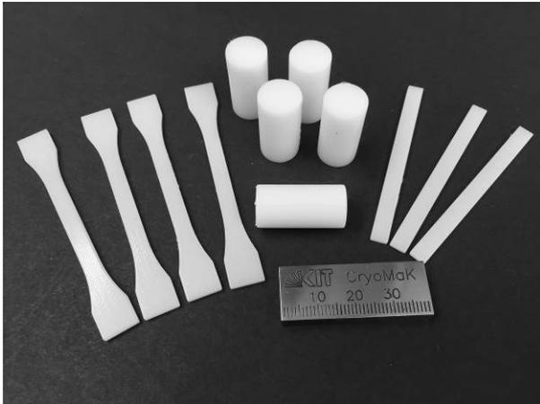
**Figure 3.** Specimen geometries manufactured by 3D printing method. Shown specimen for tensile (left), compression (middle), and thermal expansion (right) measurement.
