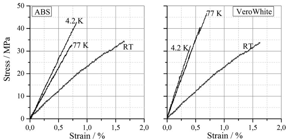
**Figure 6.** Tensile test results of ABS (left) and VeroWhite™ (right) at RT, 77 K and 4.2 K.
