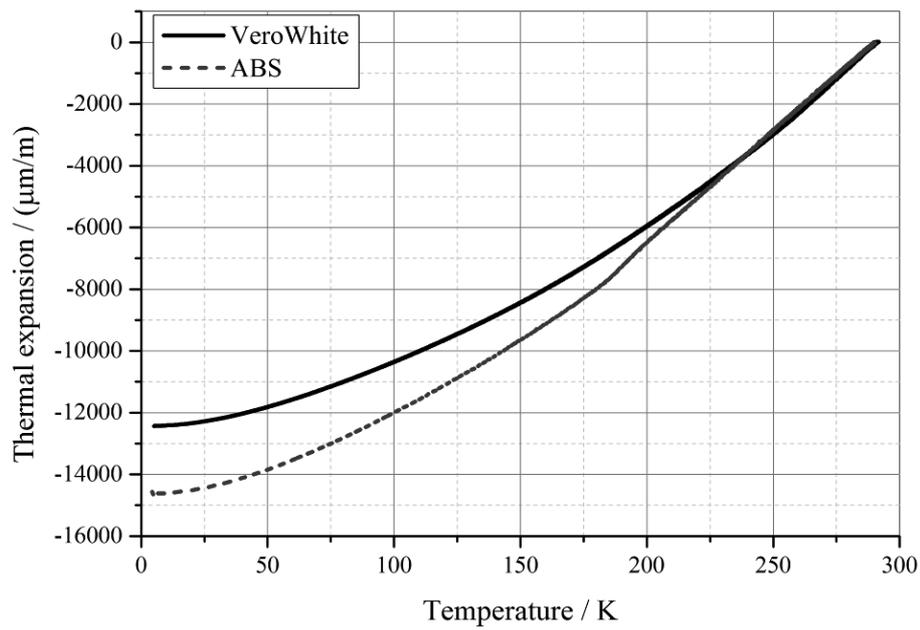
**Figure 4.** Thermal contraction between 290 K and 4.2 K of ABS and VeroWhite™.
