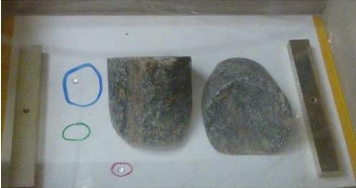
Figure 21. Äspö diorite core #2.2 fragments and the Tc reference drops ( 10 \mu\text{L } 10^{-5} \text{ M} in the blue circle and 10 \mu\text{L } 10^{-7} \text{ M} Tc in the red circle) on the autoradiography screen.
