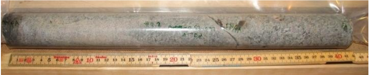
Figure 17. Drill core #2.2 (0.53-0.97 m, borehole KA2370A-01) with a natural fracture.
