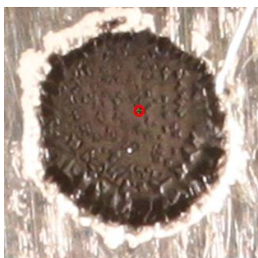
Figure 39. Magnetite sample for XPS (left) after contacting with Tc(VII)-containing solution. Red circle indicates the region where the XPS narrow scan (right) of Tc 3d spectrum was measured.
