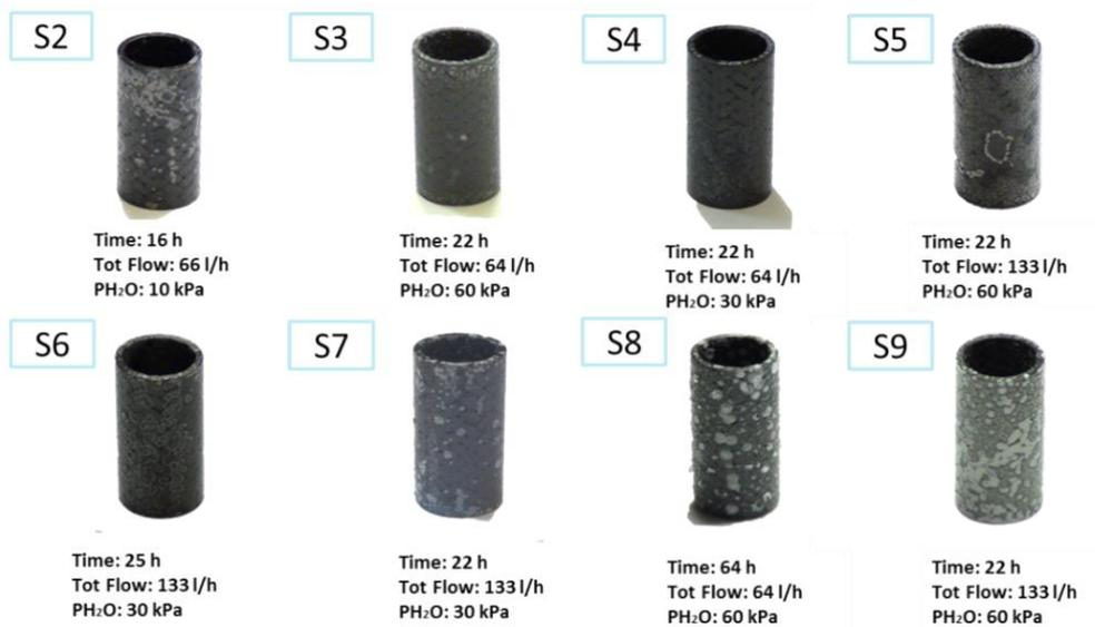
**Figure 2.16:** Post-test appearance of samples oxidized at 1600 °C at different steam partial pressures.
