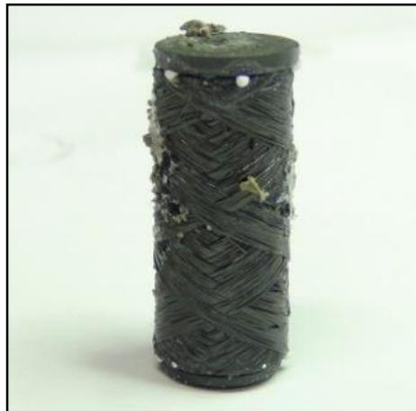
**Figure 6.14:** Triplex double layer sample T10C after quench.
