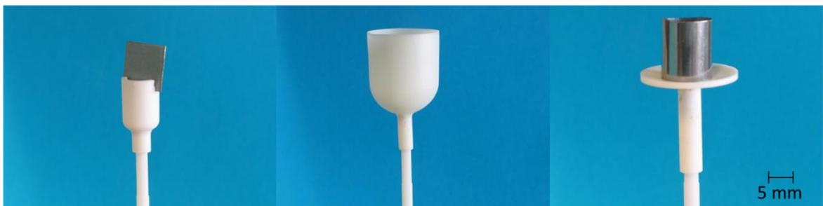
**Figure 4.3:** Overview of the different samples and sample holders: left) holder for the plates, center) holder used in the case powder was produced; right) holder for tubes.
