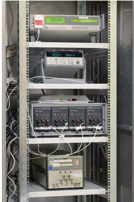
Figure 4.12: High precision measurement and calibration cabinet, described from top to bottom. High-precision digital voltmeter with 8\frac{1}{2} digits resolution. Matrix multiplexer connecting the high precision voltage dividers, voltmeters and reference sources to enable the automated calibration. Four reference sources that generate highly stable 10 V. Reference divider for calibrating the KATRIN dividers. The final arrangement contains two additional voltmeters, that can be integrated easily by plug and play.
