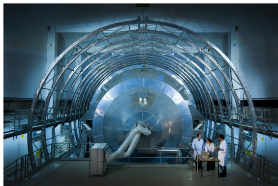
Figure 3.4: Photography from the upstream to the downstream side of the spectrometer without e-gun. The rings surrounding the vessel serve as holding structure for the air-coil system. Photo: Karlsruhe Institute of Technology (KIT), 2009.
