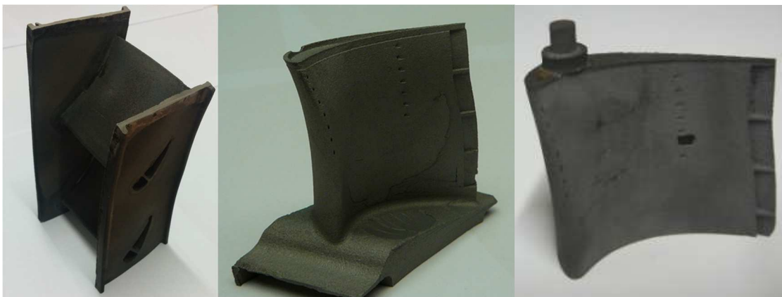
Fig. 3-6: double vane segment (left) and turbine blade geometries (middle and right) produced by HIPing of a gas-atomized Nb-20Si-23Ti-6Al-3Cr-4Hf powder, HIP can was produced by SLM, courtesy of The University of Birmingham, Interdisciplinary Research Centre in Materials Processing, Birmingham, UK
