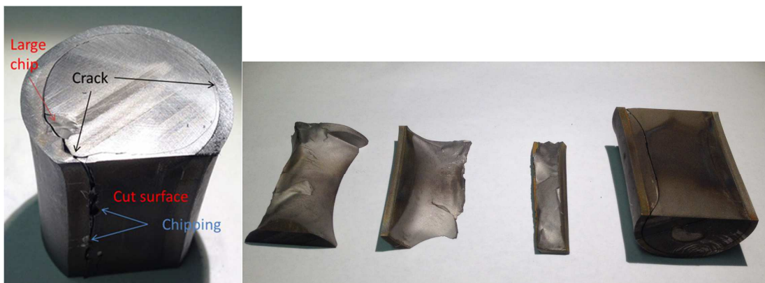
Fig. 6-1: photographs of cracked HIP MA material after EDM trials; partially still encased by the iron HIP can; can diameter 30 mm
