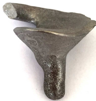
Fig. 3-1: trial to drop cast Nb-20Si-23Ti-6Al-3Cr-4Hf into a cylindrical copper mould by arc-melting; only few drops reached the bottom of the mold; using the same technique, drop casting of molybdenum silicides with an even higher melting point was possible
