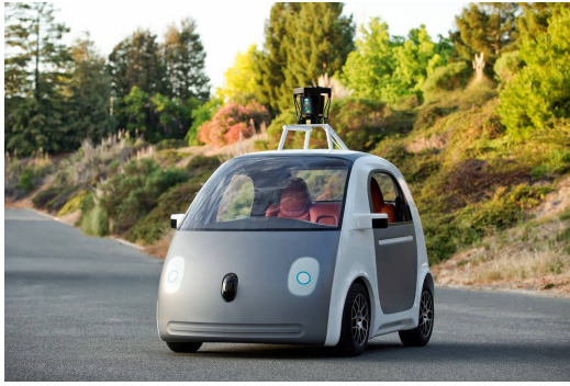
(a) Self-driving car with LIDAR [Google]. 2,1
