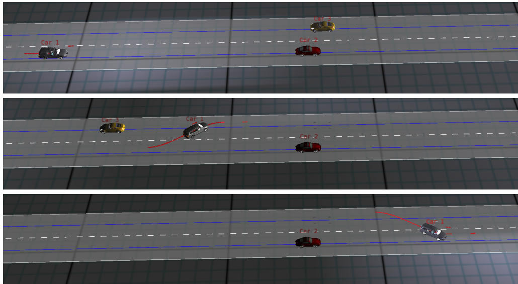
Figure 7.9: MDP highway driving: overtaking with oncoming traffic. The ego vehicle is grey. The trajectories visualizing its decisions are indicated in red [Brechtel et al., 2011]. ©2011 IEEE
