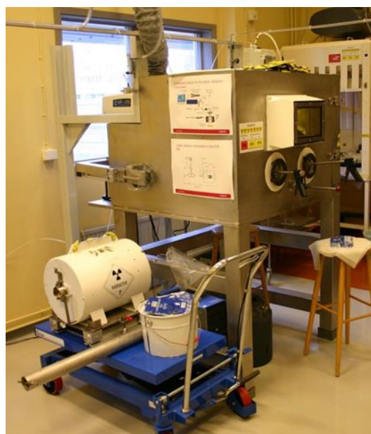
Figure 12.1: The laser ablation hot cell and the sample transfer cask.
