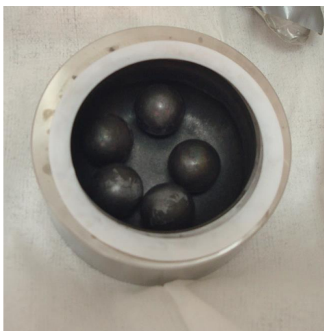
Figure 22.1: Tungsten carbide milling bowl and balls.
