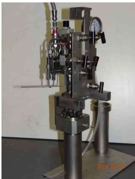
Figure 9.2: Manufactured autoclave undertaking 50 bar pressure test.
