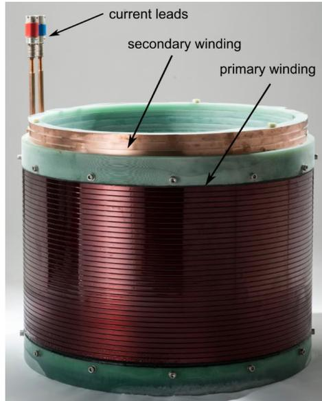
Figure 4.20: Built AC-SFCL demonstrator with secondary winding pulled out
