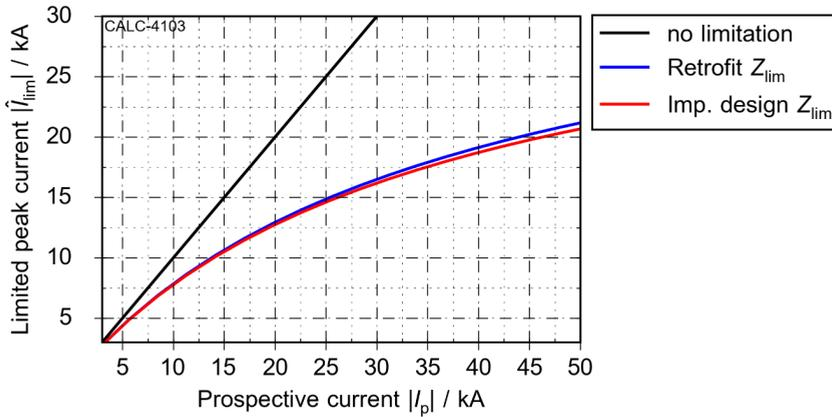
Figure 6.19: Expected fault current limitation of the retrofit and the low impedance design for 380 kV, 1 kA,  $z = 6\%$
