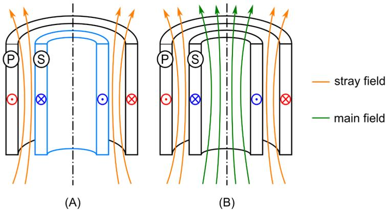
Figure 3.7: Magnetic field of the primary (P) and secondary (S) winding for (A) normal operation of the AC-SFCL (secondary winding in superconducting state) and (B) both windings are in normal conducting state.
