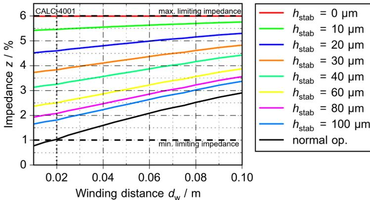
Figure 6.1: Calculated impedance of the retrofit for normal operation and fault condition for constant current  $I_{max} = 300$  A
