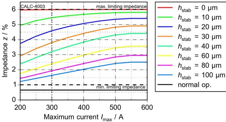
Figure 6.6: Dependency of impedance on critical current and stabilization for the low impedance design ( $d_w = 2$  cm)
