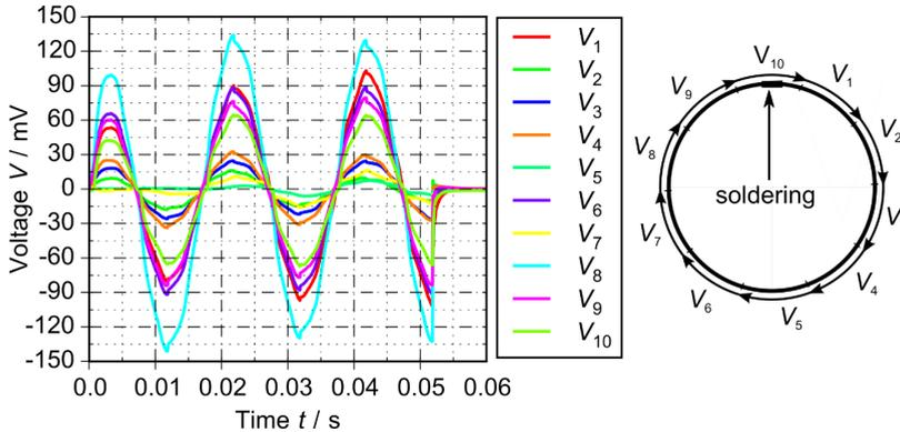
Figure 4.16: Quench results of a single short-circuited *REBCO* ring (tape B) with ten voltage taps (order is shown on the right)
