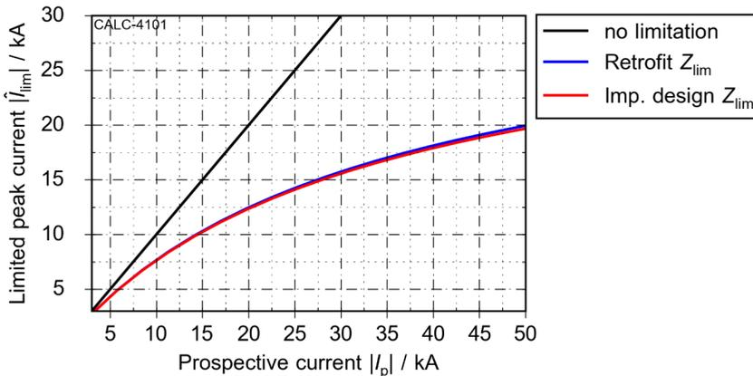
Figure 6.7: Expected fault current limitation of the retrofit and the low impedance design for 10 kV, 1 kA, z = 6%
