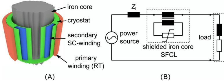
Figure 2.12: (A) Schematic of the shielded iron core SFCL and (B) equivalent circuit diagram
