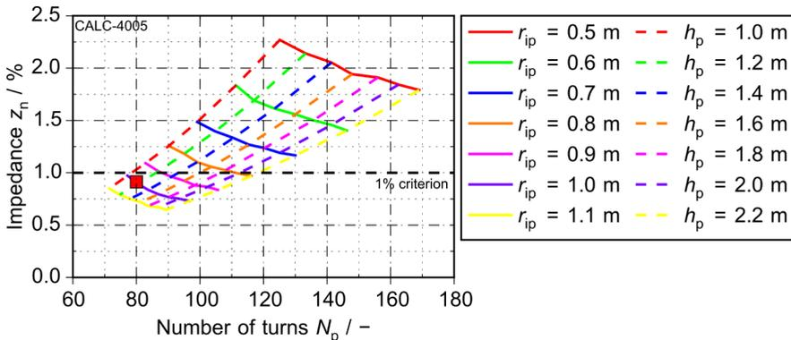
Figure 6.10: Results for impedance during normal operation of 110 kV, 1 kA,  $z = 6\%$  AC-SFCLs for variation of the geometry of the primary winding. The red square indicates the chosen low impedance design
