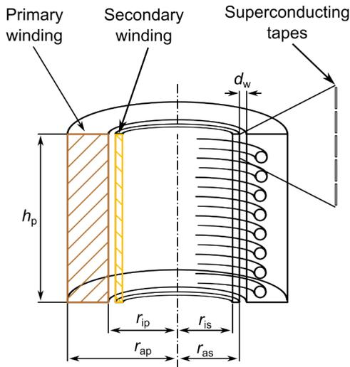
Figure 3.1: Schematic cross-sectional view of the AC-SFCL
