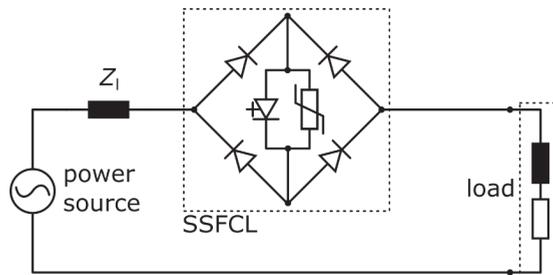
Figure 2.7: Topology of an SSFCL based on a GTO and diode bridge rectifier circuit. The GTO is placed in the DC branch parallel to a varistor [MSD04]
