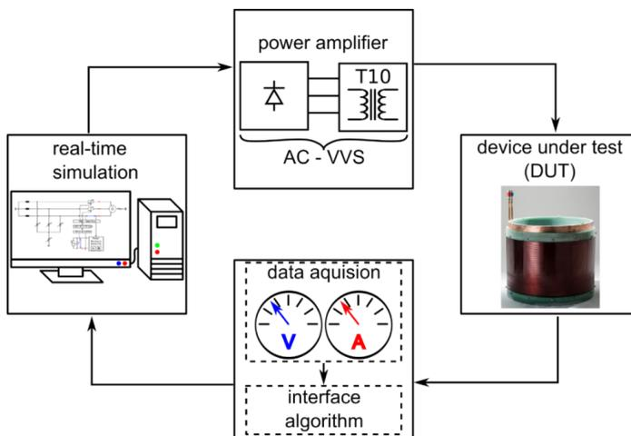
Figure 5.1: Principle of the power hardware in-the-loop setup
