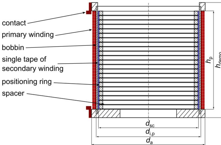
Figure 4.19: Schematic cross-sectional view of the build AC-SFCL demonstrator. The corresponding dimensions are shown in Table 4.8
