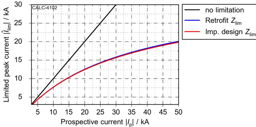
Figure 6.13: Expected fault current limitation of the retrofit and the low impedance design for 110 kV, 1 kA,  $z = 6\%$
