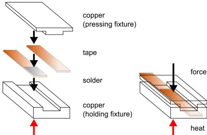
Figure 4.12: Principle of fixture for soldering tapes. The tapes are placed in the holding fixture with the pressing fixture on top. A constant force and heat is applied until the REBCO tapes form the soldered connection.
