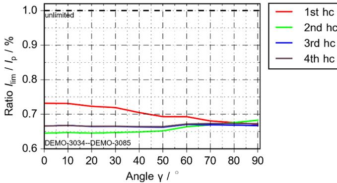
Figure 4.37: Measured fault current limitation for a fault angles  $\gamma$  between  $0^\circ$  and  $90^\circ$  for all four half cycles
