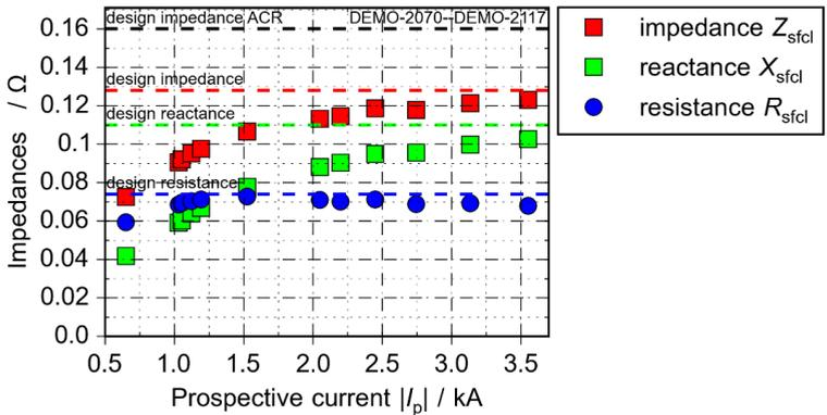
Figure 4.34: Calculated development of resistance, reactance and impedance depending on prospective current
