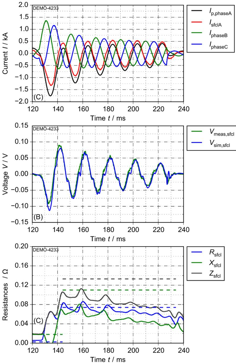
Figure 5.18: Results for fault current limitation of a 3-phase fault with ground connection for (A) currents, (B) voltages and (C) resistances ( $S_{base} = 120$  kVA,  $R_{fit} = 40$  m $\Omega$ ,  $p_f = 1.0$ )
