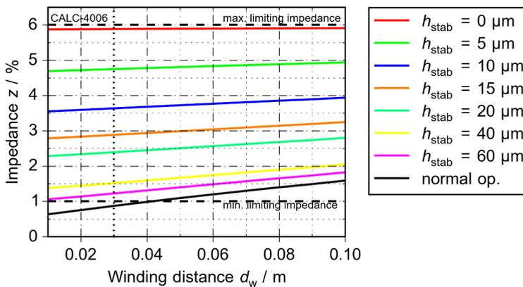
Figure 6.11: Dependency of the calculated impedance on winding distance and stabilization for the low impedance design ( $I_{max} = 300$  A)
