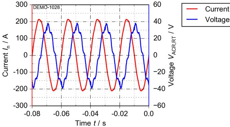
Figure 4.26: Measured current and voltage drop across the primary winding at room temperature during normal operation
