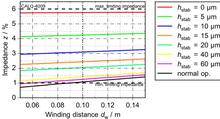
Figure 6.17: Dependency of the calculated impedance on winding distance and stabilization for the low impedance design ( $I_{\text{max}} = 300 \text{ A}$ )
