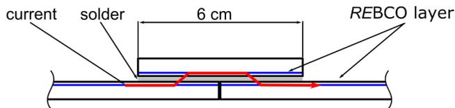
Figure 4.11: Principle of the soldered connection. The ends of a *REBCO* tape face each other and a second, short *REBCO* piece is used to make the connection.
