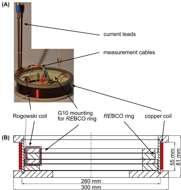
Figure 4.14: (A) Picture of the manufactured test coil and (B) cross-sectional view
