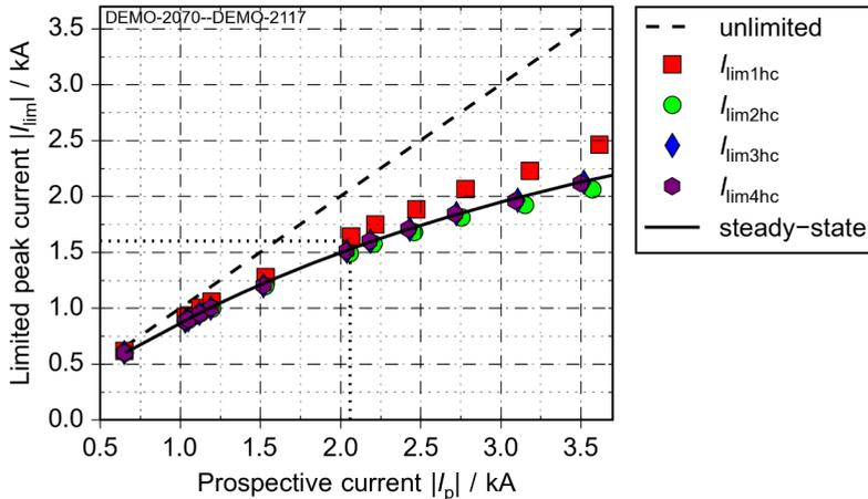
Figure 4.30: Summary of the measured fault current limitation for faults with a duration of four half cycles and the calculated result for steady-state. The case of Figure 4.29 is indicated.
