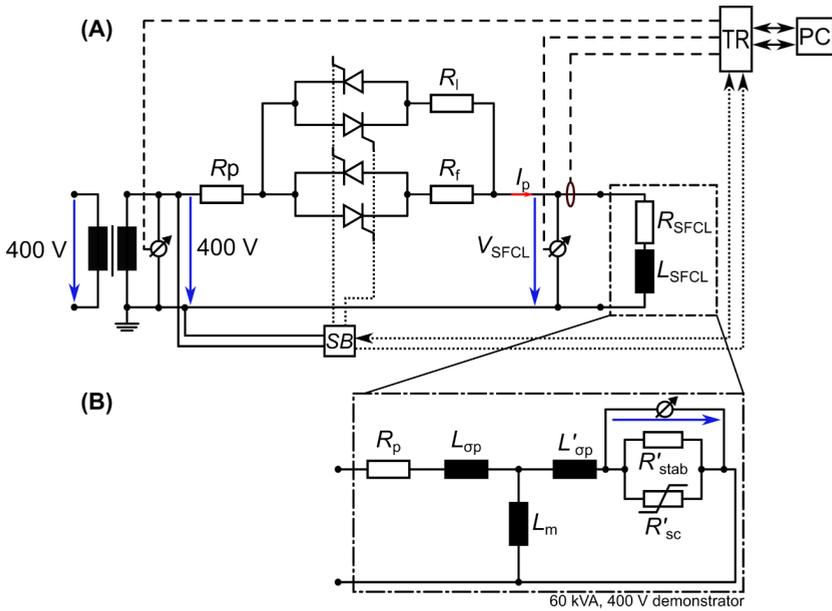
Figure 4.25: (A) Equivalent circuit diagram of the measurement setup used to investigate the AC-SFCLs behavior in all three operational modes and (B) equivalent circuit diagram of the AC-SFCL demonstrator
