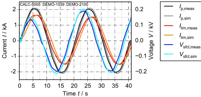
Figure 5.2: Comparison of the simulated model and measured results at KIT for fault current limitation for a fault current with  $I_p = 2$  kA and a duration of four half-cycles
