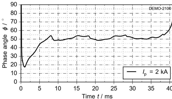
Figure 4.32: Calculated phase angle between current and voltage for the fault of four cycles shown in Figure 4.29
