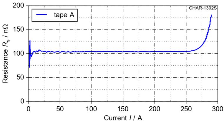
Figure 4.13: Measured resistance depending on current for small soldered pieces of REBCO tapes (6 cm lap length, 12 cm total length)
