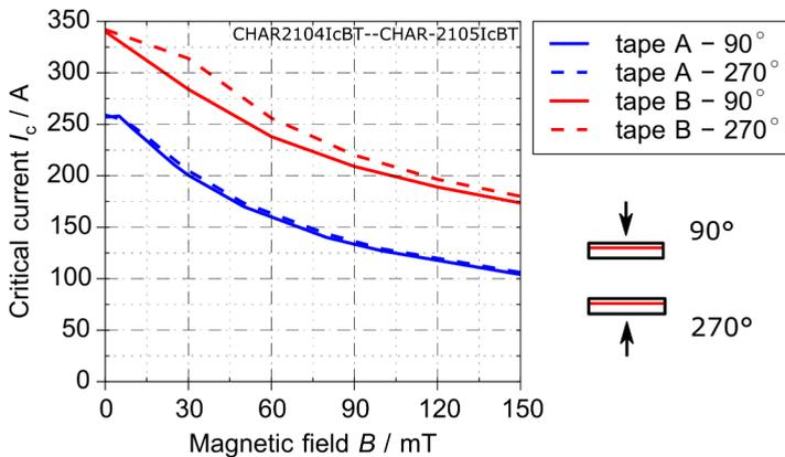
Figure 4.5: Measured critical current  $I_c$  depending on magnetic field density for perpendicular field
