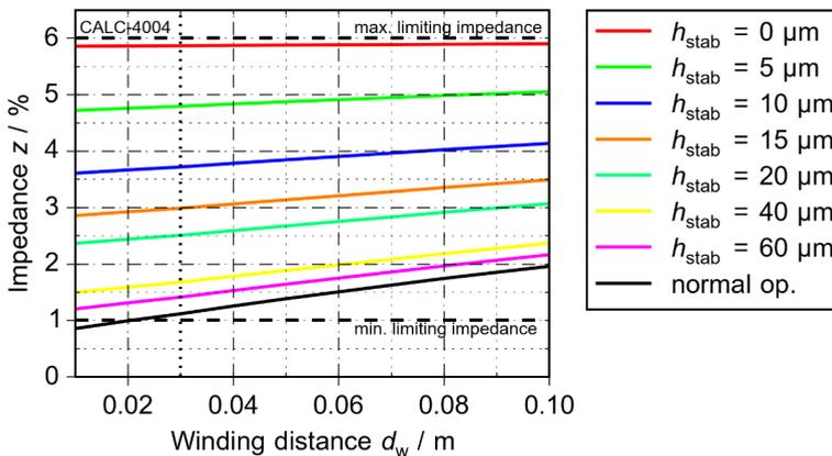
Figure 6.8: Calculated impedance of the retrofit for normal operation and fault condition for constant current  $I_{max} = 300$  A
