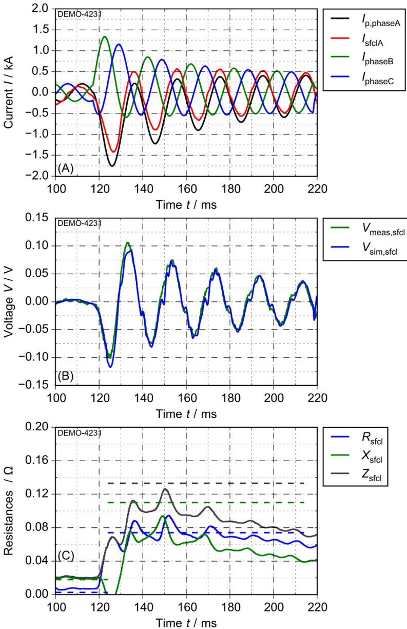
Figure 5.20: Results for fault current limitation of a 3-phase fault without ground connection for (A) currents, (B) voltages and (C) resistances ( $S_{base} = 120$  kVA,  $R_{fit} = 40$  m $\Omega$ ,  $p_f = 1.0$ )
