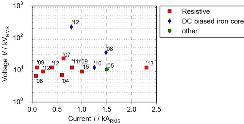
Figure 2.13: Rated voltage and current of selected field tested SFCLs (compare Table 2.2)
