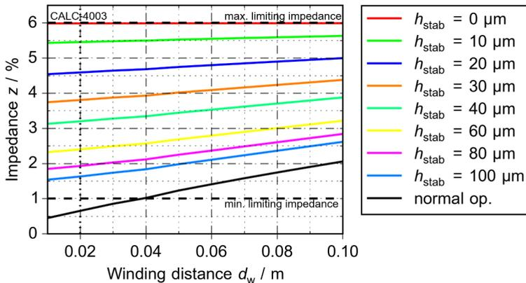
Figure 6.5: Dependency of impedance on winding distance and stabilization for the low impedance design ( $I_{max} = 300$  A)
