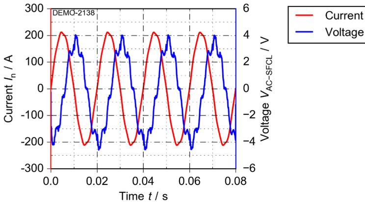
Figure 4.28: Measured current and voltage drop across the AC-SFCL demonstrator during normal operation
