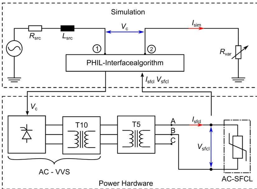
Figure 5.4: PHIL setup for verification of results and testing of different interface methods. The AC – VVS is described in [SES10].
