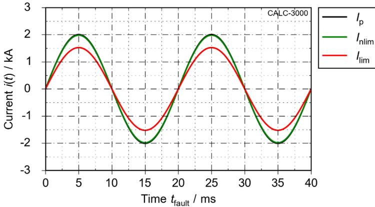
Figure 4.23: Simulation of an expected fault current limitation of the AC-SFCL demonstrator. A prospective short-circuit current of  $I_p = 2$  kA is limited to  $I_{lim} = 1.5$  kA
