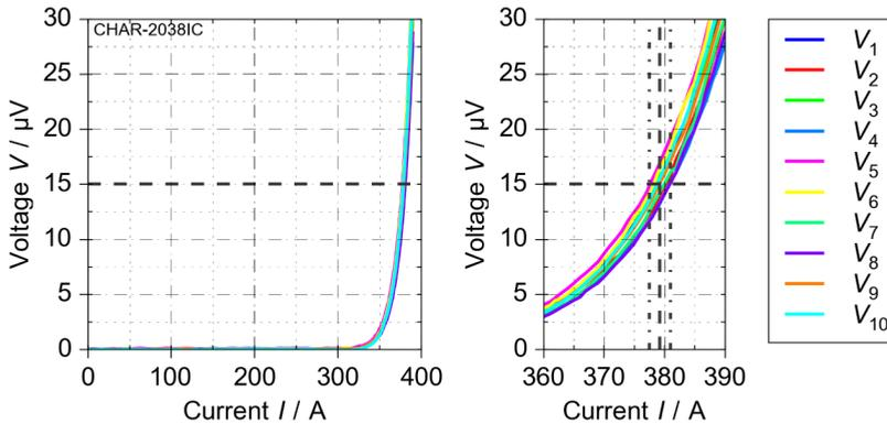
Figure 4.10: Measurement of critical current  $I_c$  for a sample of tape B at self-field
