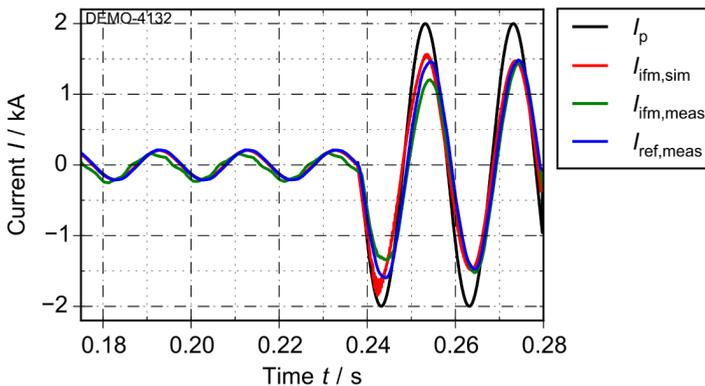
Figure 5.10: Comparison of results of the impedance feedback method (IFM) for simulation and measurement with the reference measurement during load and fault cycles
