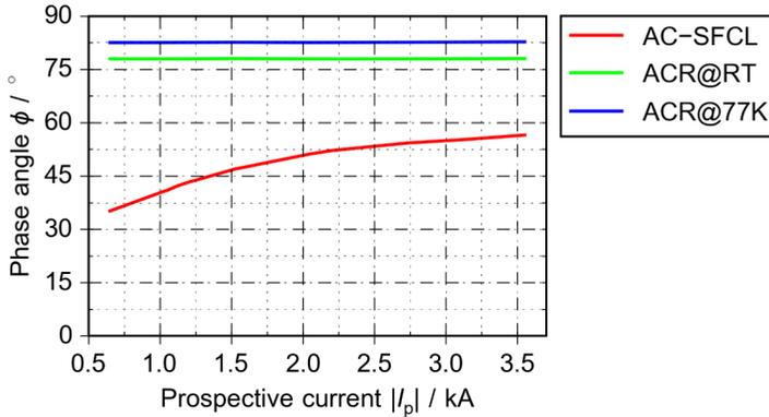
Figure 4.33: Calculated average phase angle of the AC-SFCL and the air core reactor for a fault of four cycles depending on prospective current
