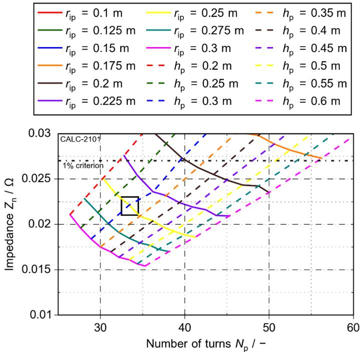
Figure 4.18: Results for impedance during normal operation of the demonstrator in the first design step magnified on geometries fulfill the  $z \leq 1\%$  criterion (fill-factor  $f_{ip} = 0.85$ ). The rectangle indicates the chosen geometry
