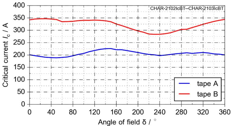
Figure 4.6: Measured critical current  $I_c$  depending on the angle of the magnetic field for tape A and tape B for a magnetic field density of  $B = 30$  mT
