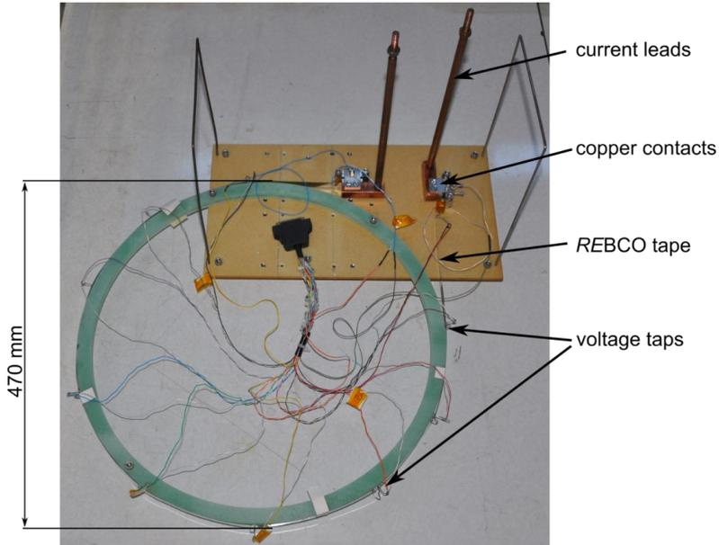
Figure 4.8: Mechanical setup for measuring the critical current at self-field and 77 K. The REBCO tape is bent with the same diameter as in the AC-SFCL.
