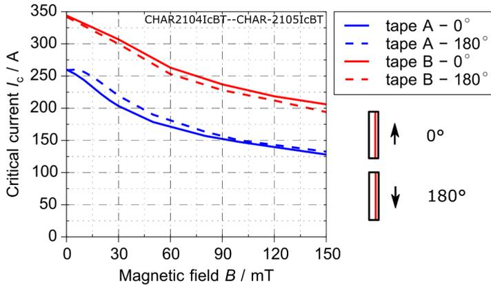
Figure 4.4: Measured critical current  $I_c$  depending on magnetic field density for parallel field
