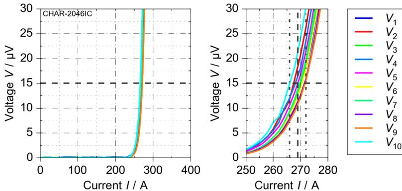
Figure 4.9: Measurement of critical current  $I_c$  for a sample of tape A at self-field
