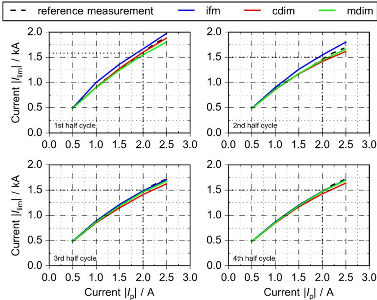
Figure 5.13: Comparison of current limitation of the three interface algorithms - simulation
