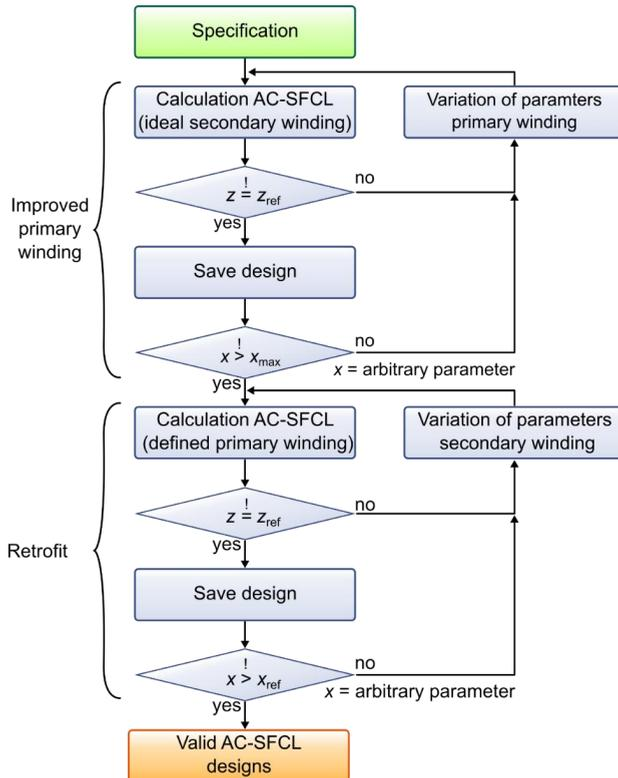
Figure 3.8: General approach of the proposed design method. The design process is separated into two major parts, the calculation of a design with an improved primary winding and the insert. This allows independent the calculation of the retrofit of an air core reactor and the design of an AC-SFCL with improved primary winding.
