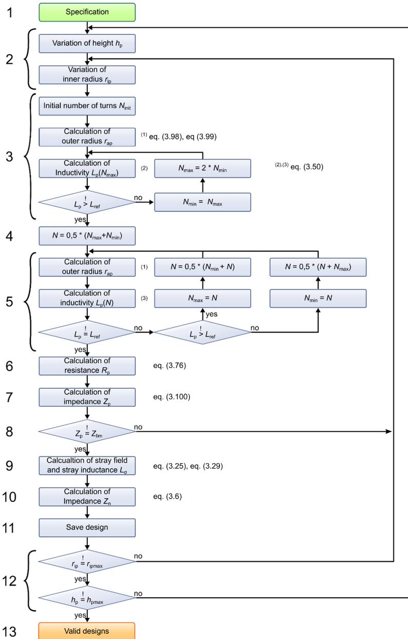
Figure 3.11: Flow diagram for optimized design. With a set of geometrical parameters the number of turns  $N$  are calculated to match the reference impedance  $L_{ref}$  and the impedance  $Z_{lim}$  assuming constant parameters for secondary winding.
