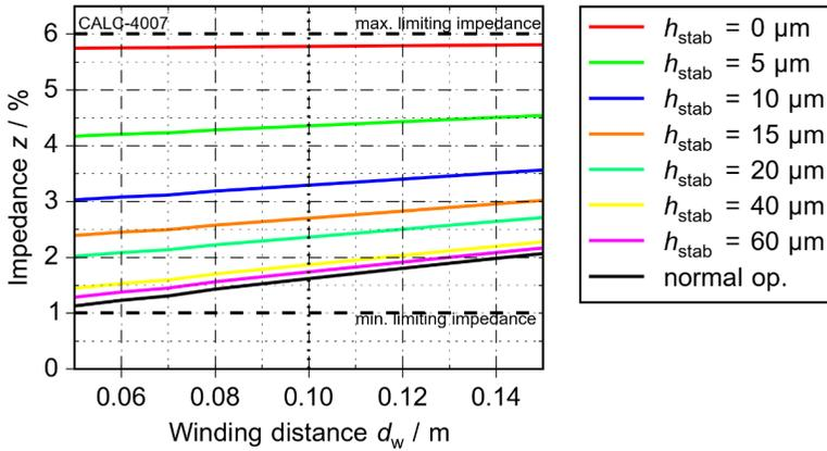
Figure 6.14: Calculated impedance of the retrofit for normal operation and fault condition for constant current  $I_{\max} = 300$  A
