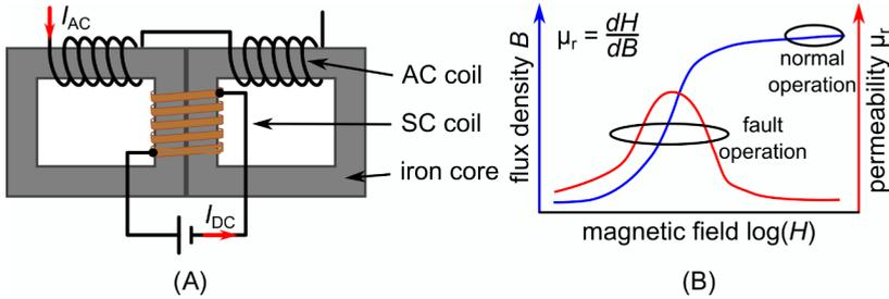
Figure 2.11: (A) Schematic of the saturated iron core SFCL for single phase and (B) qualitative magnetization curve with regions of operation according to [MD09]
