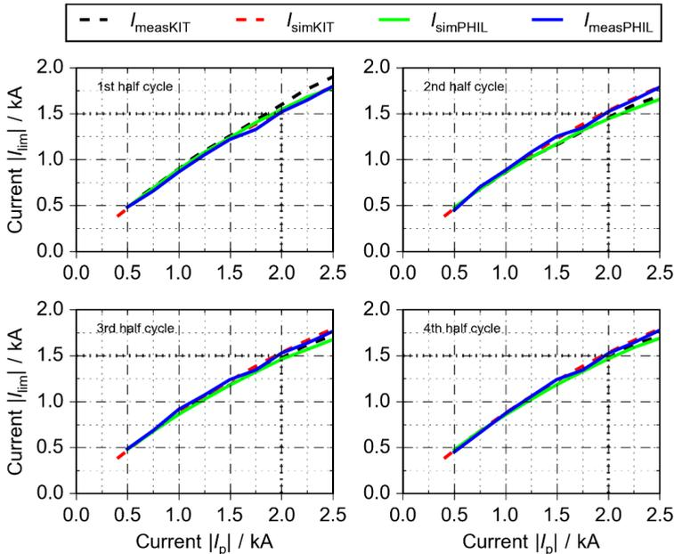
Figure 5.7: Comparison of PHIL results with KIT results for fault current limitation during four half cycles for increasing prospective currents. The example shown in Figure 5.5 is indicated.
