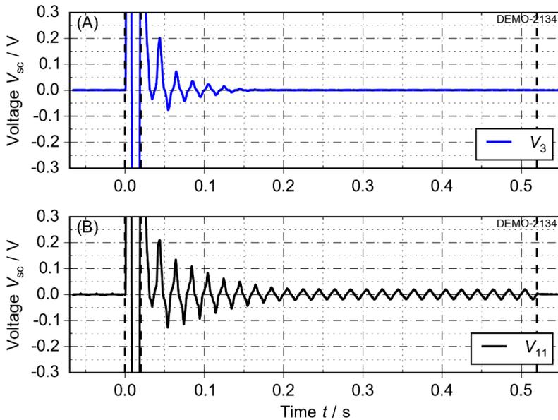
Figure 4.41: Voltages of two REBCO tapes during fault and following load cycle. (A) shows the recovery of tape 3, which recovers 124 ms after the fault is switched off, while in case (B) the tape is not recovering
