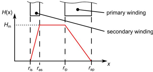
Figure 3.4: Magnetic field distribution in radial direction of the AC-SFCL, which is similar to the distribution of the magnetic field in transformers [Lei06]
