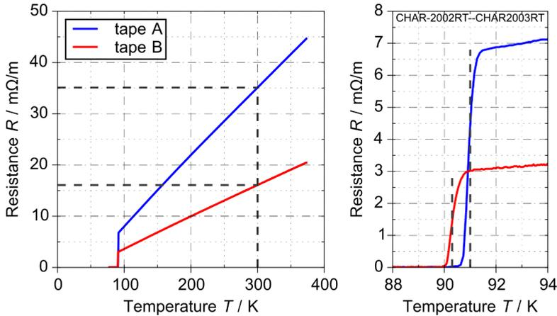
Figure 4.2: Measured resistance depending on temperature  $R(T)$  of the superconducting tape A and tape B in the measured range
