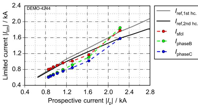
Figure 5.24: Summary of fault current limitation for symmetrical three phase fault ( $S_{base} = 180$  kVA)
