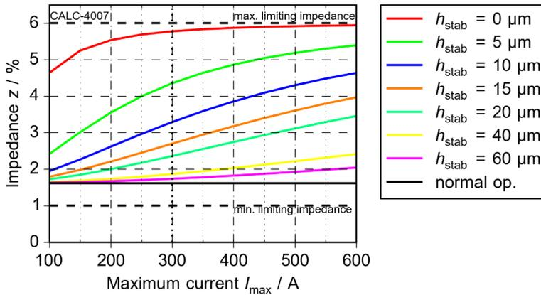
Figure 6.15: Calculated impedance of the retrofit for normal operation and fault condition for constant winding distance  $d_w = 10$  cm
