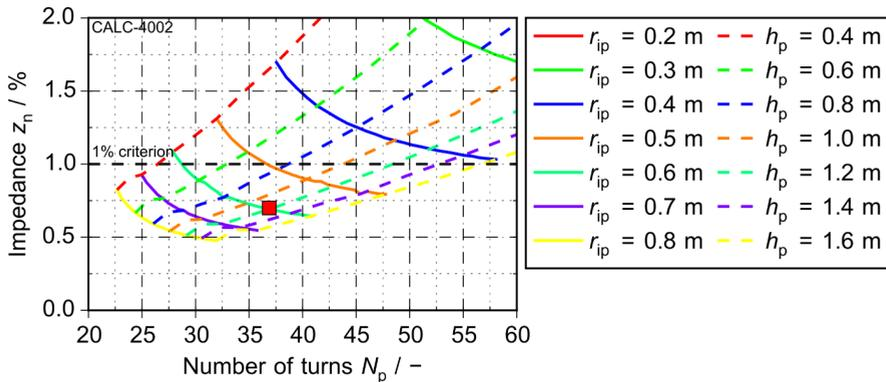
Figure 6.4: Magnified view of Figure 6.3. The red square indicates the chosen low impedance design
