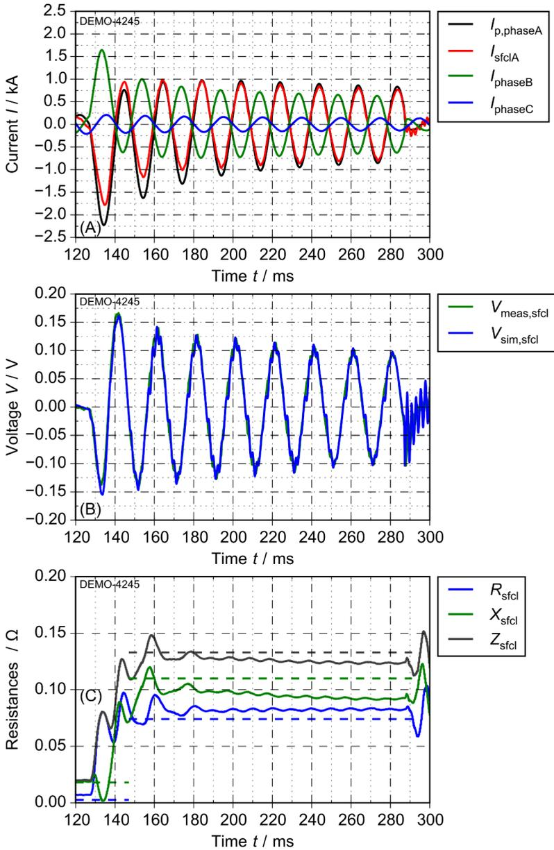
Figure 5.21: Results for fault current limitation of a 2-phase fault with ground connection for (a) currents, (b) voltages and (c) resistances ( $S_{base} = 180$  kVA,  $R_{fl} = 40$  m $\Omega$ ,  $p_f = 1.0$ )
