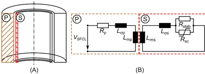
Figure 3.2: (A) Cross-section of the AC-SFCL and (B) equivalent circuit diagram showing the respective circuit for primary and secondary winding.
