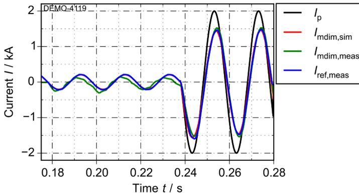
Figure 5.12: Comparison of results of the modified damping impedance feedback method for simulation and measurement with the reference measurement during load and fault cycles
