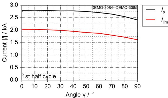
Figure 4.36: Measured fault limitation capability for a fault angles between  $0^\circ$  and  $90^\circ$  in the first half cycle
