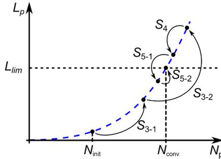
Figure 3.10: Iterative approach to calculate the inductance  $L_p$  of the primary winding. The number of turns is varied in discrete steps until the calculated impedance  $L_p$  matches the impedance necessary for fault current limitation.
