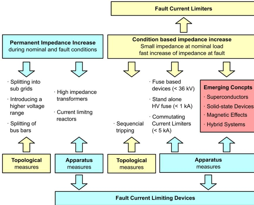
Figure 2.6: Overview of fault current measures according to [CIG12]
