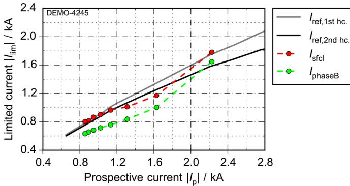
Figure 5.23: Summary of fault current limitation for unsymmetrical fault ( $S_{base} = 180$  kVA)
