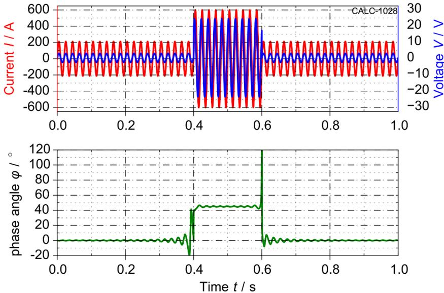
Figure C.4: Load-fault-load cycles. The phase angle between voltage and current is  $\varphi = 0^\circ$  during load and  $\varphi = 45^\circ$  during fault
