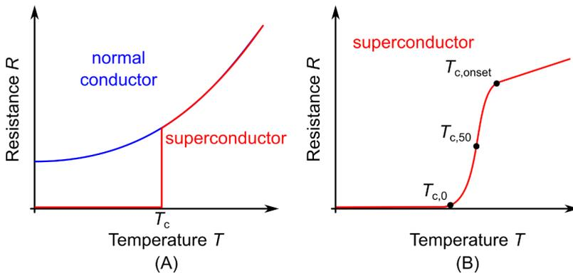
Figure 2.1: (A) Resistance depending on temperature for superconductors and normal conductors and (B) magnification around the transition and different definitions of the critical temperature [Cav98]
