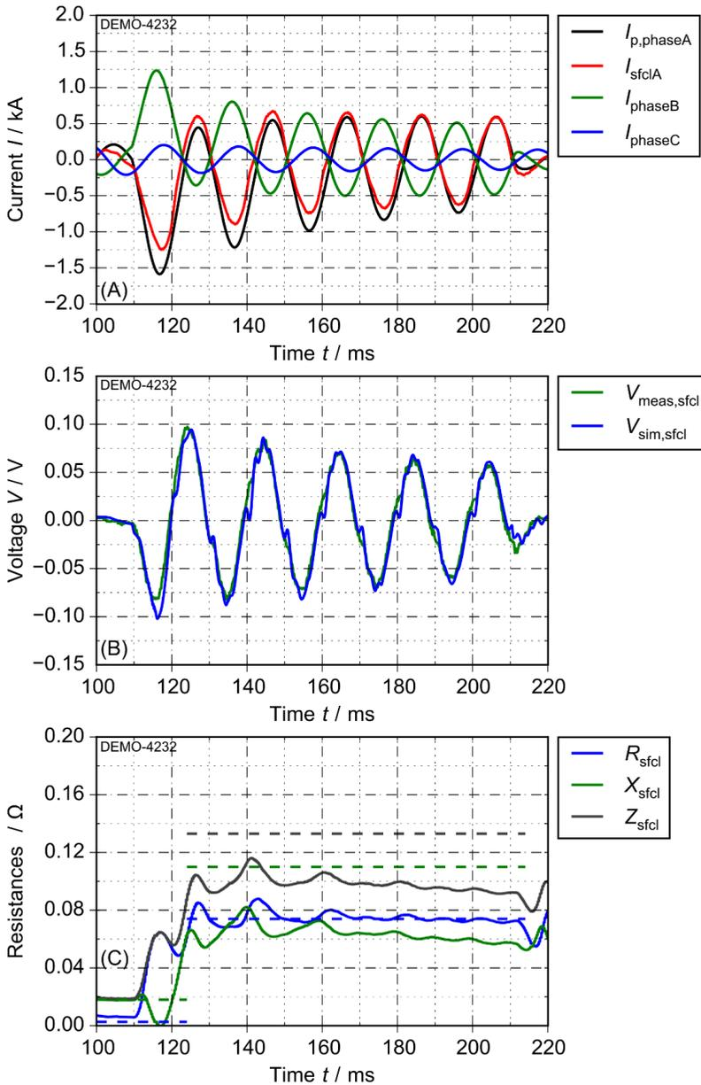
Figure 5.19: Results for fault current limitation of a 2-phase fault without ground connection for (A) currents, (B) voltages and (C) resistances ( $S_{base} = 120$  kVA,  $R_{lit} = 40$  m $\Omega$ ,  $p_{fcl} = 1.0$ )
