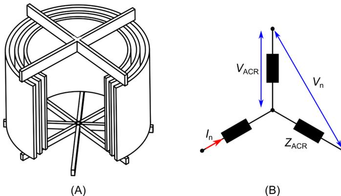
Figure 2.8: (A) Schematic of an air core reactor and (B) equivalent circuit with annotations for 3 air core reactors in Y-connection
