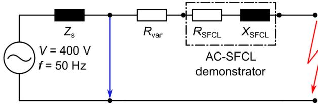
Figure 4.22: Equivalent circuit diagram of the calculated short-circuit
