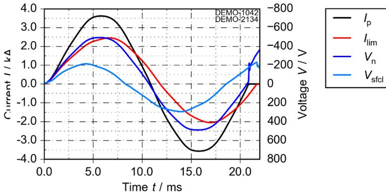
Figure 4.38: Fault current limitation for a fault of  $|I_p| = 3.6$  kA and a duration of two half cycles
