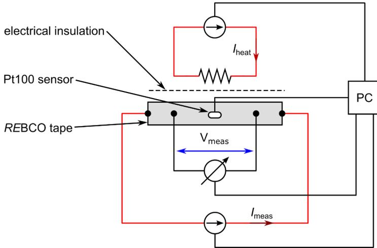
Figure 4.1: Diagram of the setup to measure the resistance depending on temperature  $R(T)$ . The REBCO tape is cooled down to 77 K and the slowly heated up. During the heating process a small current  $I_{\text{meas}}$  and the voltage drop across the tape  $V_{\text{meas}}$  are used to calculate the resistance  $R(T)$ .
