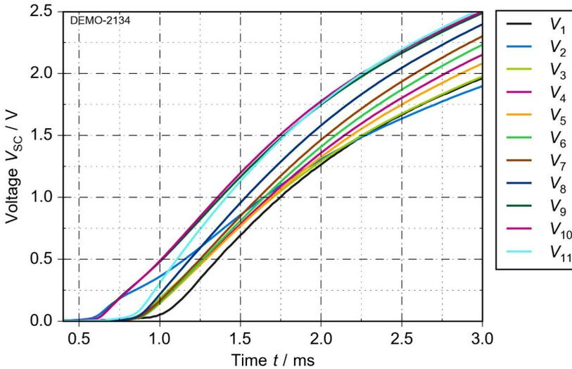
Figure 4.40: Magnification of the voltages at the *REBCO* tapes in the first half cycle, after engaging the fault
