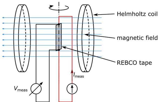
Figure 4.3: Schematic of the setup for measuring the critical current  $I_c(B, T)$ . A homogeneous magnetic field is generated using two Helmholtz coils. The REBCO tape is rotated within the magnetic field.
