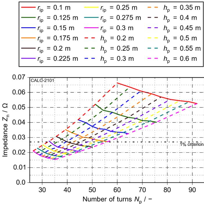
Figure 4.17: Results for impedance during normal operation of the demonstrator in the first design step (fill-factor  $f_{ip} = 0.85$ )
