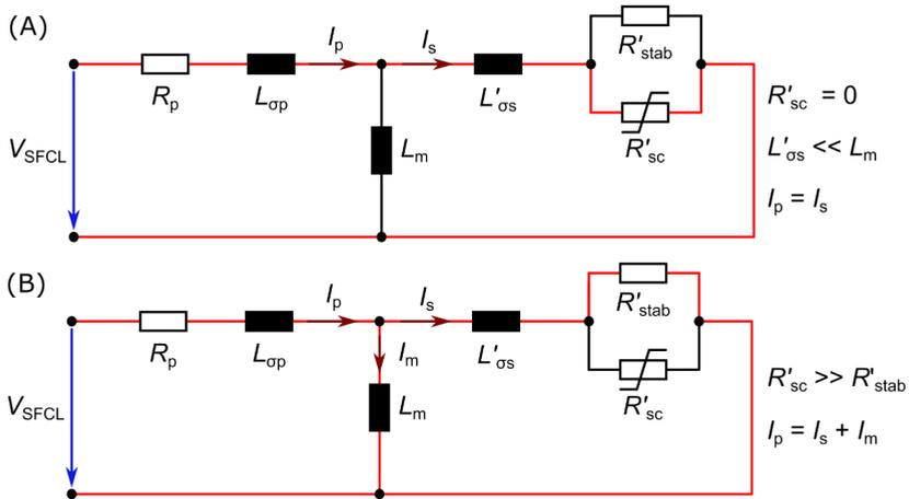
Figure 3.3: Modes of operation: (A) During normal operation the main inductance  $L_m$  is short-circuited and (B) during fault current limitation the resistance  $R'_{stab}$  and inductance  $L_m$  contribute to the total impedance
