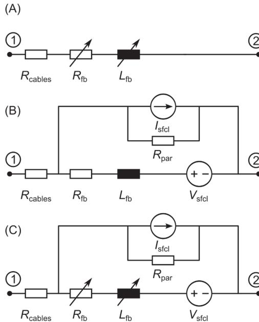
Figure 5.8: Equivalent circuit diagrams of (A) impedance feedback method, (B) classical damping impedance method and (C) modified damping impedance feedback method
