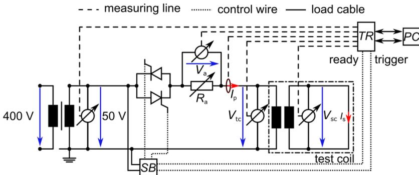
Figure 4.15: Measurement setup for quench experiments of single, short-circuited superconducting *REBCO* rings
