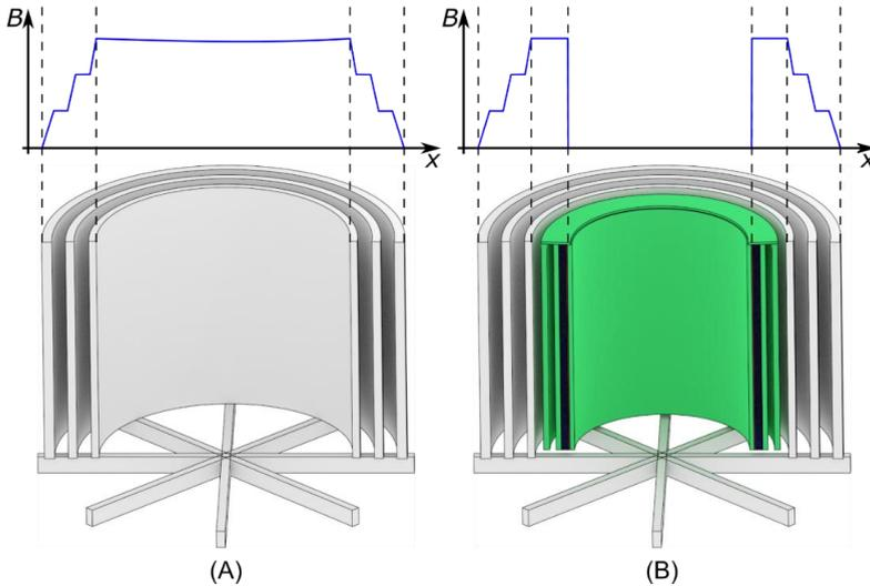
Figure 2.15: Magnetic field distribution in case of (A) the air core reactor and (B) the AC-SFCL during normal operation
