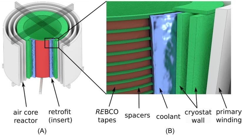
Figure 2.14: Schematic of the AC-SFCL: (A) Air core reactor with insert and (B) magnification of the insert showing the insulation and the winding
