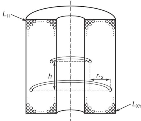
Figure 3.6: Cross-section of a solenoid winding divided into a finite number of current loops with two current loops indicated as in Figure 3.5
