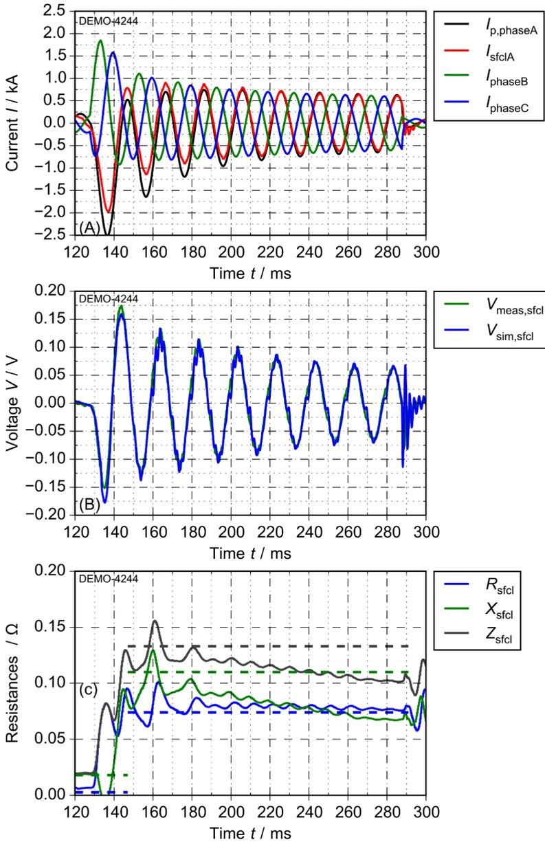
Figure 5.22: Results for fault current limitation of a 3-phase fault with ground connection for (a) currents, (b) voltages and (c) resistances ( $S_{base} = 180$  kVA,  $R_{lit} = 40$  m $\Omega$ ,  $p_f = 1.0$ )
