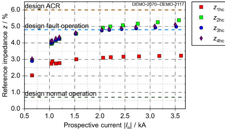
Figure 4.31: Calculated impedance of a fault of four half cycles for each half cycle depending on peak prospective current  $|I_p|$ . The calculated steady-state values are indicated.
