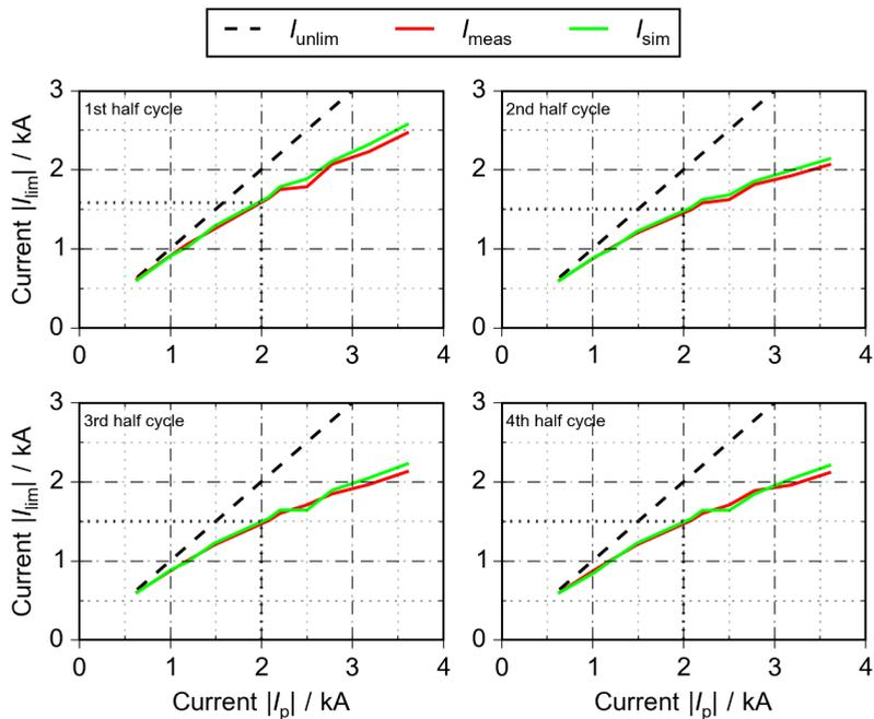
Figure 5.3: Comparison of the simulated model and measured results at KIT for fault current limitation for fault currents with increasing prospective current (the example in Figure 5.2 is indicated)
