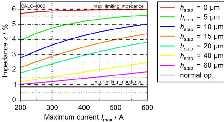
Figure 6.12: Dependency of the calculated impedance on critical current and stabilization for the low impedance design ( $d_w = 3$  cm)
