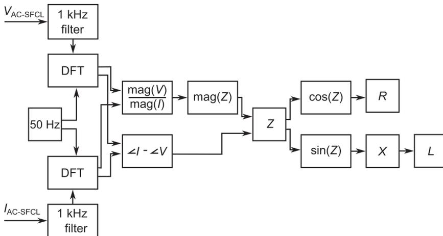
Figure 5.9: Approach to calculate instantaneous values of resistance and inductance from measured voltage and current
