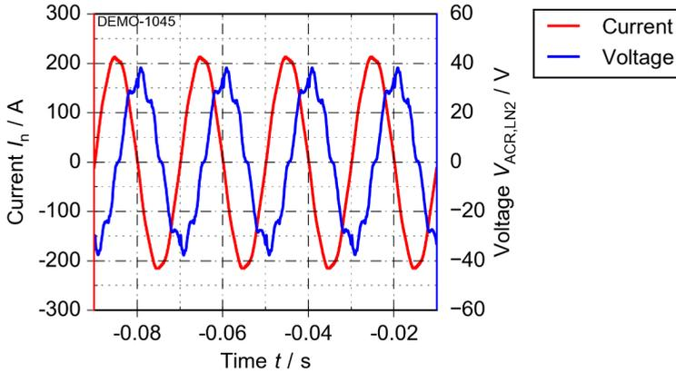
Figure 4.27: Measured current and voltage drop across the primary winding at 77 K during normal operation
