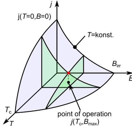
Figure 2.4: Combination of all three critical values to determine the point of operation with safety margins according to [Kom95]
