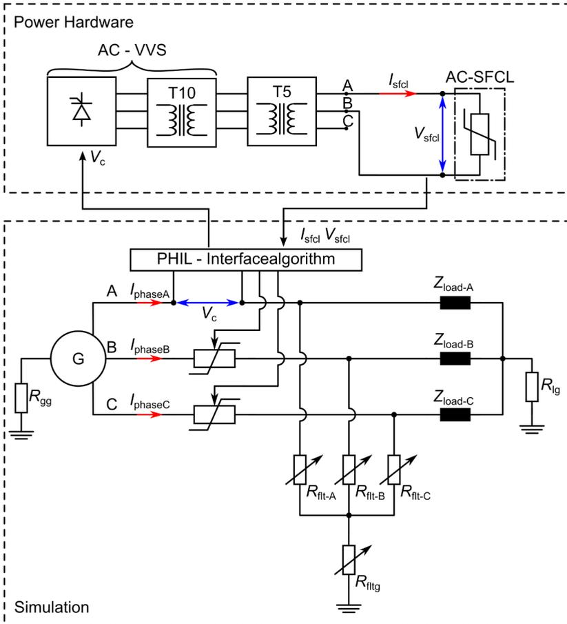
Figure 5.15: Three phase PHIL test setup. The Hardware part remained the same as in the preliminary tests shown in Figure 5.4
