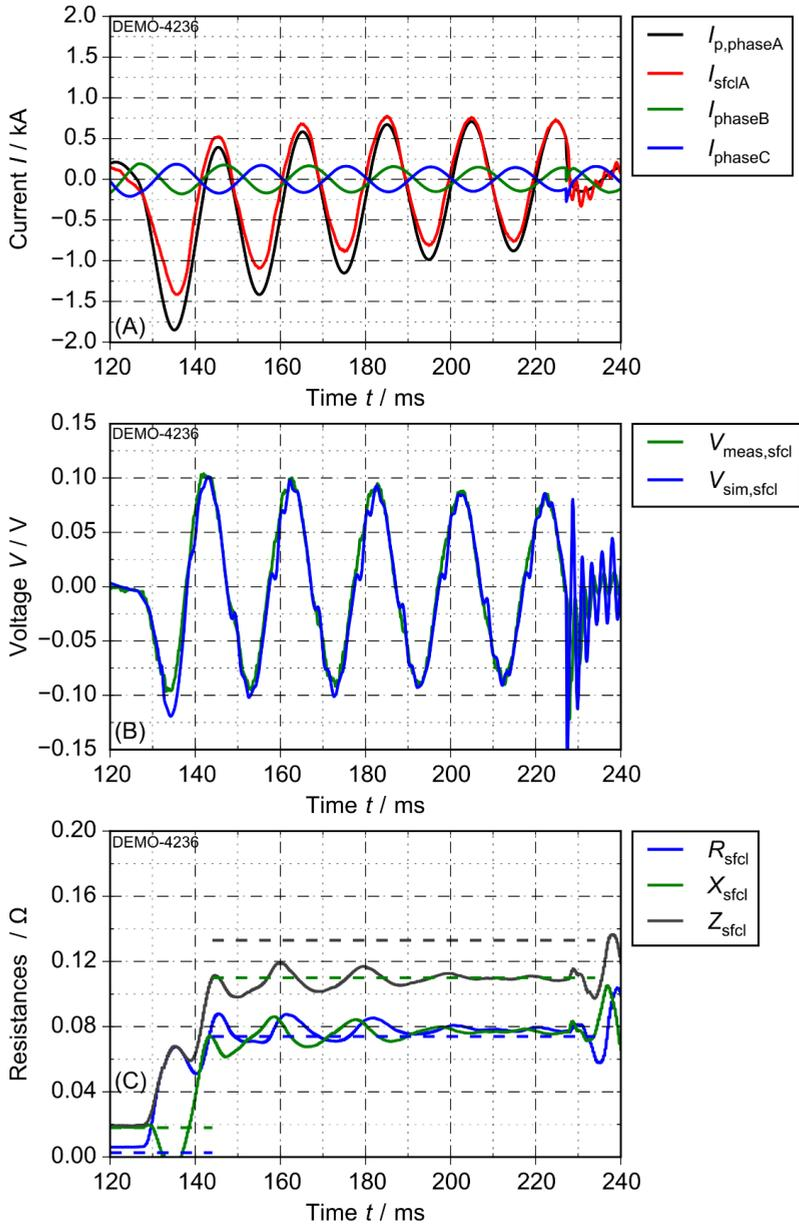
Figure 5.16: Results for fault current limitation of a 1-phase fault for (A) currents, (B) voltages and (C) resistances ( $S_{base} = 120$  kVA,  $R_{fit} = 40$  m $\Omega$ ,  $\rho_r = 1.0$ )
