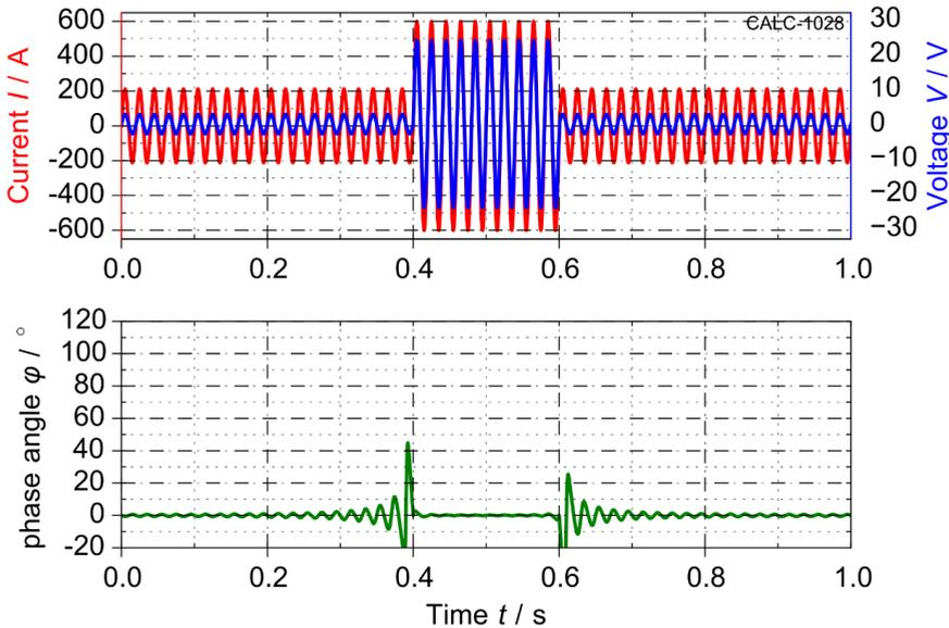
Figure C.3: Load-fault-load cycles. The phase angle between voltage and current is  $\varphi = 0^\circ$  during load and  $\varphi = 0^\circ$  during fault
