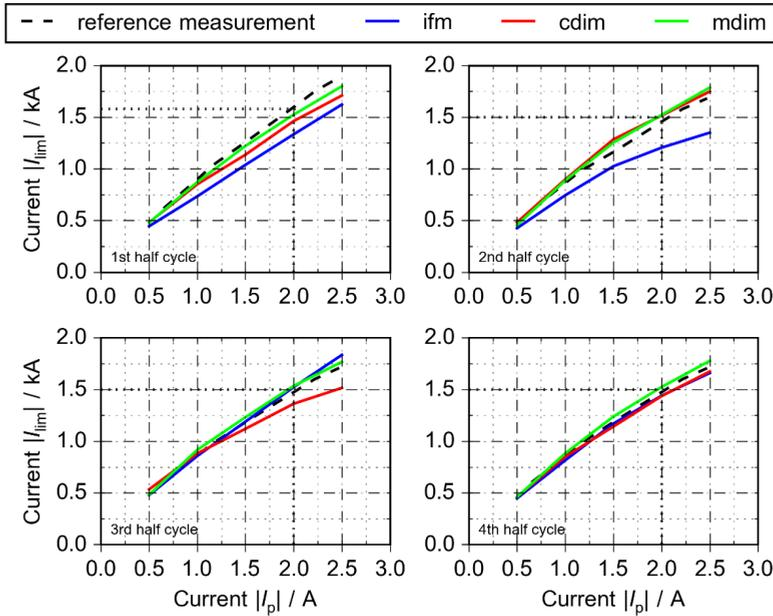
Figure 5.14: Comparison of current limitation of the three interface algorithms - measurement
