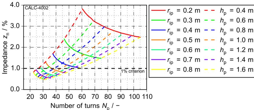
Figure 6.3: Calculated impedance during normal operation of 10 kV, 1 kA, z = 6% AC-SFCLs for variation of the geometry of the primary winding
