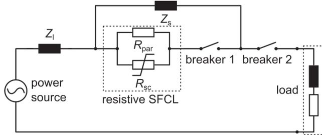
Figure 2.10: Circuit diagram of a resistive type SFCL with parallel impedance  $Z_s$  and circuit breakers
