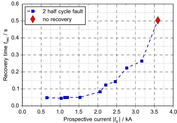
Figure 4.42: Summarized results of recovery under load. At  $|I_p| = 3.6$  kA the tape shown in Figure 4.41 is not recovering
