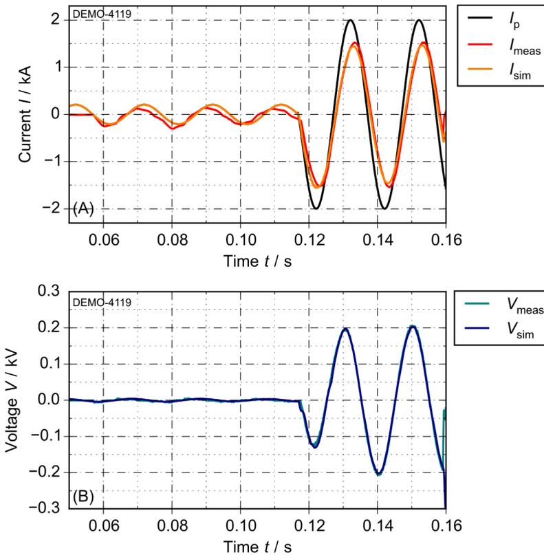
Figure 5.5: Comparison of results for three cycles load operation and limitation of a short-circuit current of  $I_p = 2$  kA with a duration of two cycles: (A) currents and (B) voltages
