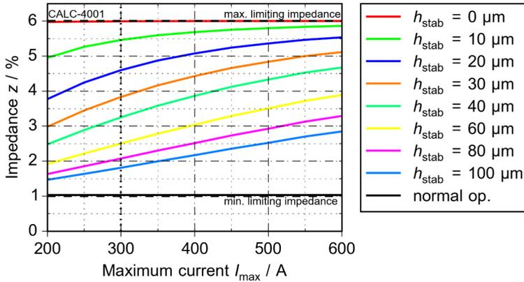
Figure 6.2: Calculated impedance of the retrofit for normal operation and fault condition for constant winding distance  $d_w = 2$  cm
