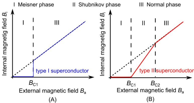
Figure 2.3: Behavior in an external magnetic field of (A) type I superconductors and (B) type II superconductors
