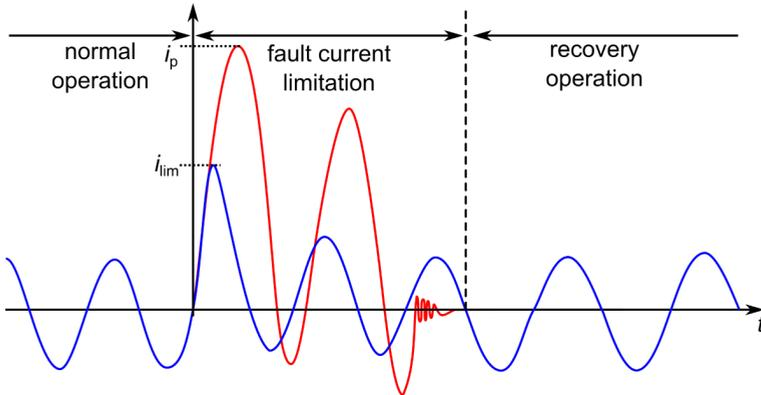
Figure 2.9: Operational modes of a superconducting fault current limiter. The red curve shows the unlimited fault current and the blue curve the limited fault current
