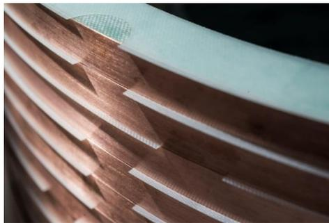
Figure 4.21: Close-up of the secondary winding. The REBCO tapes can be identified by their brushed copper surface. Spacers between the REBCO tapes keep the tapes separated and at position, while the cuttings in the spacers allow the flow of liquid nitrogen.
