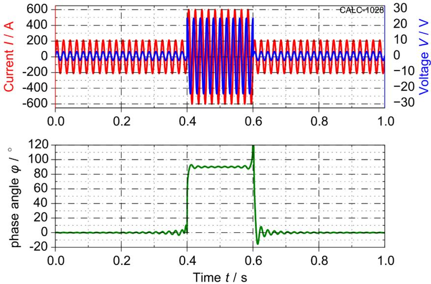
Figure C.5: Load-fault-load cycles. The phase angle between voltage and current is  $\varphi = 0^\circ$  during load and  $\varphi = 90^\circ$  during fault
