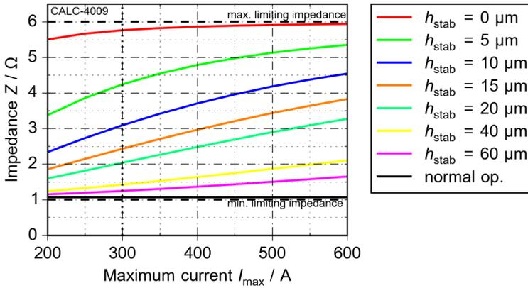
Figure 6.18: Dependency of the calculated impedance on critical current and stabilization for the low impedance design ( $d_w = 10$  cm)
