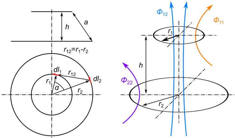
Figure 3.5: Two coaxial current loops with radii  $r_1$  and  $r_2$  and distance  $h$
