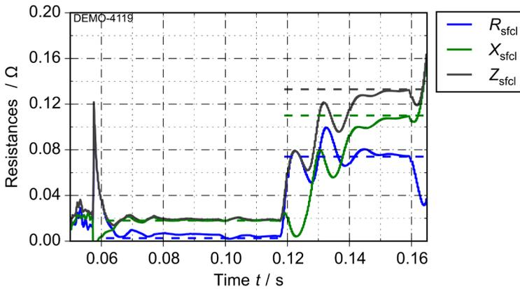
Figure 5.6: Calculated values for resistance, reactance and impedance during the load and the fault cycle. The respective design values for load and fault are plotted as dashed lines.
