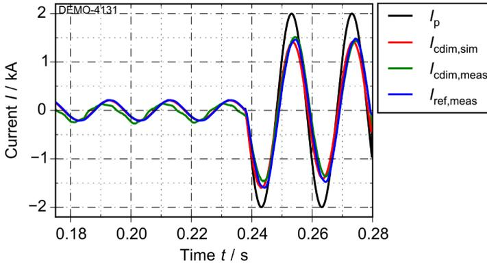
Figure 5.11: Comparison of results of the damping impedance feedback method for simulation and measurement with the reference measurement during load and fault cycles
