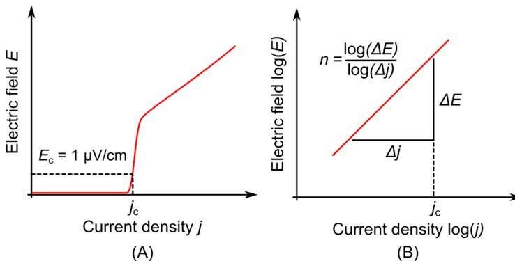
Figure 2.2: (A) Definition of the critical current density  $j_c$  and (B) definition of the n-value
