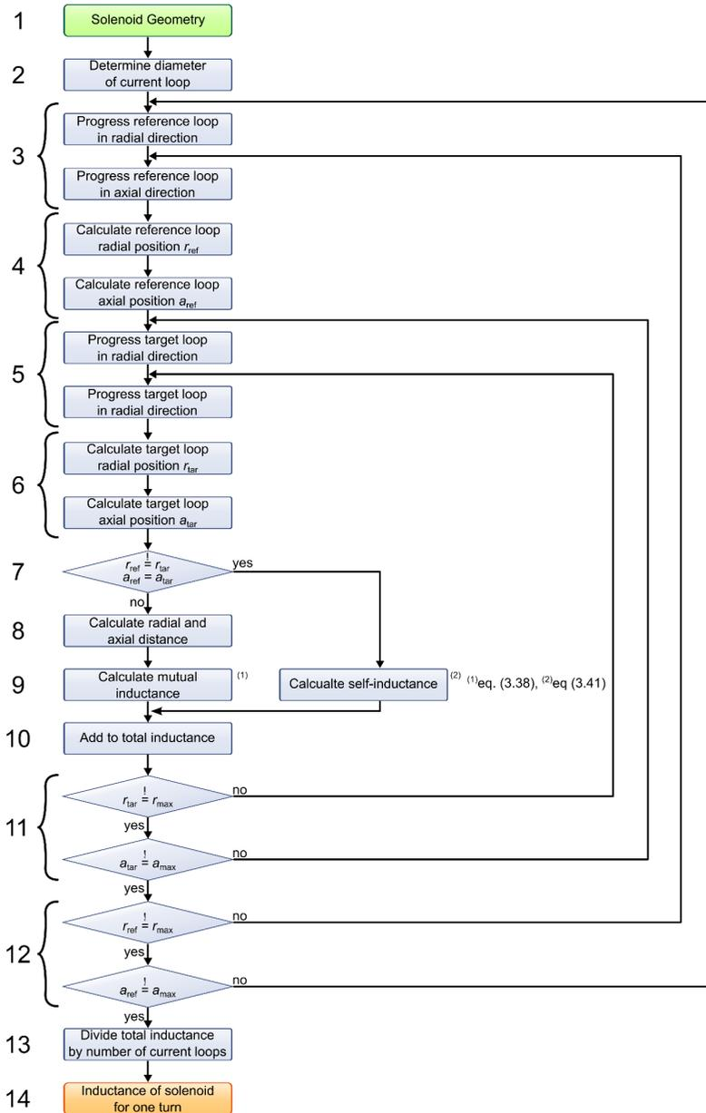
Figure B.1: Flow diagram of the function to calculate the inductance of a solenoid with arbitrary cross section
