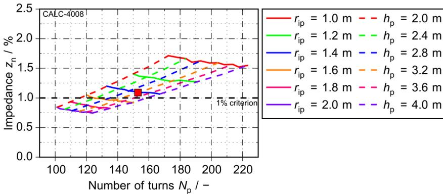
Figure 6.16: Results for impedance during normal operation of 380 kV, 1 kA, z = 6% AC-SFCLs for variation of the geometry of the primary winding. The red square indicates the chosen low impedance design
