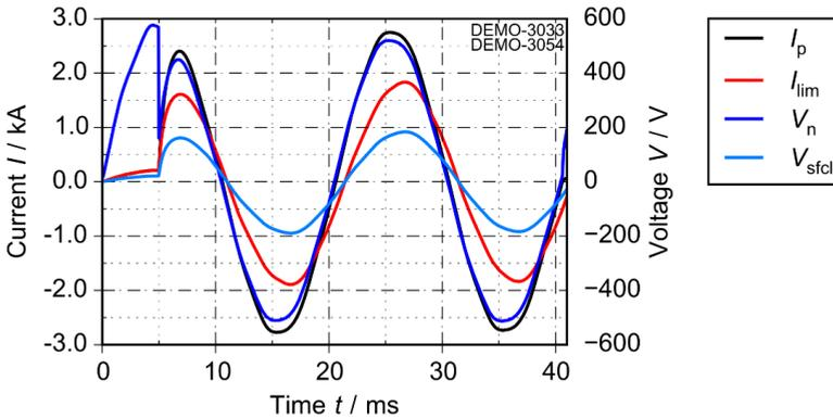
Figure 4.35: Measured limitation of a fault current of four half cycles triggered at a fault angle of  $\gamma = 90^\circ$  and a prospective fault current of 2.5 kA in the first half cycle-.
