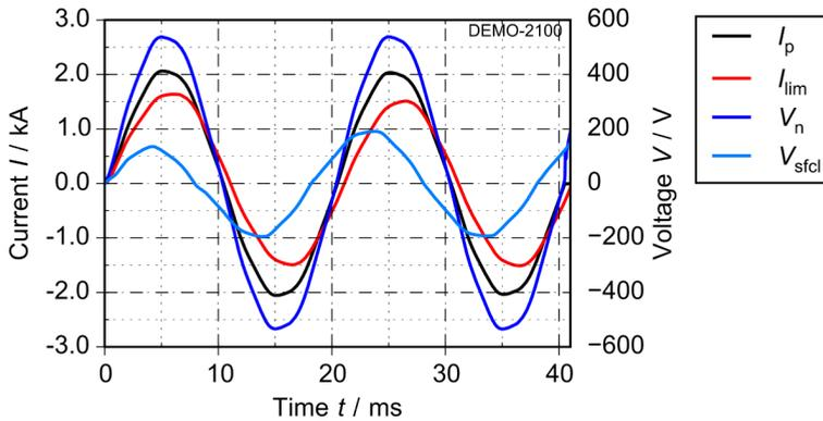
Figure 4.29: Fault current limitation for a fault of four half cycles
