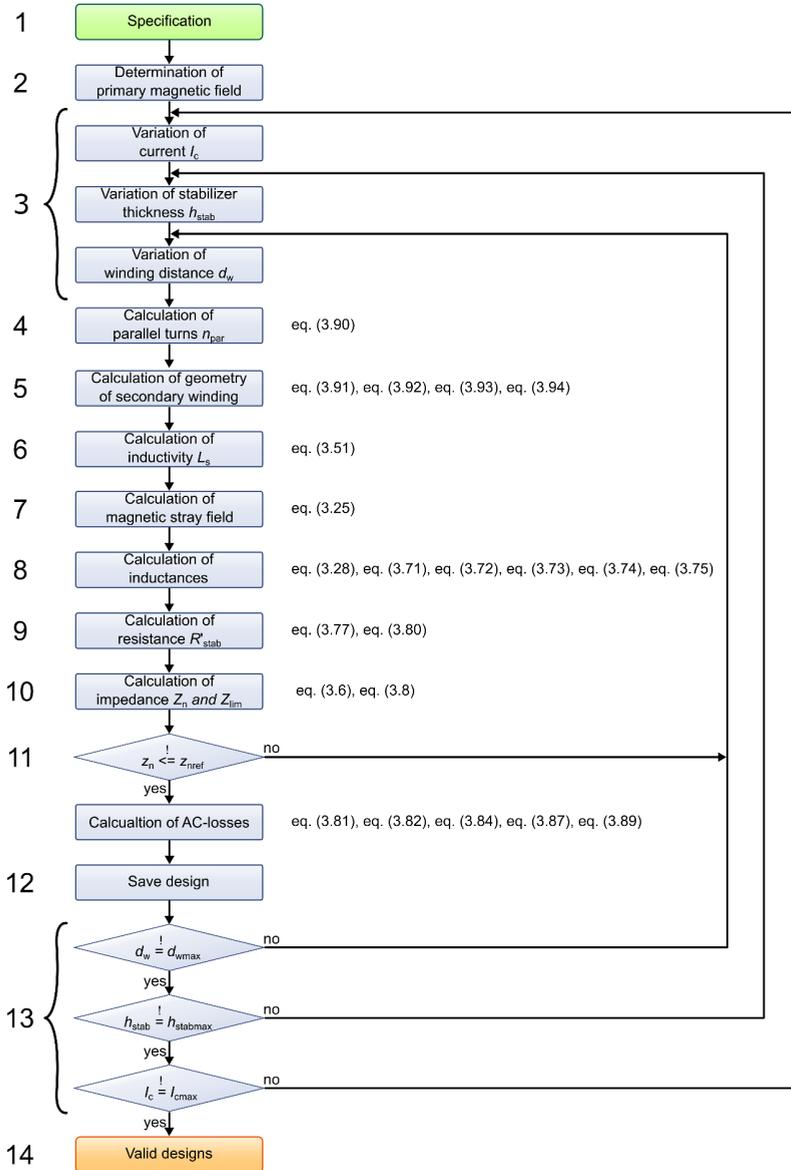
Figure 3.9: Flow diagram for calculation of the retrofit. Assuming constant parameters for the primary winding a secondary winding is calculated. If the impedance of the design during normal operation the AC-losses of the AC-SFCL design are calculated and the design is stored.
