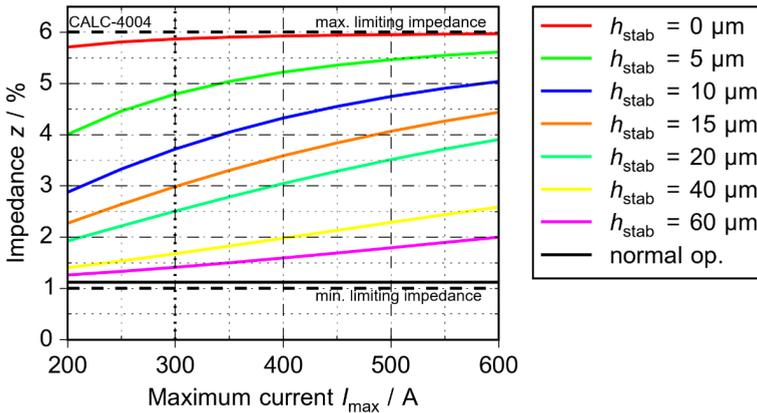
Figure 6.9: Calculated impedance of the retrofit for normal operation and fault condition for constant winding distance  $d_w = 3 \text{ cm}$
