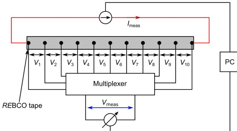
Figure 4.7: Setup to measure critical current distribution of each *REBCO* tape intended for the use in the AC-SFCL demonstrator. The current is increased in discrete steps and the voltage drop of each section is measured after each current increase.
