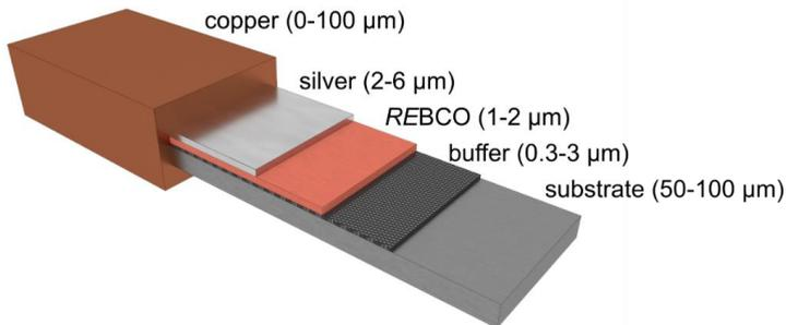
Figure 2.5: Typical layered structure of a *REBCO* conductor. Thickness and width of the layers are not to scale
