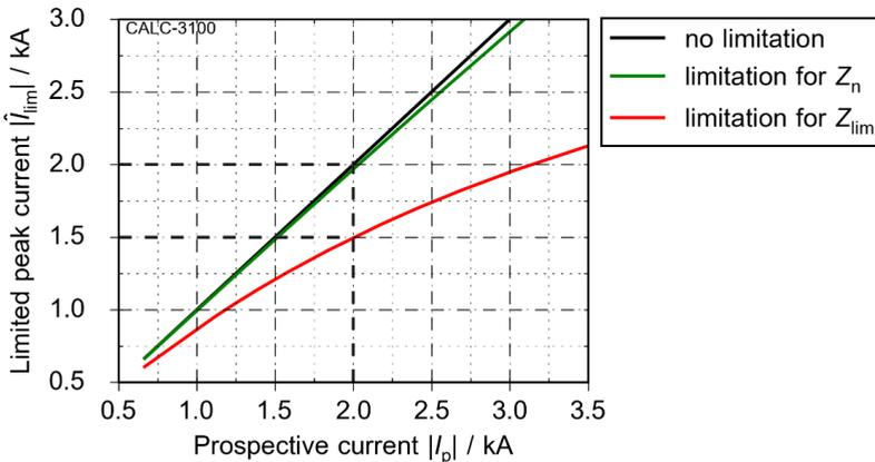
Figure 4.24: Simulation of expected progression of peak limited short-circuit current  $|I_{lim}|$  with peak prospective current  $|I_p|$ . The example in Figure 4.23 is indicated.
