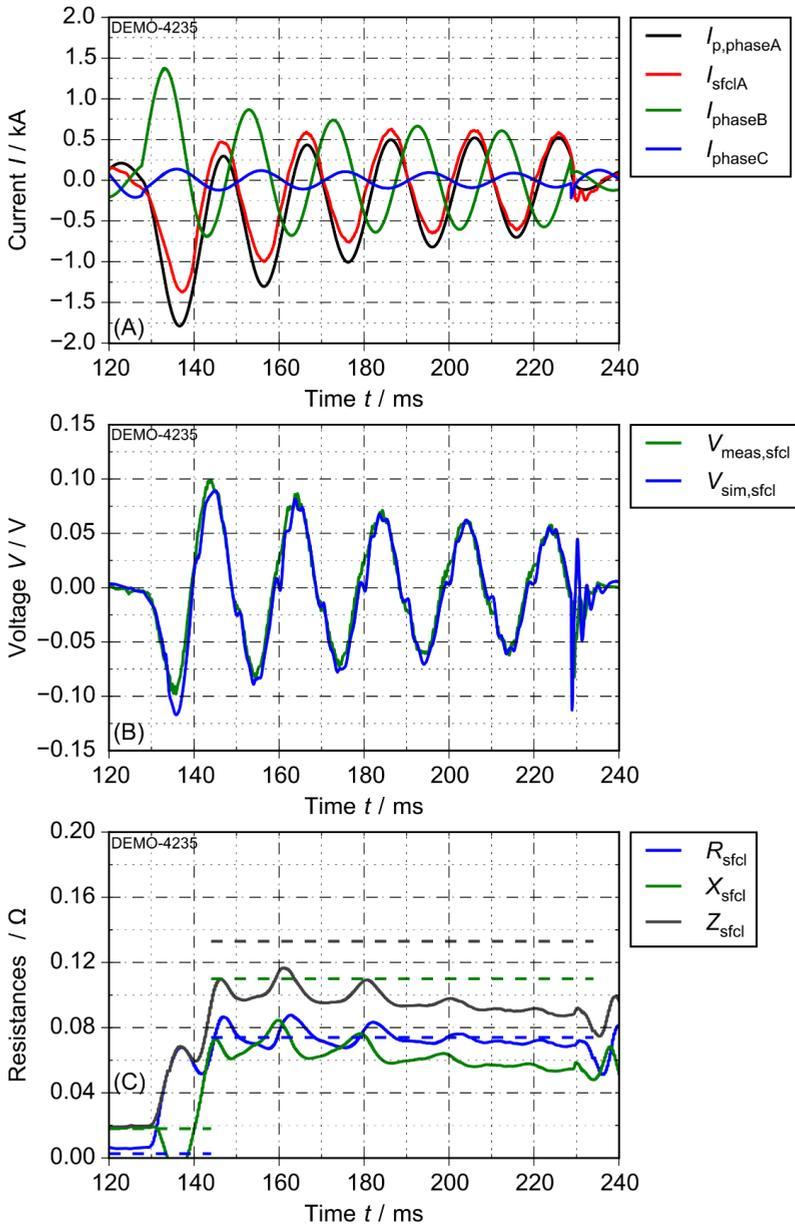
Figure 5.17: Results for fault current limitation of a 2-phase fault with ground connection for (A) currents, (B) voltages and (C) resistances ( $S_{base} = 120$  kVA,  $R_{flt} = 40$  m $\Omega$ ,  $p_f = 1.0$ )
