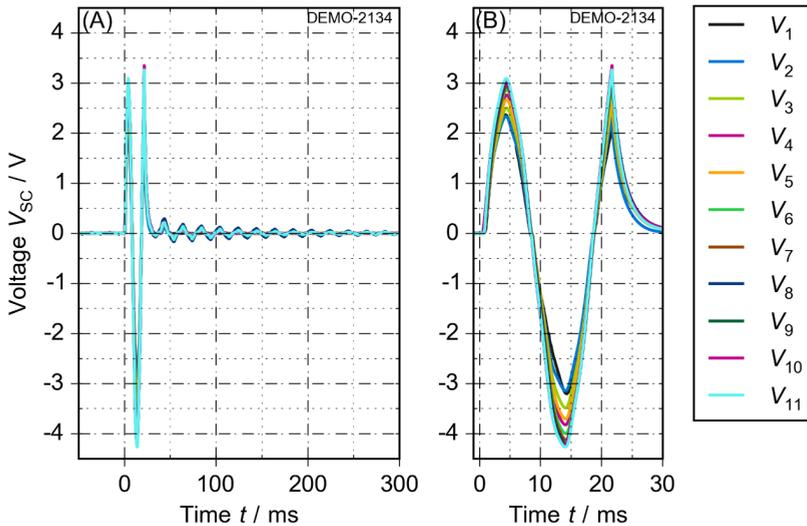
Figure 4.39: Voltage signals at the *REBCO* tapes during fault current limitation for a fault of two half cycles (A) including the load cycle and (B) magnified on the fault.
