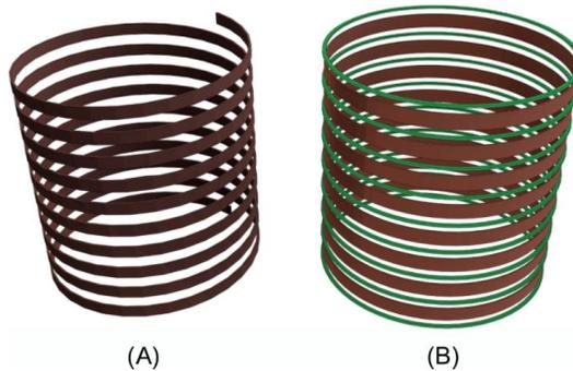
Figure 2.16: (A) Conventional solenoid winding and (B) winding consisting of stacked rings with spacers
