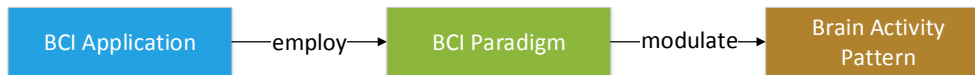
Figure 1.4 – Summary of the structural relationship between BCI applications, BCI paradigms and brain activity patterns.
