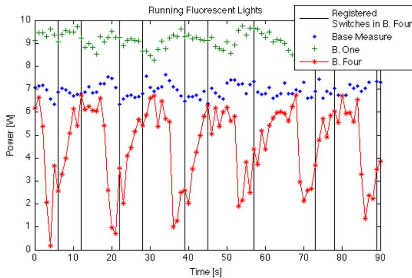
Figure 4.9: Time series profile of the fluorescent light with registered likelihood changes marked
