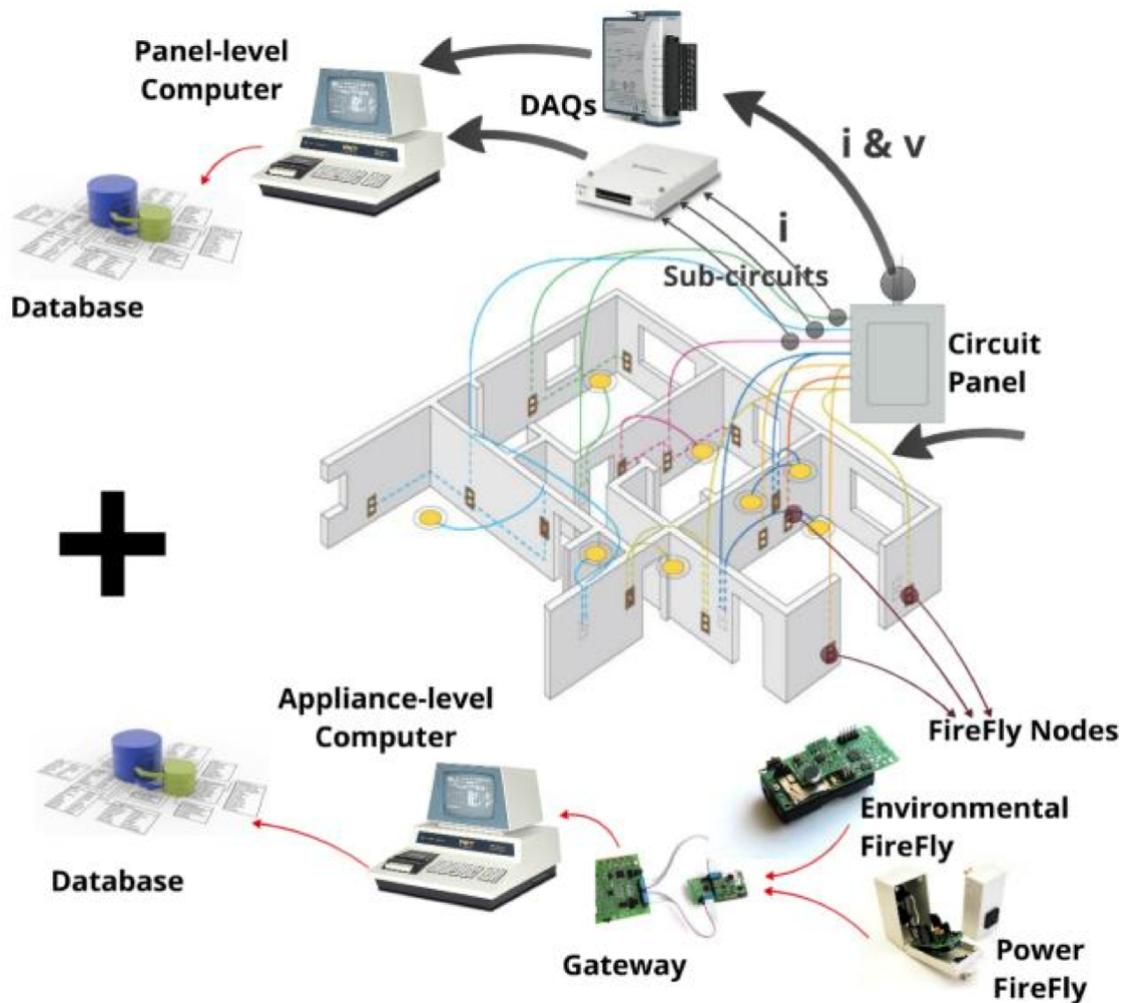
Figure 6.2: BLUED setup for data and ground truth collection (Anderson et al., 2012).
