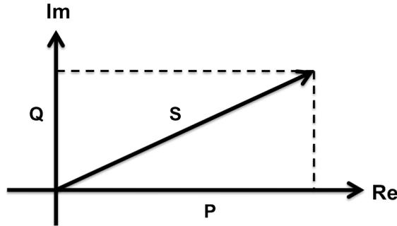
Figure 4.4: Apparent power ( $S$ ) as the vector sum of the real ( $P$ ) and reactive power ( $Q$ )
