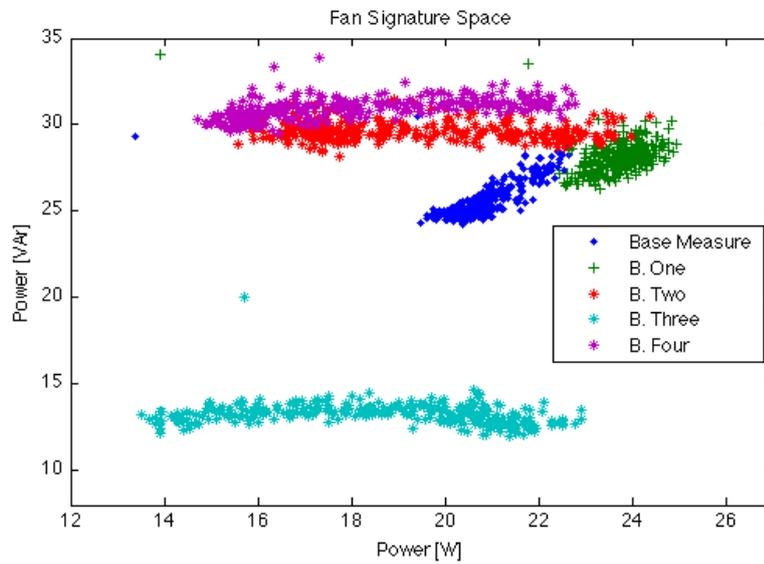
Figure 4.8: Real and reactive power measurements from the table fan.
