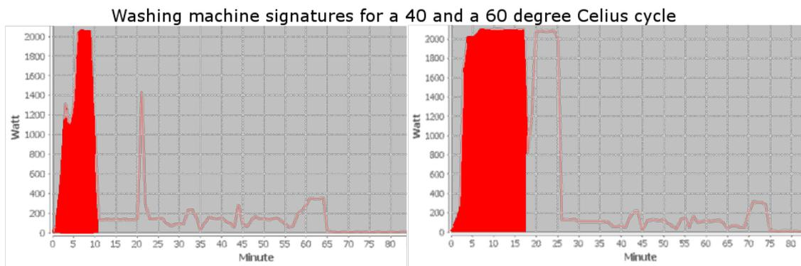
Figure 6.6: Disaggregated states for a washing machine, showing the heating power surges used for setting determination marked. With the area below the graph representing the energy used during a certain time-span
