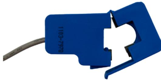
Figure 4.2: Ferrite split-core current transformer (CT) with  $n = 2000$  turns and a maximum current restriction of  $I_{max} = 100A$ .
