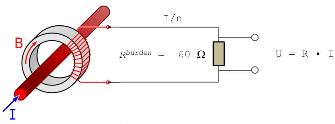
Figure 4.3: Physical Working Principle of power measurement by induction.
