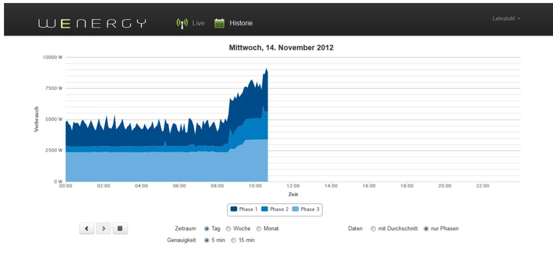
Figure 5.3: Web-based live feedback view based on three phase measurements
