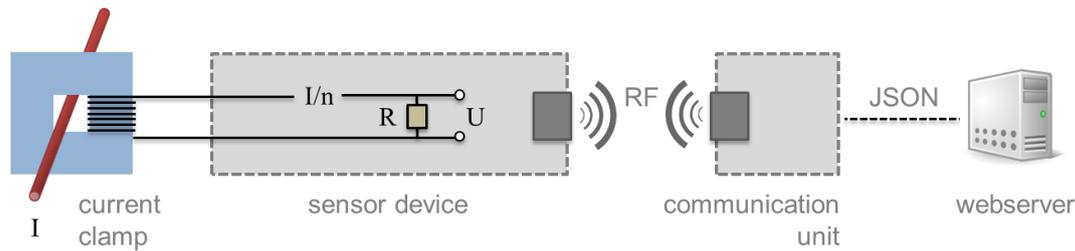
Figure 4.1: Measurement System Overview: power line (single phase), current clamp sensor, sensor device, communication unit, web server
