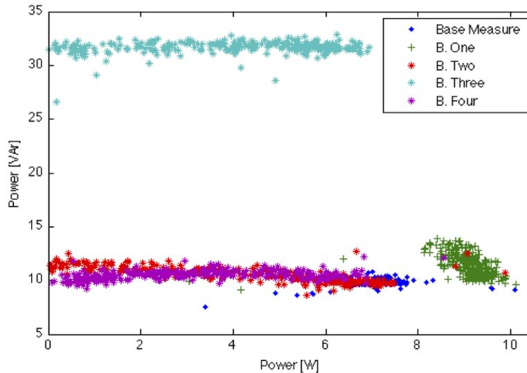
Figure 4.7: Real and reactive power measurements from the fluorescent light.
