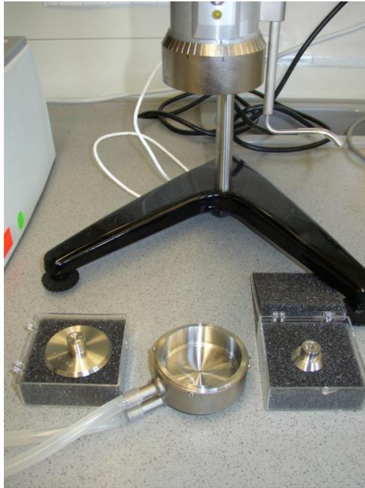
Abb. 2.4: Viskosimeter Brookfield RVDV-II
