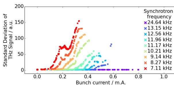
Figure 3: The standard deviation of the THz signal displayed over bunch current is shown for different settings of the magnet optics (with constant RF-voltage), which result in different synchrotron frequencies indicated by color [7].
