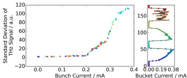
Figure 2: The calculated standard deviation of the THz signal of each bunch is plotted over the corresponding bunch current. The current profile was patterned to resample the whole current range.
