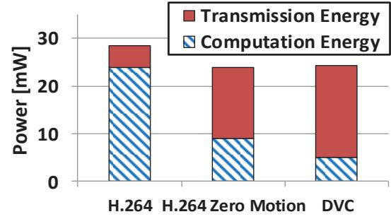
Figure 2-12: Comparing the computational and transmission power for an ASIC-based video sensor [82]
