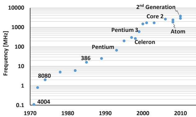
Figure 1-2: Evolution of Intel processors
