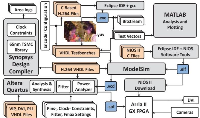
App-Figure C-1: Simulation and design methodology of the proposed multicast H.264/AVC video encoder.
