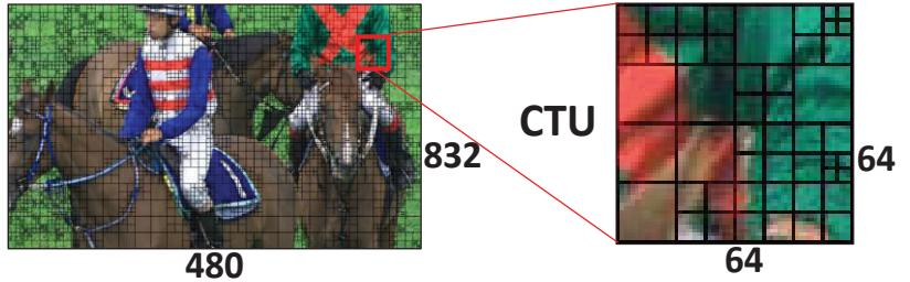
Figure 2-5: Video sequence “RaceHorses” with overlaid PU structure after HEVC processing, with a CTU of  $64 \times 64$
