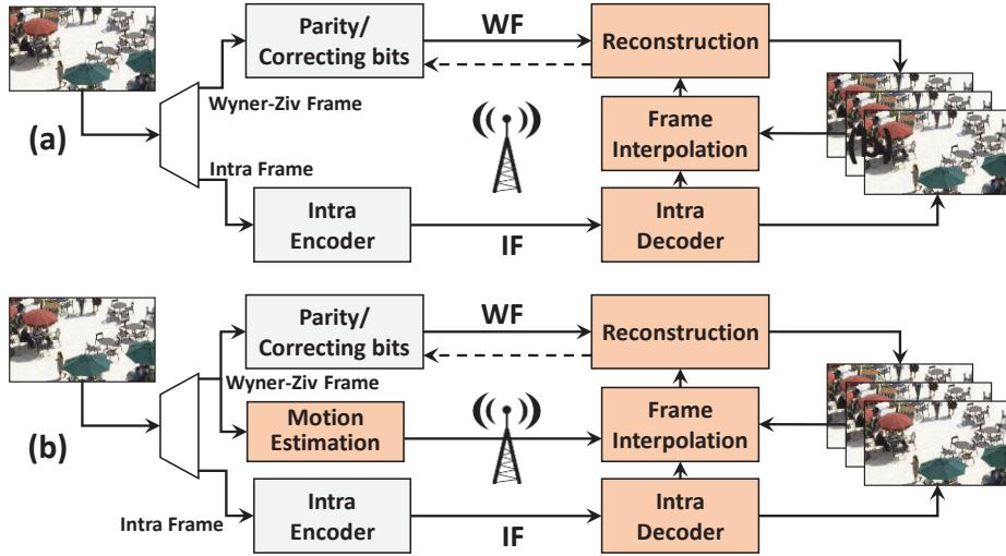
Figure 2-14: (a) Distributed Video Coding, DVC and (b) Hybrid Distributed Video Coding (HDVC)
