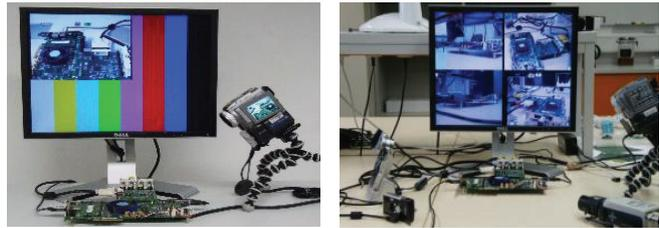
App-Figure C-3: Prototype implementation on Altera's Arria II GX FPGA.
