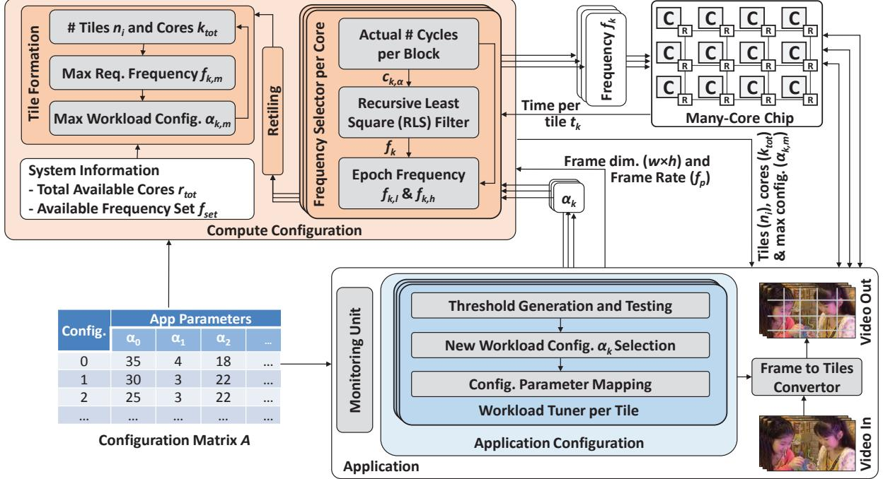
Figure 4-2: Power efficient workload balancing approach on a many-core platform.
