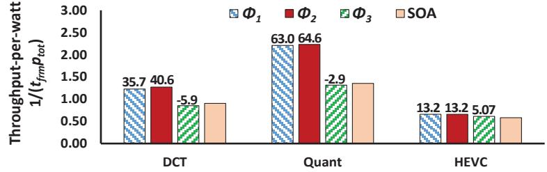
Figure 6-8: Average throughput per watt  $1/(t_{frm} \times p_{tot})$  for different efficiency indices and State-of-the-Art (SOA) [2]. The percentage improvement against SOA is written on top of the bars.
