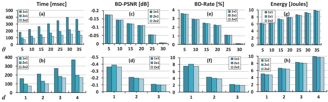
Figure 4-10: Impact of  $\theta$  and  $d$  on (a, b) time per frame, (c, d) BD-PSNR, (e, f) BD-Rate [59] and (g, h) energy with different tile settings using “Keiba” sequence ( $832 \times 480$ ). The anchor encoding is done with 1 tile, maximum  $\theta$  and  $d$ .
