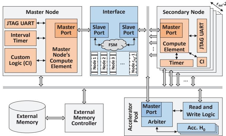
Figure 5-3: Heterogeneous system with custom hardware components
