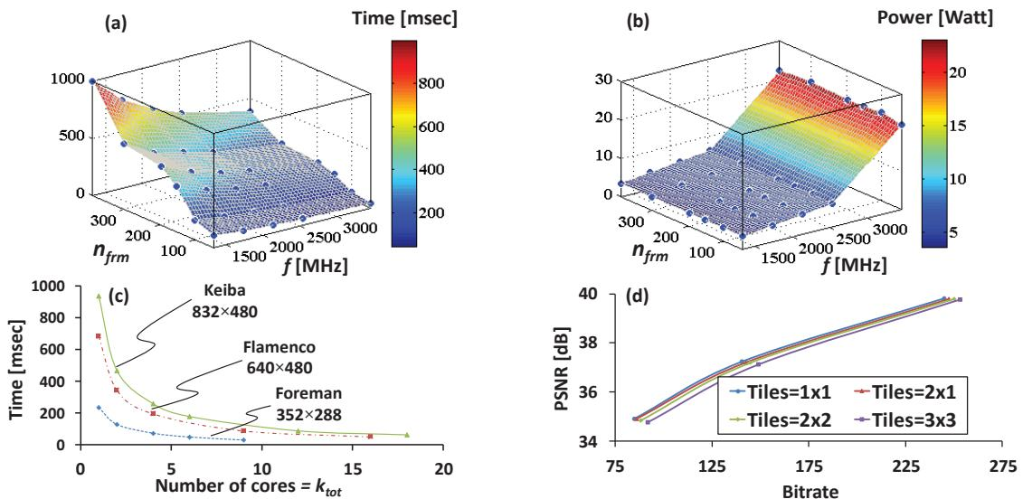
Figure 3-3: (a) Average time (msec) at different frequencies, (b) power consumption for different frequencies and frame sizes, (c) at  $f=2.16$  GHz, average time (msec) per frame with varying number of cores and (d) PSNR Vs. Bitrate plot by using "Foreman" video sequence ( $352 \times 288$ ) for HEVC encoding
