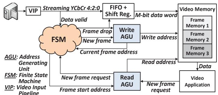
Figure 2-2: Video memory management system for storing raw video samples in the video memory
