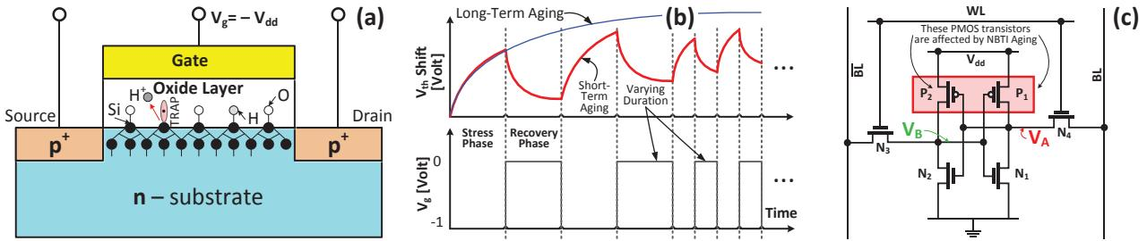
Figure 2-16: (a) PMOS transistor under NBTI aging with breaking Si-H bond at the Si-SiO<sub>2</sub> interface, (b) Stress and recovery phases for a PMOS transistor, and (c) Standard 6-T SRAM cell.
