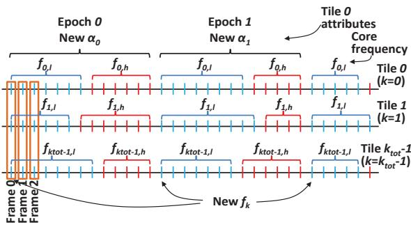
Figure 4-8: An example frequency and workload allocation to collocated tile in video application
