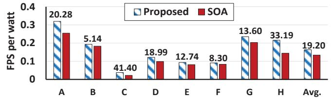
Figure 6-3: Comparing the power-efficiency (fps per watt) of the proposed workload balancing approach employing compute and application configuration compared to State-of-the-Art (SOA) [1]. The percentage improvement of our scheme is written on top of the bars.
