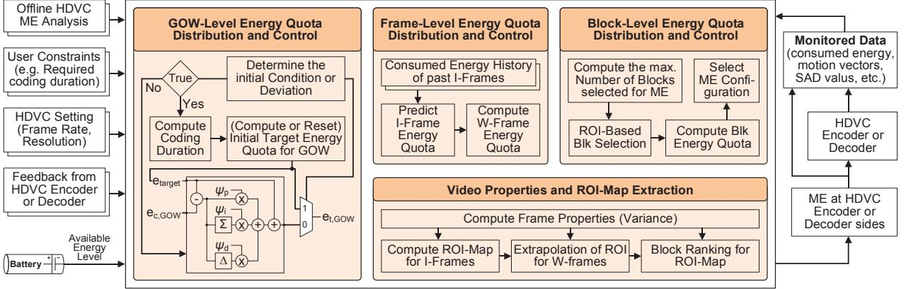
Figure 4-23: Operational flow of the proposed hierarchical energy budgeting for HDVC. Here, Blk: Block.
