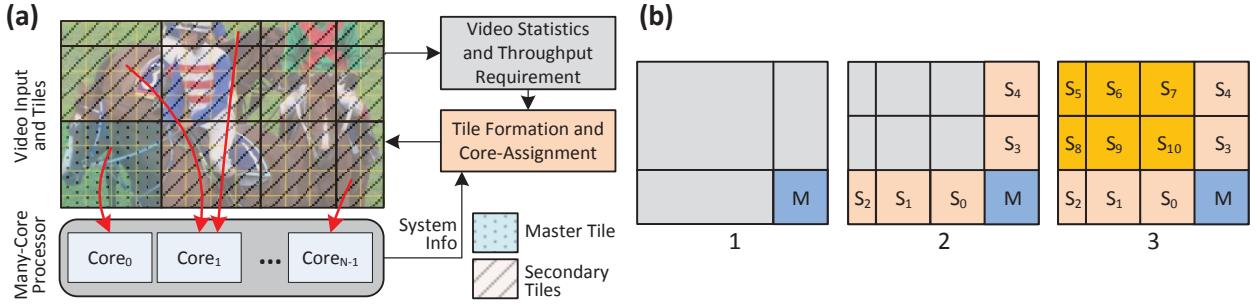
Figure 4-4: (a) Non-uniform tiling and cores assignment, (b) Master and secondary tile formation scheme
