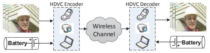
Figure 4-21: Video capture and wireless transmission scenario with resource constrained video encoder(s) and decoder(s).
