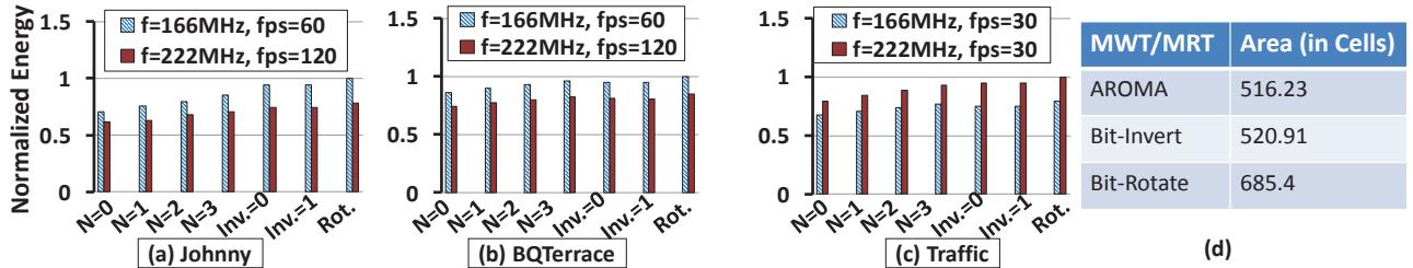
Figure 6-20: (a-c) Energy consumed per frame of MWTs and MRTs at different frequency and FPS configurations. (d) Total area (in cells) for different MWTs/MRTs. Inv.= 0 denotes that the Invert MWT/MRT is inactive while Inv.= 1 denotes active Invert MWT/MRT. Rot. denotes Rotate MWT/MRT
