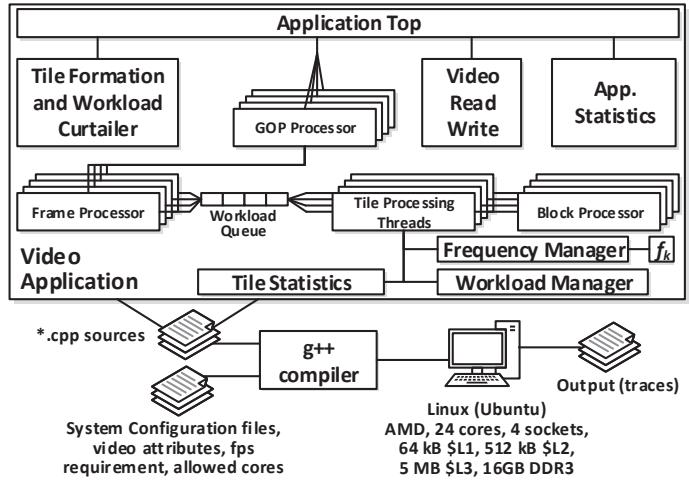
Figure 6-1: Simulation setup and multithreaded video application design
