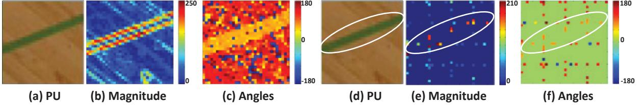
Figure 4-11: (a-c) Gradient generation for estimating the best Intra angular mode using [123], (d-f) proposed gradient generation with downsampled data
