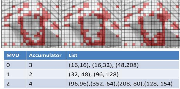
Figure 4-24: (top) ROI identification and then extrapolation for two W-frames, (bottom) example hash-table to store ROI map
