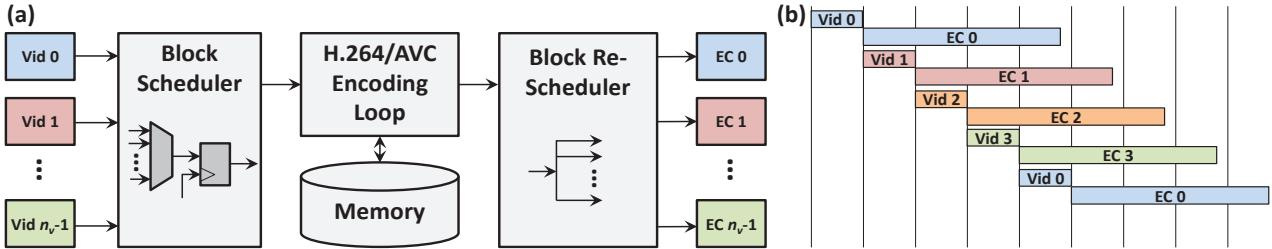
Figure 5-9: (a) Block processing scheduler and (b) example schedule with  $n_v=4$
