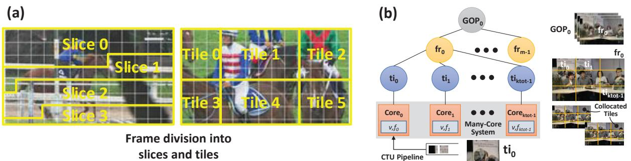
Figure 2-10: (a) Frame division into slices and tiles for parallel processing, (b) Video partitioning hierarchy. Here, fr: frame, ti: tile
