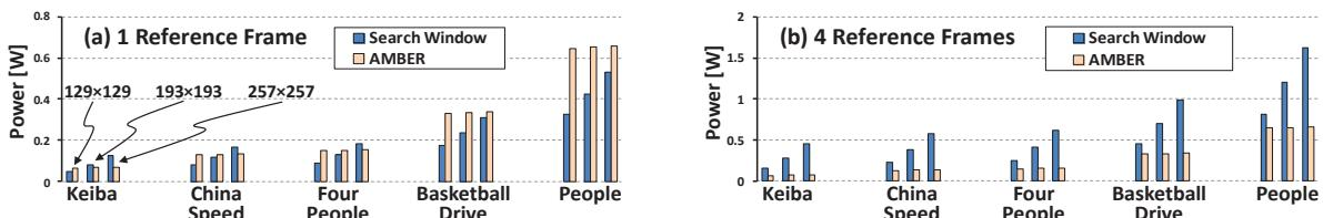
Figure 6-16: Comparing power consumption for the search window approach and AMBER, using (a) one reference and (b) four reference frames for ME of HEV Inter-encoding
