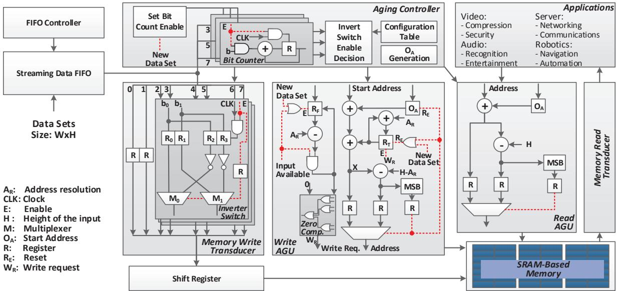
Figure 5-24: Overview of the proposed SRAM memory anti-aging architecture. Note the Memory Write Transducer, Write AGU, Read AGU and Memory Read Transducer connected to the SRAM. The aging controller configures these units by generating appropriate signals to adapt input data at read and write ports of the memory
