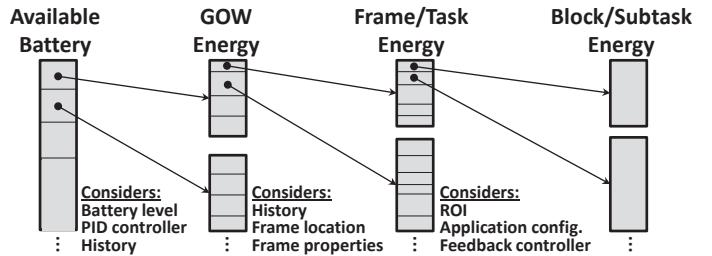
Figure 4-22: Energy quota distribution at different hierarchical levels
