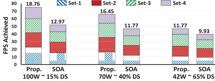
Figure 6-9: Fps achieved using proposed resource budgeting approach and State-of-the-Art (SOA) [3] for different amount power budgets (Dark Silicon, DS). The average fps per set is written on top of the bars.
