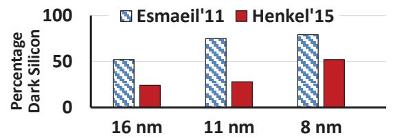
Figure 2-15: Dark Silicon prediction trends. Here, Esmaeil'11 is [8] and Henkel'15 is [299].
