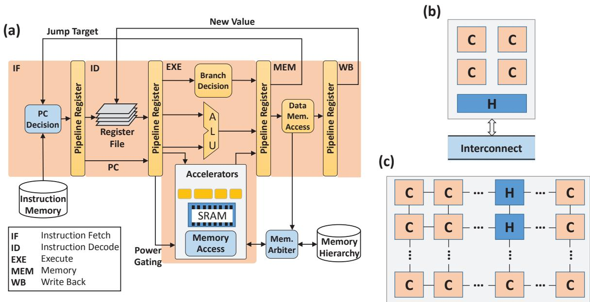
Figure 2-18: Accelerator locality, (a) In-core, (b) tightly coupled, (c) loosely or decoupled accelerators
