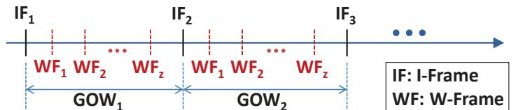
Figure 2-13: Group of WF (GOW) structure showing IFs and WFs
