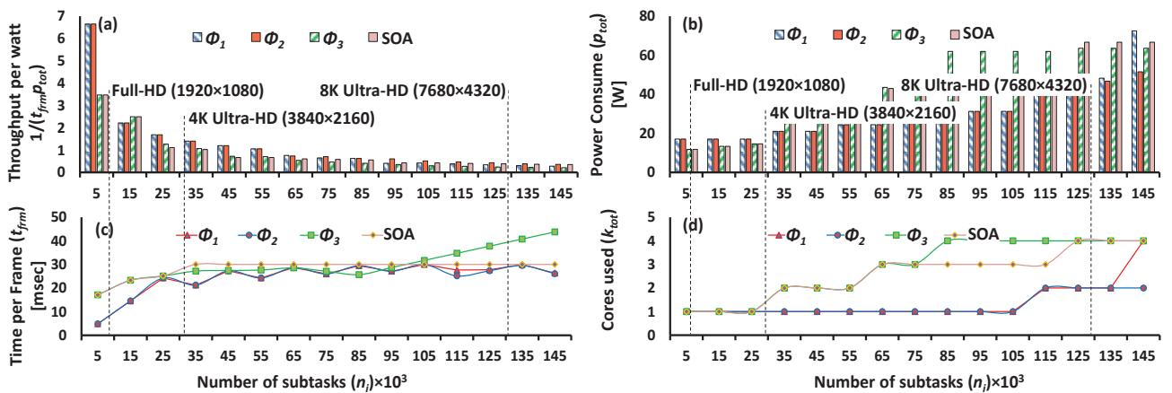
Figure 6-7: (a) Performance of the proposed and State-of-the-Art (SOA) [2] approaches for the “DCT” benchmark. The number of DCTs (or subtasks) for different image resolutions are portrayed on top of the graph. For the “Quant” benchmark, (b) power consumption, (c) time per frame and (d) number of cores used is given for different  $n_i$ , using our proposed efficiency indices and State-of-the-Art (SOA) [2] approach.
