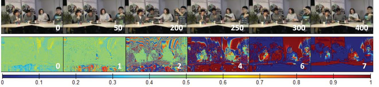
Figure 3-14: (top) Video sequence “FourPeople” ( $1280 \times 720$ ) with frame numbers written and (bottom)  $\Delta$  stressmaps for specific bits of the video sequence, by plotting duty cycle ( $\Delta$ ) of the specific bit on spatial scale. The higher order bits have a biased  $\Delta$  whereas the  $\Delta$ s of lower order bits are self-balancing
