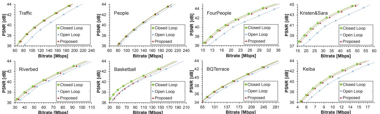
Figure 5-19: PSNR vs. Bitrate plot for proposed and open loop  $\theta=1$ ; each value represents the average results for QP sweeps from 18 to 32 (step size = 2)
