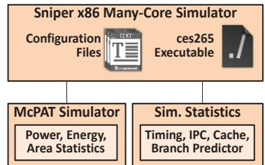
App-Figure B-2: Sniper simulator setup to run ces265
