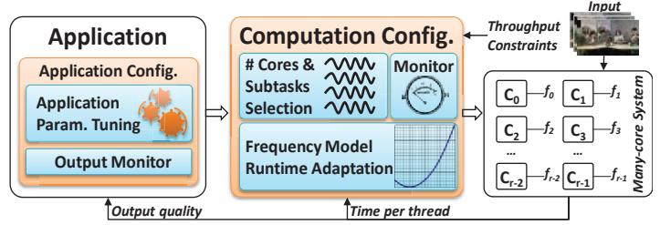
Figure 4-1: Overview of the proposed power-efficient workload balancing approach on a many-core system
