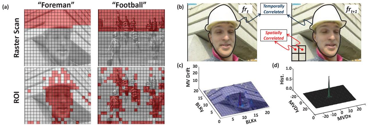
Figure 3-10: (a) Selected blocks (BLKs) at encoder for ME, in raster-scan and ROI order, (b) Spatial and temporal correlation among blocks of two frames ( $fr$ ), (c) Motion Vector Drift (MVD) and (d) Occurrence frequency of MVD for the “Foreman”
