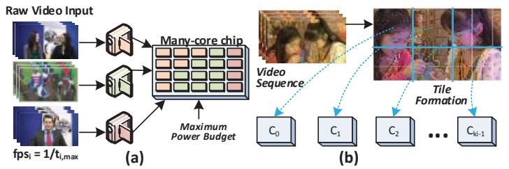
Figure 2-11: (a) Multi-video capture and encoding on a many-core chip,
