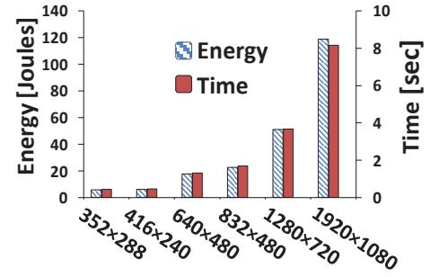
Figure 3-2: Energy and time consumption for HEVC Intra-encoding on x86 core
