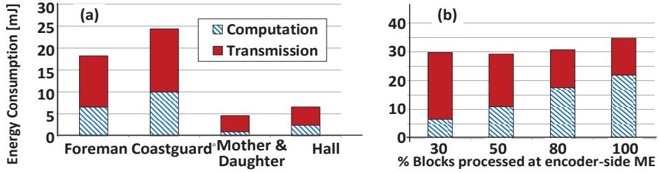
Figure 3-9: Analyzing the energy distribution for (a) different video sequences and (b) different number of MBs processed for ME
