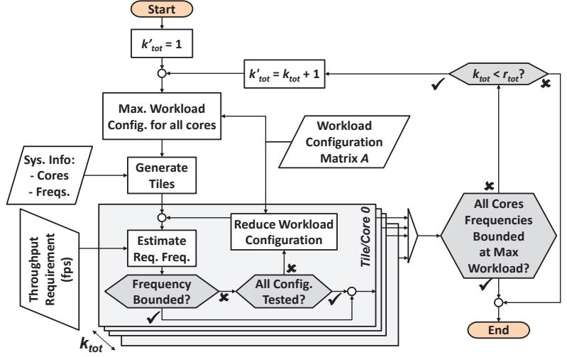
Figure 4-3: Uniform tiling, frequency and workload selection.
