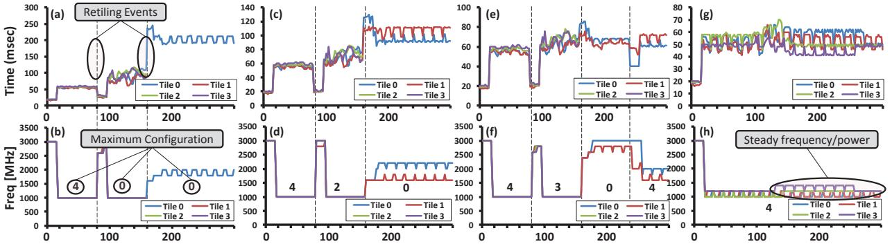
Figure 6-6: Cores' time, frequency and maximum configuration, per frame for frame interpolation with allowed number of cores ( $r_{tot}$ ) = 4: (a,b) FPS = 5 (c,d) FPS = 10 (e,f) FPS = 15 (g,h) FPS = 20
