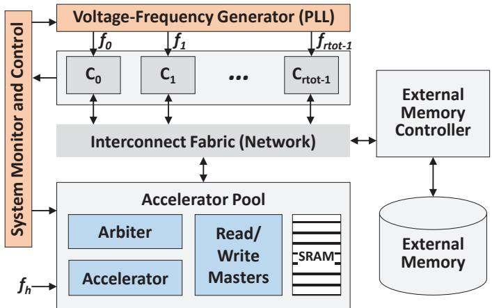
Figure 5-4: Power-efficient accelerator allocation
