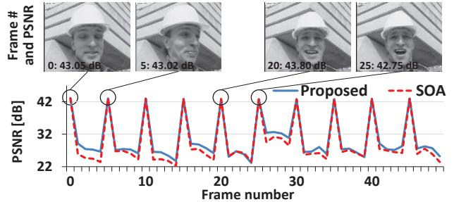
Figure 6-14: PSNR of the proposed scheme compared with the State-of-the-Art (SOA) [4], with same transmission energy and GOW size of 5 video frames (1 IF and 4 WF)
