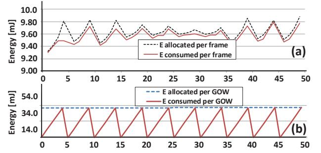
Figure 4-27: Proposed and consumed energy per (a) frame and (b) GOW
