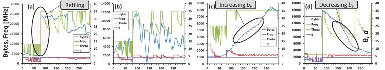
Figure 6-5: HEVC Frequency and workload tuning with the output bytes, for (a) Tile 1 of “ChinaSpeed”, (b) Tile 0 of “Keiba”, (c) Tile 0 and (d) Tile 7 of “BQTerrace”
