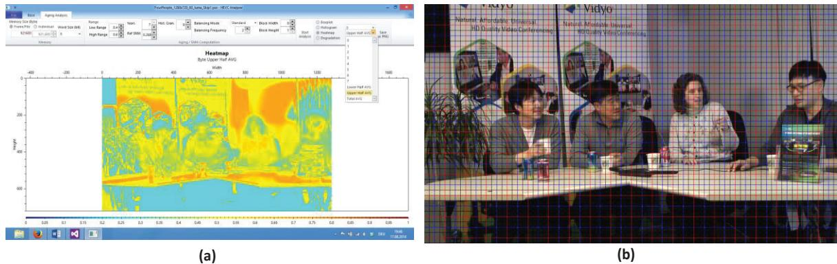
App-Figure D-2: (a) Visualizing the stressmap of “FourPeople” sequence and (b) 16×16, 32×32 and 64×64 grid overlaid on the video.
