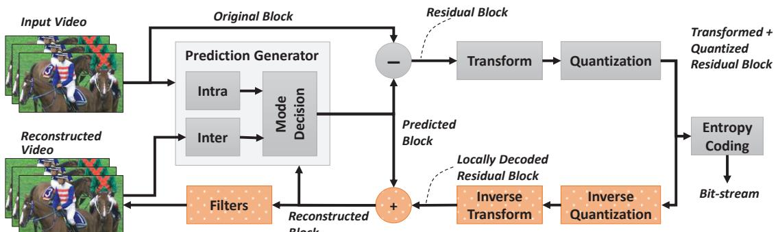
Figure 2-3: Basic modules of video encoder. The gray boxes are used for encoding purposes and the orange boxes denote the local decoder modules used inside the encoder.
