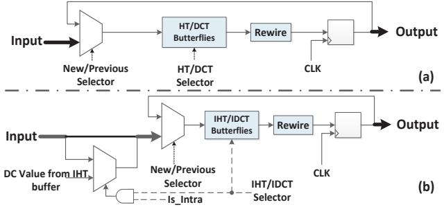
Figure 5-13: Folded design of (a) DCT and (b) IDCT
