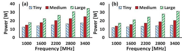
Figure 3-11: Power-frequency profiles for (a) DCT and (b) Quant
