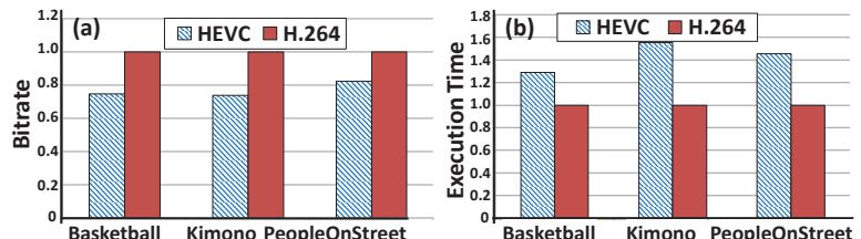
Figure 3-6: Comparing H.264-Intra to HEVC-Intra for relative (a) bit-rate and (b) execution time for different video sequences
