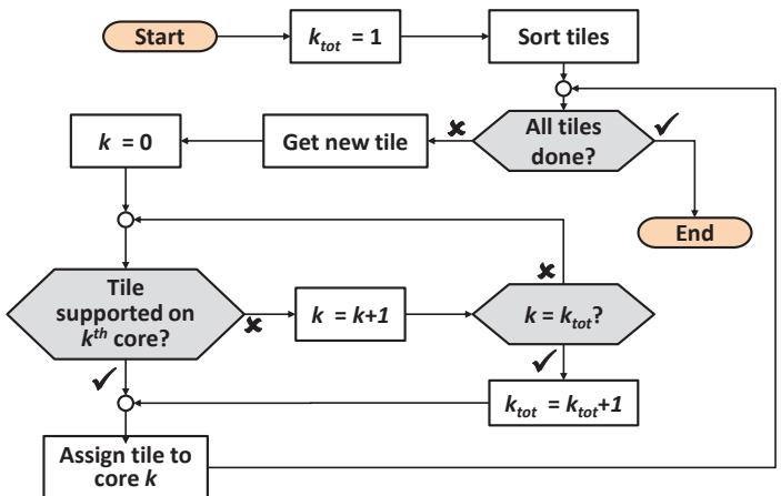
Figure 4-5: Tile-to-core assignment heuristic for non-uniform tiling.
