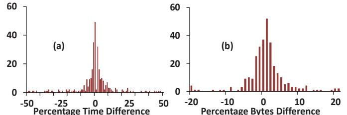
Figure 3-4: Percentage difference histogram of (a) time and (b) bytes for collocated tile number 0 of “Foreman” sequence ( $352 \times 288$ ) for 300 frames
