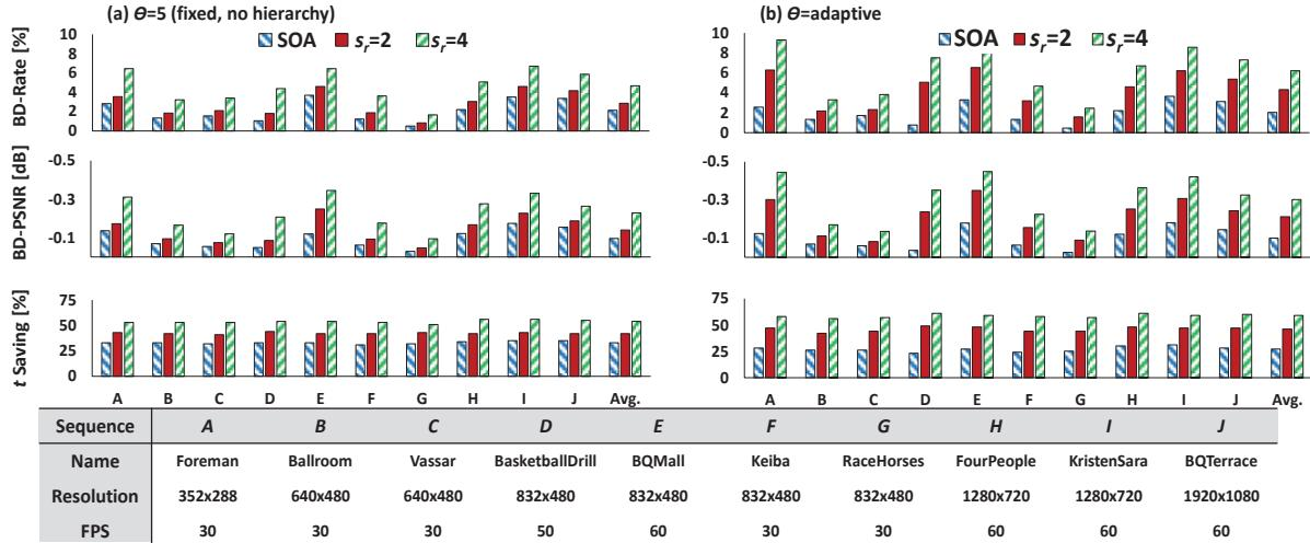
Figure 4-13: Comparison of video quality (BD-Rate and BD-PSNR [59]) and time savings for the proposed mode estimation approach with State-of-the-Art (SOA) [123] for (a) fixed and (b) adaptive number of angular modes
