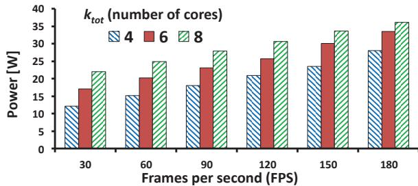
Figure 5-6: Power consumption of the programmable cores for the given FPS requirement and different number of cores
