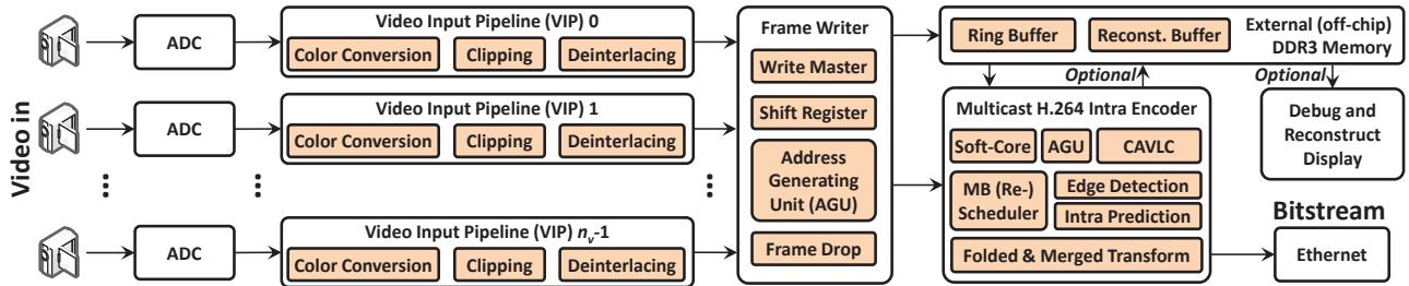
Figure 5-8: Overview diagram of the multicast H.264/AVC Intra-only encoder
