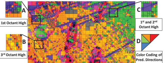
Figure 3-8: Color-coded intra angular directions per PU on 2<sup>nd</sup> frame of “BasketBallDrill” with CTU of 64×64
