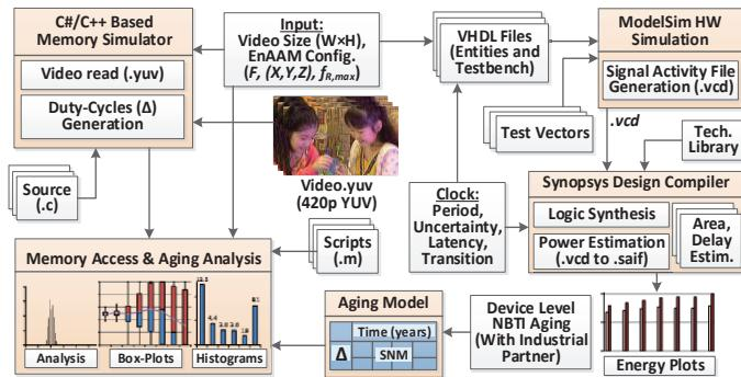
Figure 6-17: Experimental setup showing different hardware and software components for analyzing aging of SRAM circuits.
