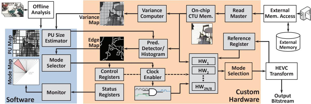
Figure 5-20: Hardware-software collaborative control for complexity and power reduction of HEVC Intra encoding
