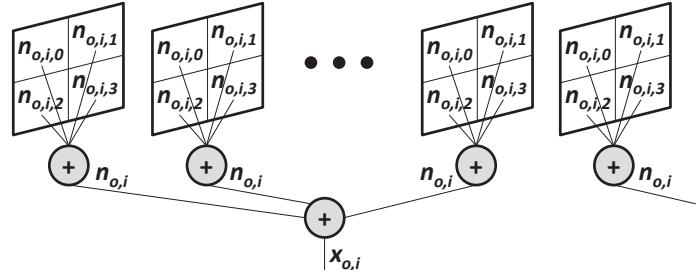
Figure 4-20: Concept of misprediction or offset used in this work. An example 4-core cluster is shown, where each core processes a single subtask and gives subtasks offset  $n_{o,i,j}$ .
