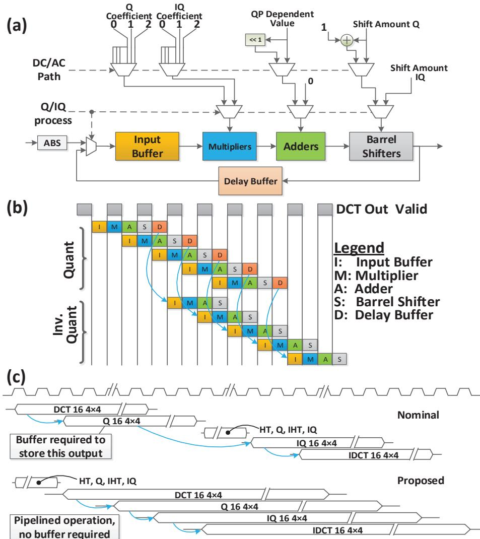
Figure 5-15: (a) Interlaced quantizer and inverse quantizer, (b) scheduler of quantizer/inverse quantizer and (c) scheduler of (inverse) transform and (inverse) quantization using nominal and proposed architectures
