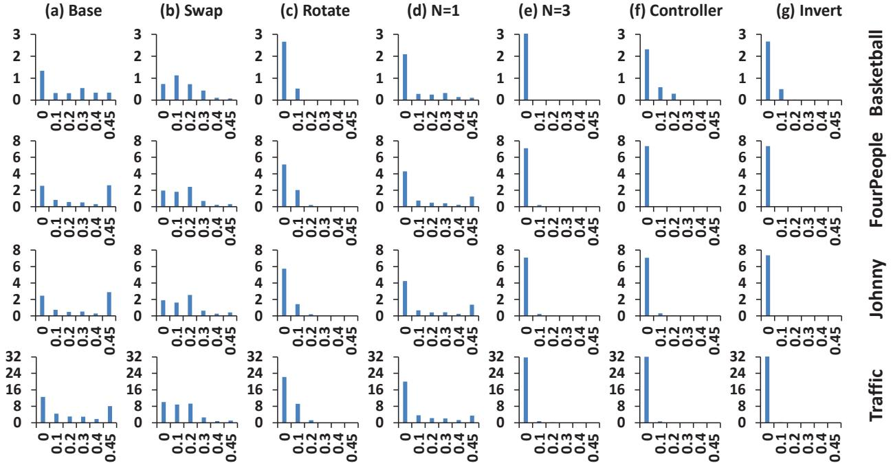
Figure 6-18: Histogram of duty cycle per bit, for a single frame memory partition with different comparison partners as given in Table 6-5. Values on x-axis denote the value  $\delta$  as given in by Table 5-4. The y-axis denotes total number of bits in millions. The best aging balancing is achieved when the histogram is crowded towards 0. For all (excluding the base and adaptive controller case), every second frame is adapted ( $f_R = 1$ ).
