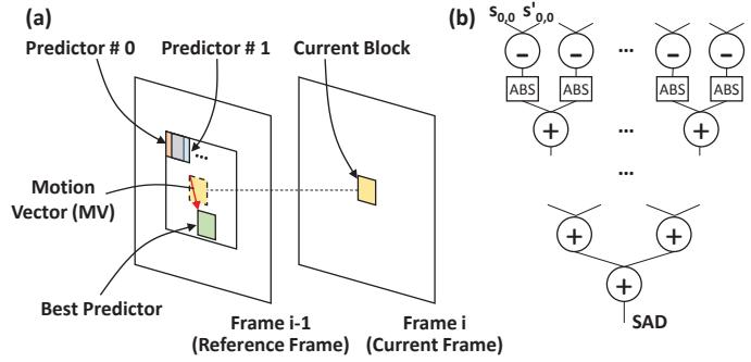
Figure 2-8: Motion estimation process and SAD computation
