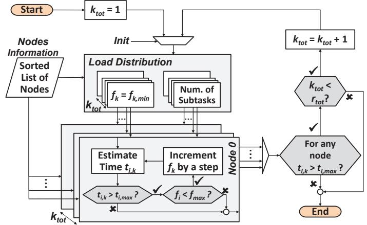
Figure 4-16: Workload distribution and balancing on heterogeneous nodes.
