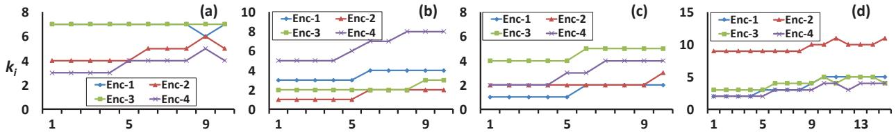
Figure 6-10: Runtime allocation (per epoch) of number of threads/cores for encoders at  $p_{tot}=100$  Watts ( $\sim 15\%$  DS) of (a) Set-1, (b) Set-2, (c) Set-3,(d) Set-4.
