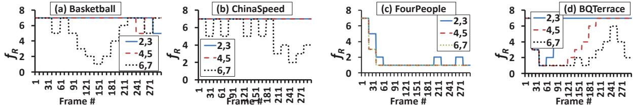
Figure 6-19: Runtime adaptation of  $f_R$  by the proposed aging controller with  $n_i=5$ ,  $(\tau_1, \tau_2, \tau_3) = (0.75n_i, 0.50n_i, 0.25n_i)$ ,  $F=20$ . Minimum  $f_R=1$ , maximum  $f_R=8$ .  $s_L=(1-\varepsilon)\times s_{init}$  and  $s_H=(1+\varepsilon)\times s_{init}$  where  $\varepsilon$  for bits (3,5,7) = (1/64, 1/32, 1/8).
