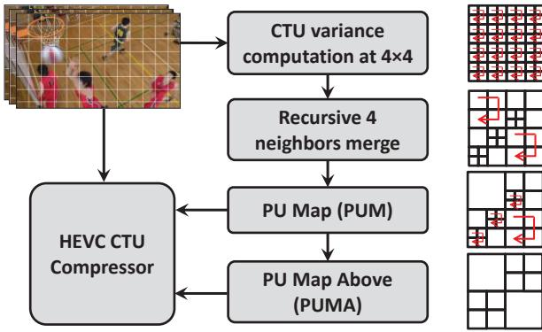
Figure 4-14: PU structure determination process
