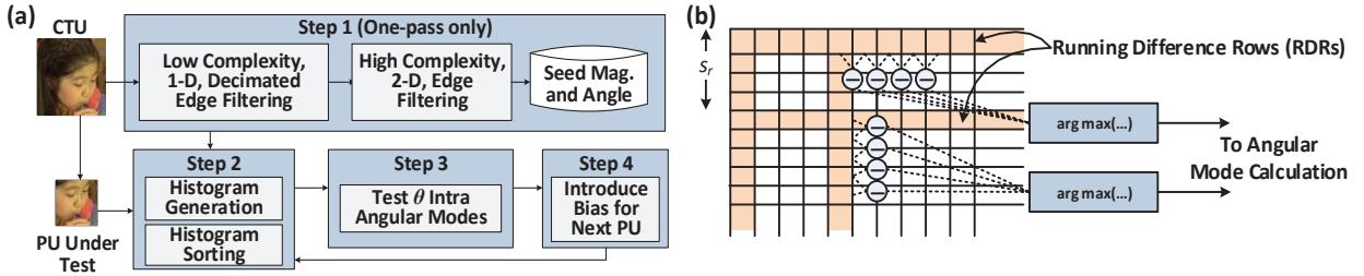
Figure 4-12: (a) Proposed fast Intra angular mode estimation, (b) Seed pixel extraction process for  $r_d=4$
