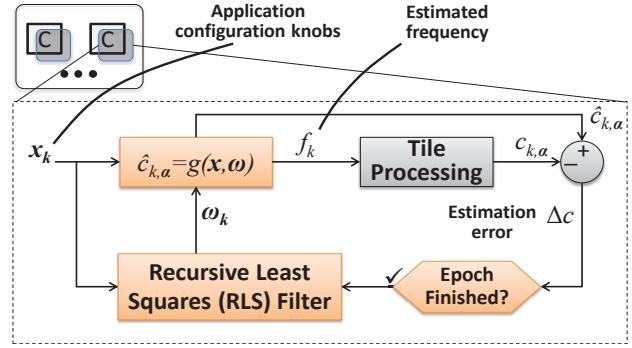
Figure 4-9: Per core frequency estimation model
