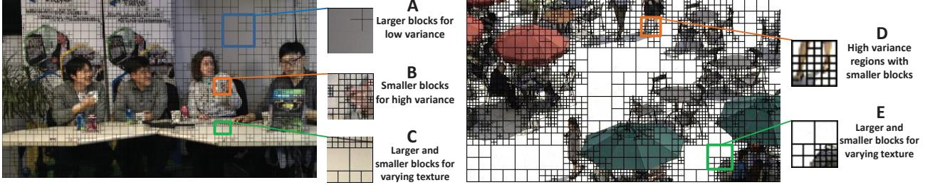
Figure 3-7: PU borders on the 4<sup>th</sup> frame of “FourPeople” and 31<sup>st</sup> frame of “BQSquare” video sequence
