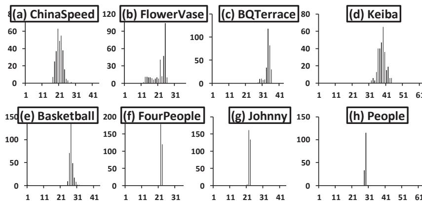
Figure 3-13: Percentage histogram of SRAM memory overwritten with new bits by video sequences. X-axis presents the percentage of bits changed in the subsequent frames, y-axis presents the number of times a certain percentage occurs for 300 continuous frames.
