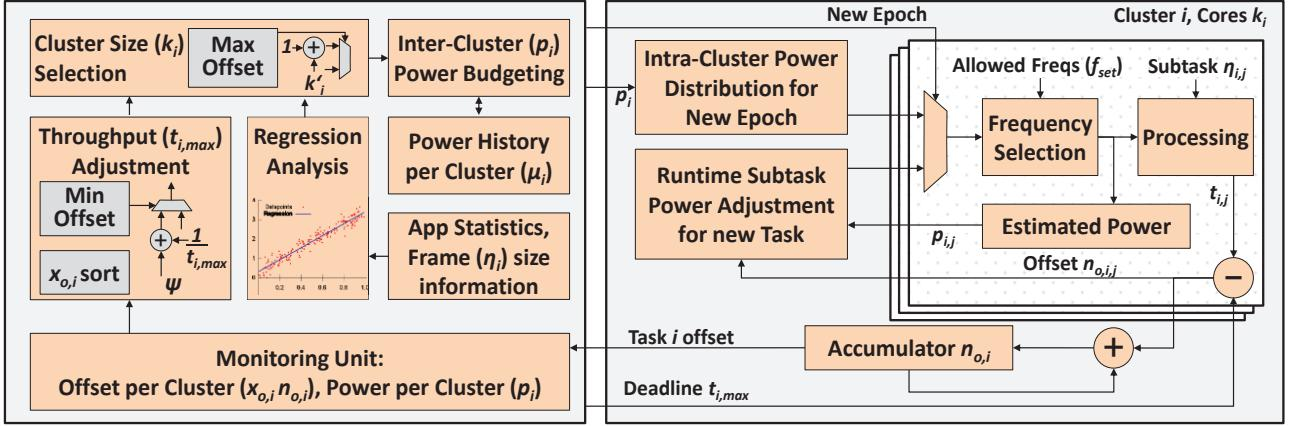
Figure 4-19: Details of the proposed multi-granularity power budgeting scheme. For simplicity, only one task is shown.
