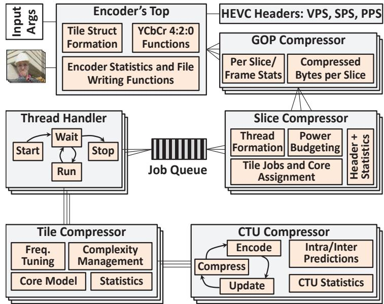
App-Figure B-1: Software architecture of ces265. The Encoder's Top object can have multiple GOP Compressor objects. Each GOP Compressor object can have access to multiple Slice Compressor objects. With each Slice Compressor object, a Workload Queue object is associated, with can be accessed by multiple Thread Handler objects.
