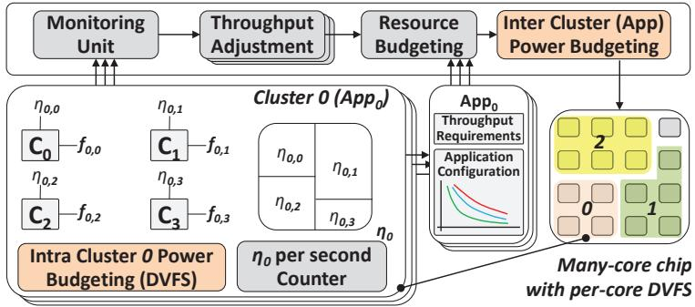
Figure 4-17: Overview of resource budgeting for mixed multithreaded loads.
