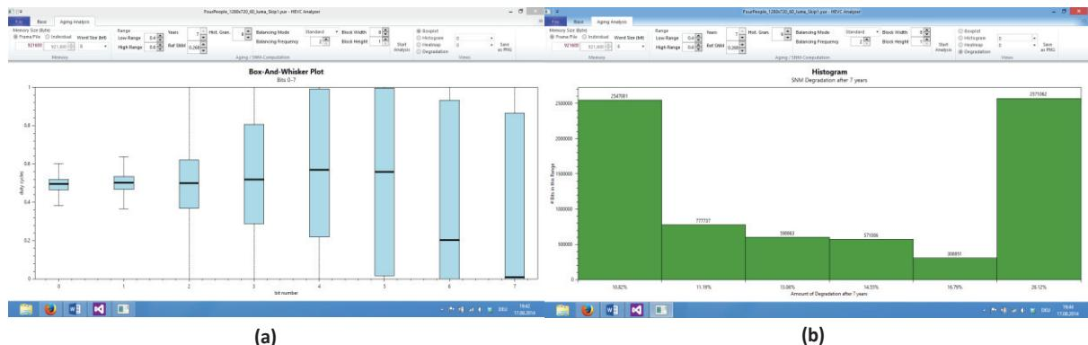
App-Figure D-3: (a) Box-plot of duty-cycles for all bits and (b) SNM degradation histogram.
