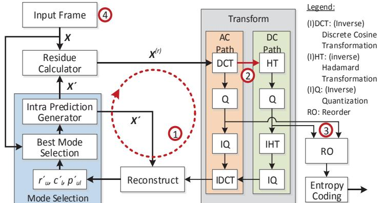
Figure 5-10: H.264/AVC Intra processing loop architecture. The current MB is labelled as  $X$ , the predicted and residue MBs are labeled  $X'$  and  $X^{(r)}$ ; sequential data dependencies are shown by dashed arrows (① and ②)
