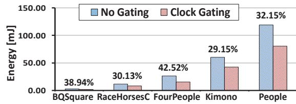
Figure 5-21: Average Energy consumption for one frame
