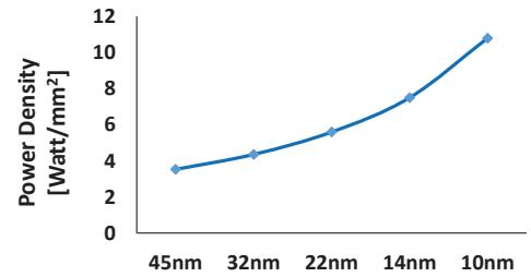
Figure 1-5: Power density for different fabrication technologies [36]
