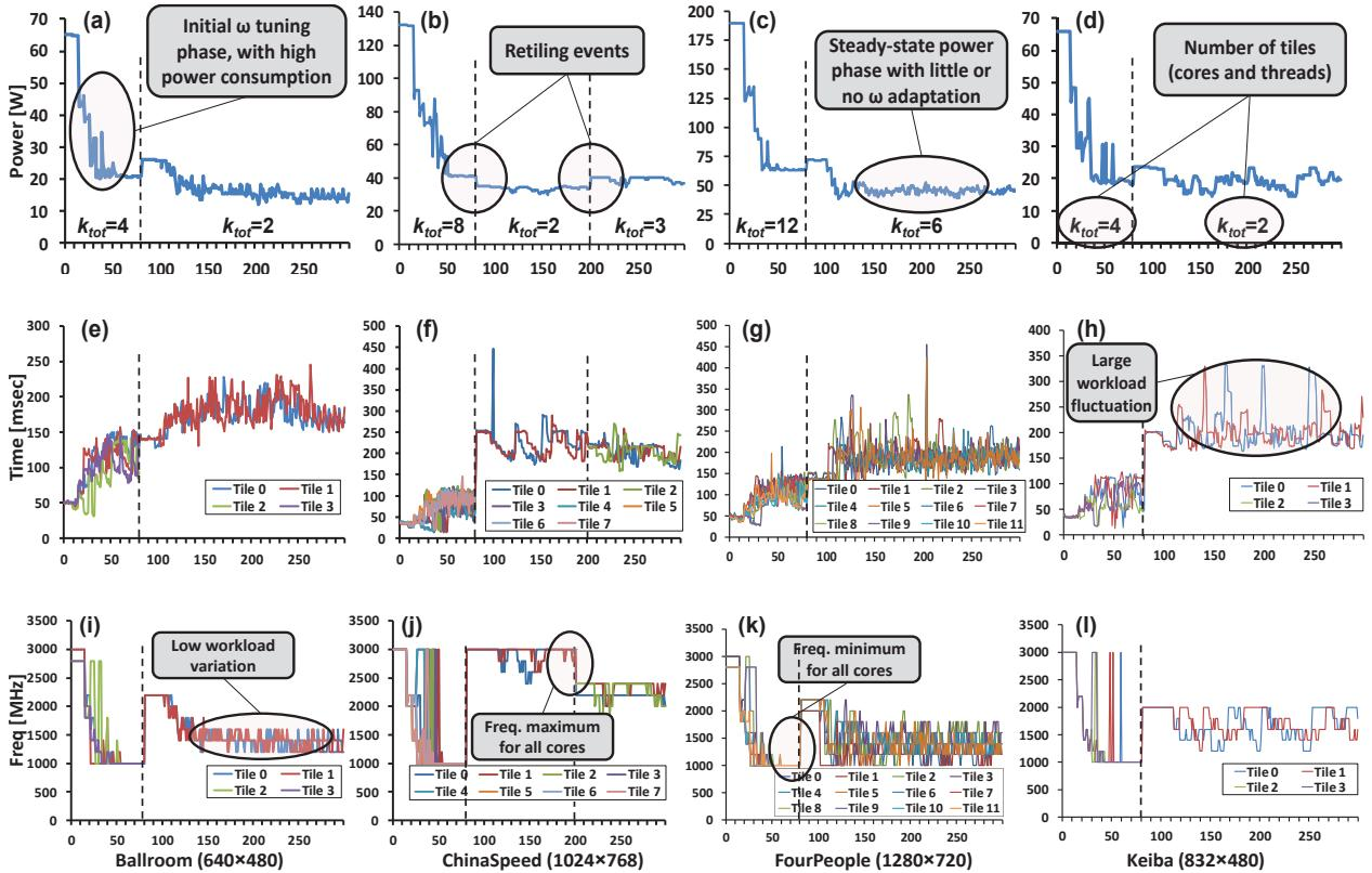
Figure 6-4: (a-d) Power [W], (e-h) time per tile [msec] and (i-l) frequency per tile [MHz] for different video sequences, using  $f_p=5$  and  $\varepsilon=0.05$  or 5%
