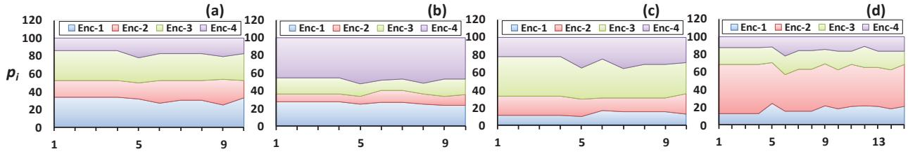
Figure 6-11: Stacked area plot for Inter-cluster, runtime power (in Watts) for encoders at  $p_{tot}=100$  Watts, ( $\sim 15\%$  DS) of (a) Set-1, (b) Set-2, (c) Set-3, (d) Set-4
