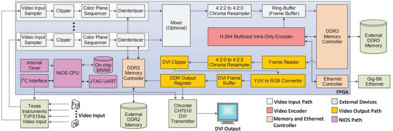
App-Figure C-2: Prototype architecture on Altera's Arria II GX FPGA. For complete system implementation of H.264 Intra-only
