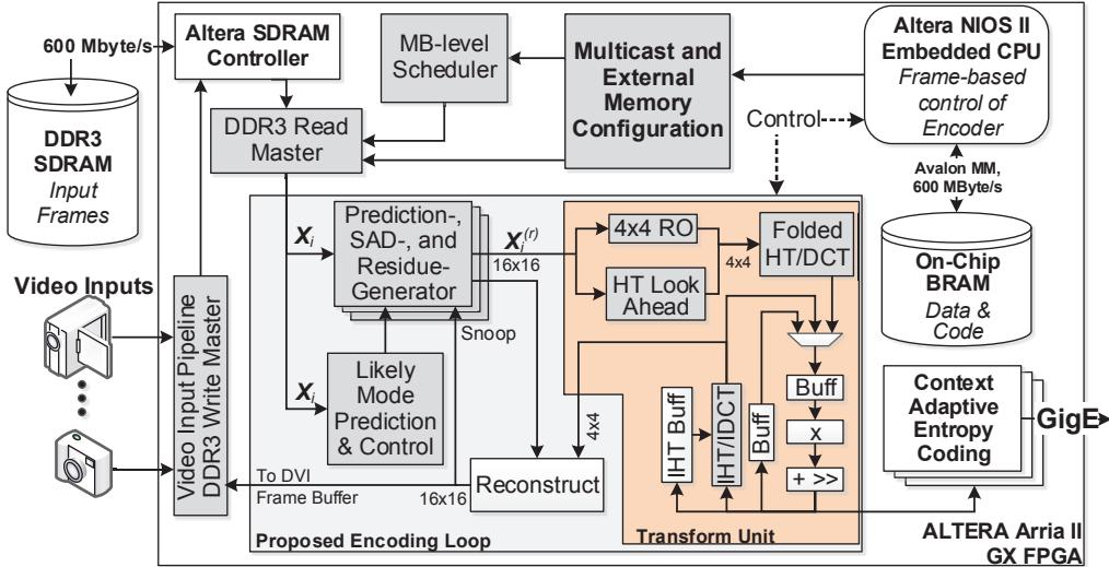
Figure 5-11: Proposed hardware accelerator architecture for multicast H.264/AVC Intra video encoder. This design also shows the connections of the multicast encoder with the I/O ports of the system
