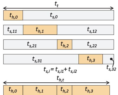
Figure 5-5: Breakdown of an example execution time on a 4-core system and a shared accelerator
