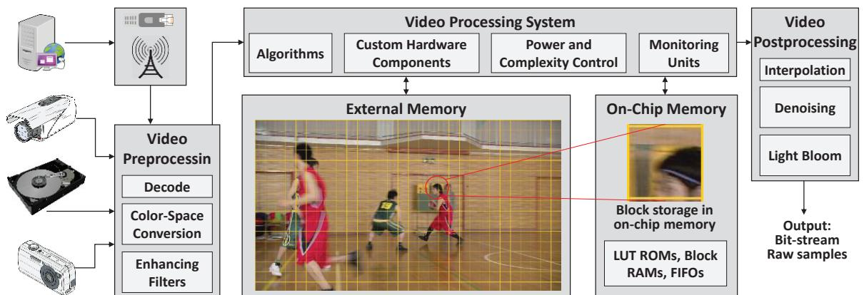
Figure 2-1: Basic video processing system. The frame is divided into blocks and logically stored in the external memory as shown in the figure. A block of size  $b_w \times b_h$  is processed at a time
