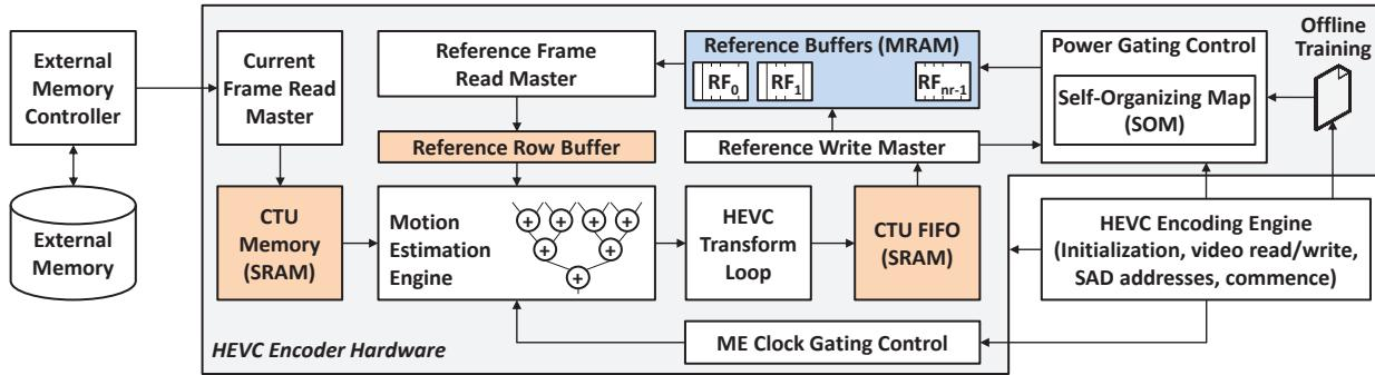
Figure 5-22: AMBER system architecture for HEVC video encoder
