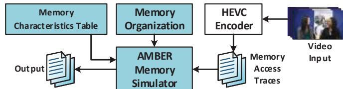
Figure 6-15: Hybrid memory simulation setup.
