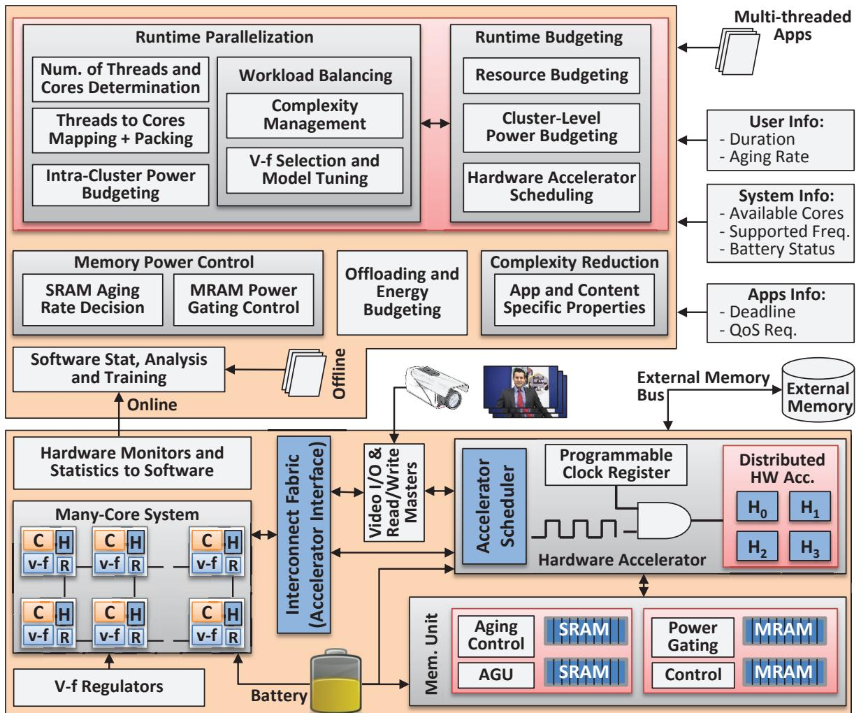
Figure 3-1: Software and hardware layers of the proposed multimedia system.
