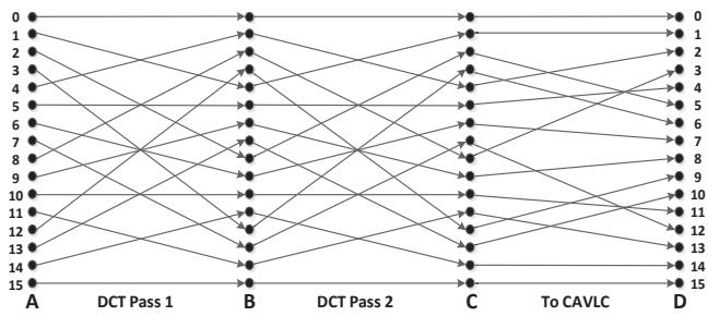
Figure 5-14: Data flow graph from the output of HT/DCT butterflies to the input of the entropy coder
