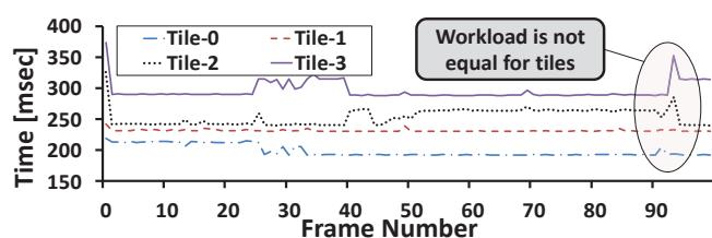
Figure 3-5: Time consumption of each tile ( $2 \times 2 = 4$  tiles per frame) of Non-Local Means Filter for “Foreman” sequence ( $352 \times 288$ )
