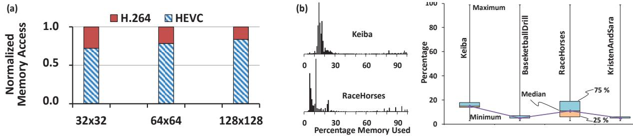
Figure 3-12: (a) ME memory access comparison between H.264/AVC and HEVC for three search window sizes, (b) ME memory access percentage statistics for TZ search in HEVC
