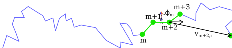
Figure C.2.2.: For the calculation of the first order dihedral derivatives, the change of the vector from atom m + 1 to atom i upon a change of the dihedral angle \phi_m is analyzed.
