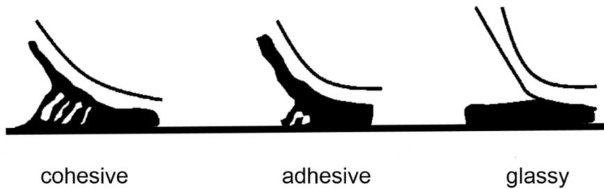
Figure 9. Failure mode explanation in a 90° peel test.<sup>[27]</sup>
