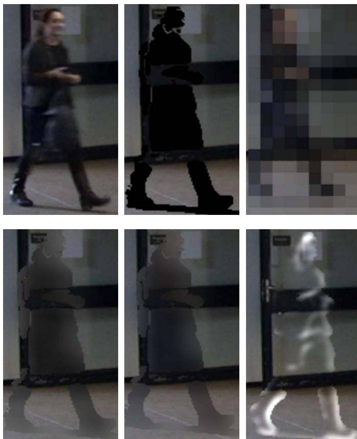
Figure 7.1: Anonymization functions: original, silhouette, pixelization, gray-scale blurring, blurring, edge detection
