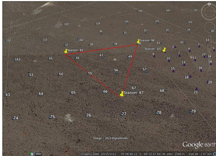
Figure 5.10.: Positions of the four prototype stations deployed at the Auger site. Three tripole stations with LOPES 3D antennas with station number 87, 91 and 98 and one low-frequency station with station number 107 have been deployed from 15 November 2013 till 22 November 2013.
