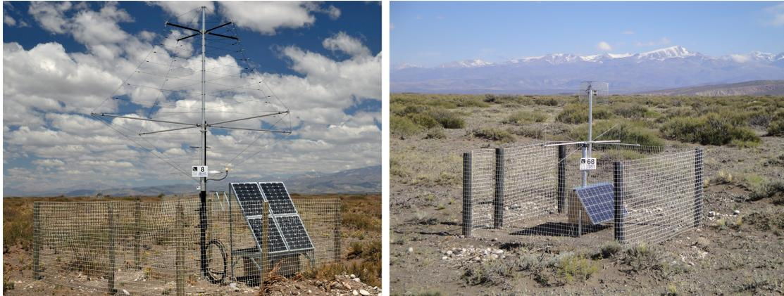
Figure 3.8.: Picture of one LPDA station on the left and picture of one Butterfly station on the right [68].
