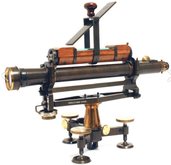
(a) Kern precise levelling instrument, since 1864, image source: Stadtmuseum Aarau (2015)
