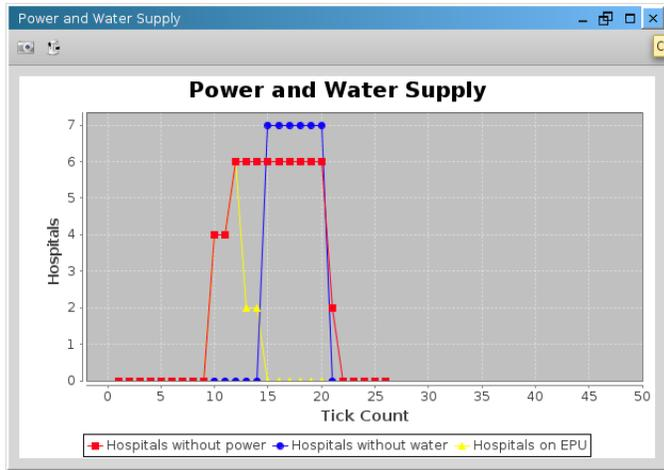
Fig. 3. Time dependent status of hospitals (EPU = emergency power generators), red means the number of hospitals without power, blue without water and yellow number of hospitals where the emergency power is on
