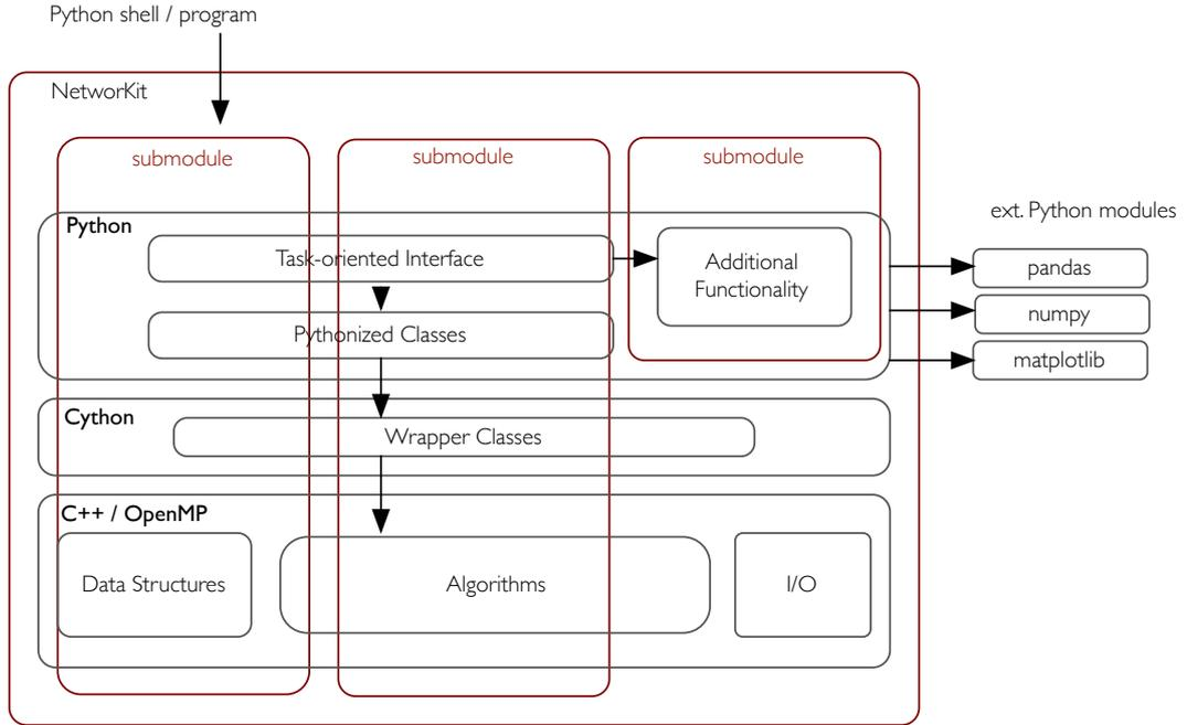
Figure 10: NetworkKit architecture overview ( $\rightarrow$  represents call from/to)
