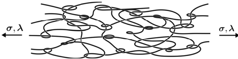
Figure 3.4.: Stretched and oriented polymer chains
