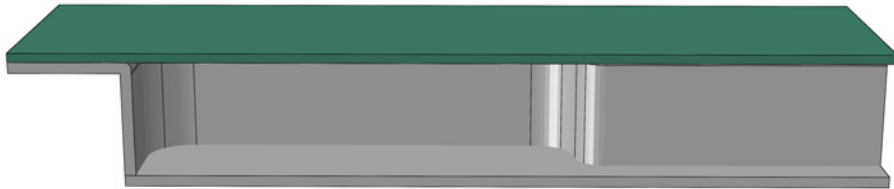
(a) 3D model of film is initially placed on the mold
