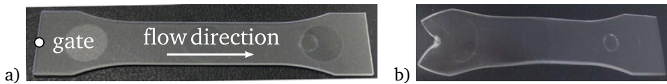
Figure 4.19.: Injection molded tensile test specimen: a) initial state with indicated gate and flow direction, b) deformed state after heating to 120 °C
