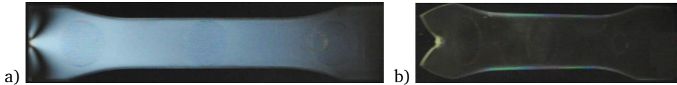
Figure 1.3.: Molecular stretch and orientation in the injection molded test specimen made visible due to birefringence under polarized light (left). No orientation is visible after heating above glass transition temperature (right).
