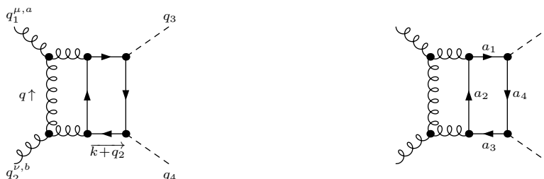
Figure 3.7: Process definitions for a sample IR divergent diagram. Left: momentum assignment of the propagators. Right: Denominator assignment for the Feynman parametrisation of eq. (3.34).
