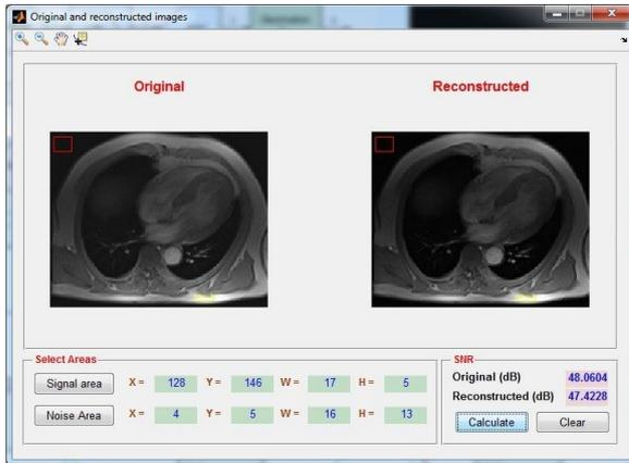
**Figure 4.6:** GUI of a Matlab program used to compare the original and the reconstructed MR image. It also determines the SNR of identical user-selectable regions of interest in both images, indicated here by yellow (signal region) and red (noise region) rectangles via equation 4.2.
