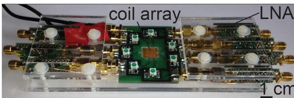
**Figure 2.18.:** Phased array of several hexagonally wire bonded micro coils [36]. The phased array of micro coils with tuning and matching electronics is mounted on a PCB. Seven low-noise preamplifiers are connected to the phased array.
