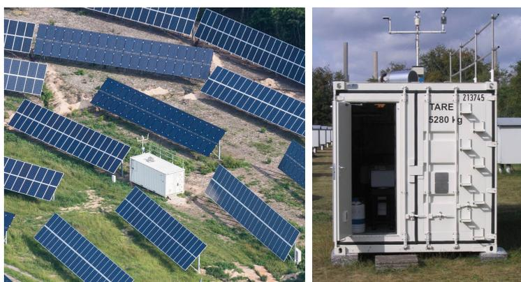
**Figure 3.1:** Aerial photograph of the Karlsruhe FTS site at the Campus North of the KIT (left panel) and the certified shipping container wherein the spectrometer is hosted (right panel). Photograph courtesy of KIT (left panel) and F. Hase (right panel).
