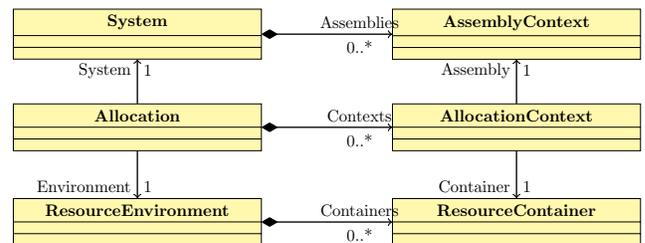
Figure 11: A simplified metamodel excerpt of PCM for deployment
