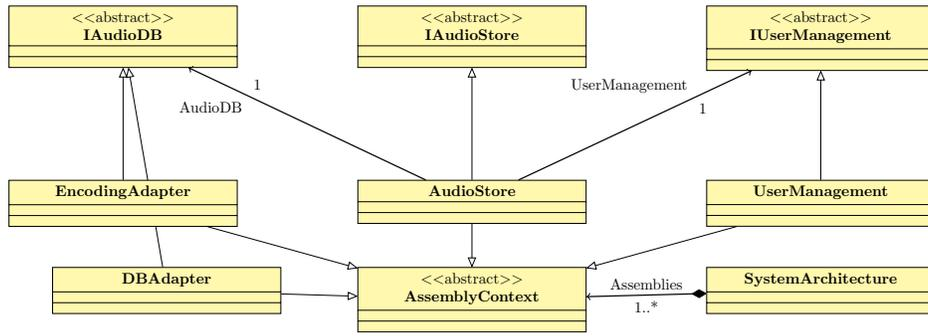
Figure 10: Excerpt of the implied DeepADL metamodel to specify the architecture of a MediaStore system based on a repository of component types
