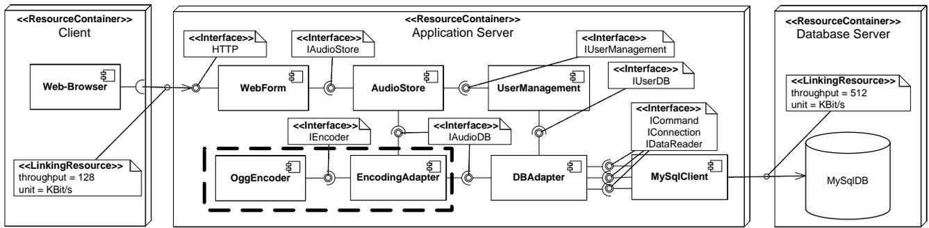
Figure 8: The software architecture of the MediaStore [6]
