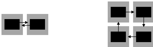
Figure 2.10: Deadlock because of opposing routes (left) and because of boxes waiting in a loop (right)
