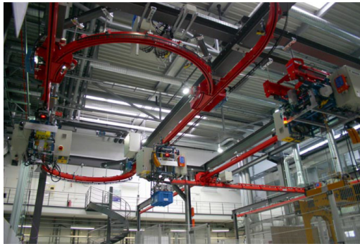
Figure 2.7: Photograph of electric monorail system (Chisu et al. 2010)
