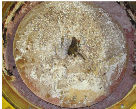
Full-scale block #32 after 26.7 years exposure in NaCl solution
