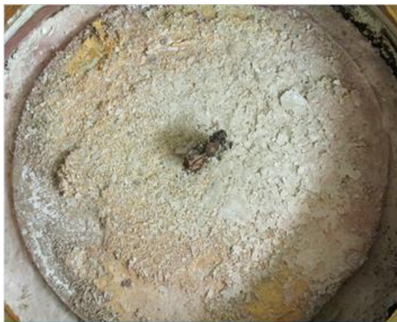
Full-scale block #35 after 25.3 years exposure in NaCl solution
