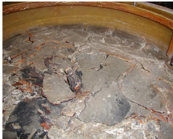
Full-scale block #33 after 17.1 years exposure in MgCl_2 solution
