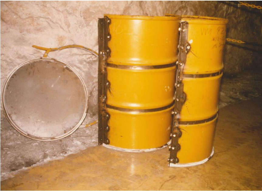
Fig. 3 Photo of the mould used to prepare cement blocks #20 to #36.
