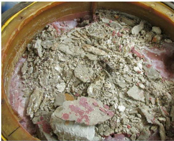
Full-scale block #36 after 23.3 years exposure in MgCl_2 solution
