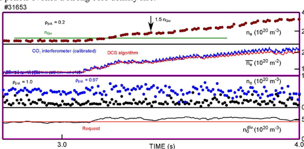
Figure 2: Controlling the divertor neutral gas pressure keeps the local edge density (close to separatrix at  $p_{pol} \approx 1.0$  and pedestal top at  $p_{pol} \approx 0.97$ ) constant. The increase of the validated line average density correlates well with the evolution of the core density at  $p_{pol} \approx 0.2$ .
