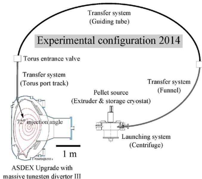
Figure 1: Set up as operated in the campaign 2014. AUG with an all W clad wall and now also equipped with the massive tungsten divertor III and the full set of B coils. The revitalized pellet launching system was optimized and commissioned for efficient particle fuelling from the torus inboard at high speed and high particle throughput. As well, admixing different gases to the main fuelling species (mostly deuterium) is now facilitated.
