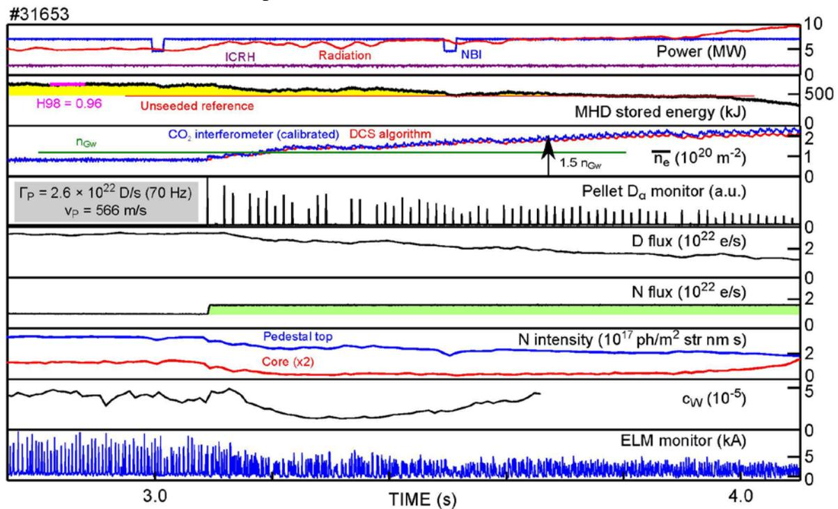
Figure 3: The N pump out can be mitigated by an increased N puffing rate during the high density phase. Thus, high density operation with benign ELM behavior and still higher confinement compared to the unseeded reference can be achieved.
