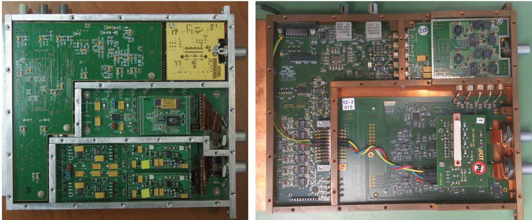
Figure 2.18: Two opened detector readout and biasing units, *bolometer boxes*. An older bolometer box version 1 in the left photo and the newer bolometer box version 2-3 including the upgrade for higher detector voltages in the right photo. Both boxes connect at the outer surface of the cryostat with the 3 connectors on the right side to the cold electronics. The digitized data is sent on the optical fibers to the DAQ crate. Further details in text.
