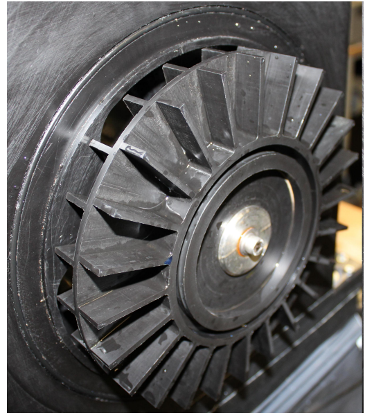
(b) Impeller (24 blades) mounted on POM Basis; Circumferential blade offset visible.
