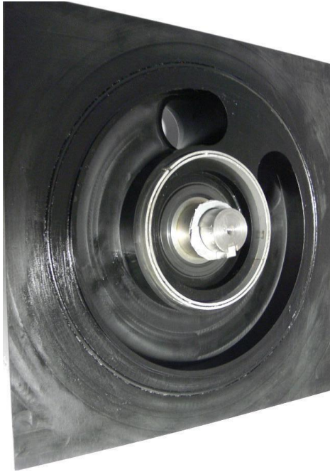
(a) POM Basis with milled side channel, shaft and circumferential labyrinth sealing.
