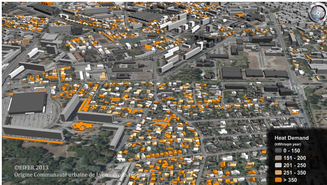
Figure 10: Results from building classification and steady-state heat demand calculation (Bahu, Koch et al. 2013)
