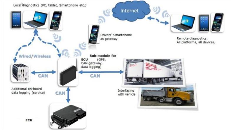
Figure 5: Schematic view of the architecture of a remote diagnostic system for online monitoring
