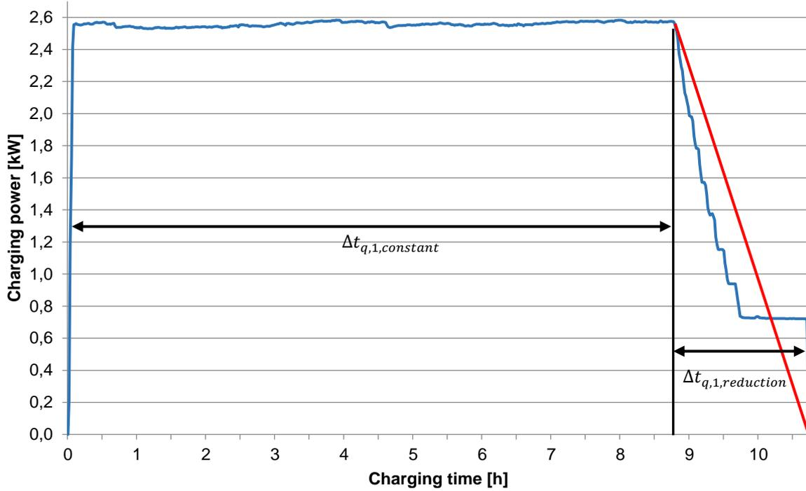
**Figure 3: Recorded charging curve of project EV (e-Wolf Delta 2) at domestic power outlet**
