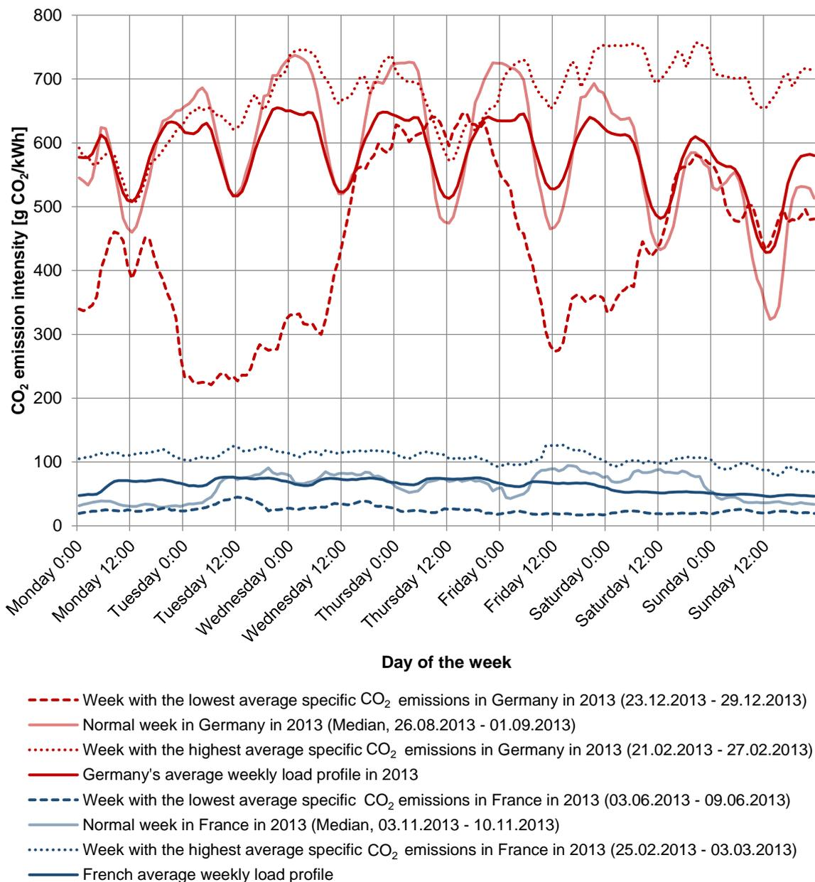
Figure 1: CO<sub>2</sub> emission intensities of electricity generation in France and Germany in 2013 (Sources: EEX Transparency, 2015; RTE, 2014)
