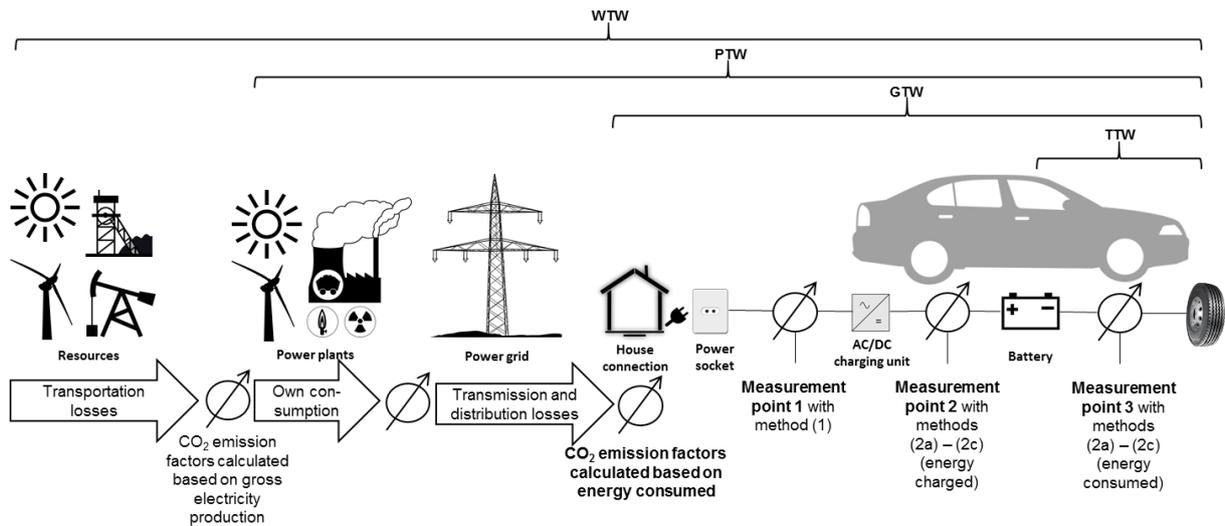
**Figure 2: Energy measurement points and methods in the energy supply chain for charging EV**
