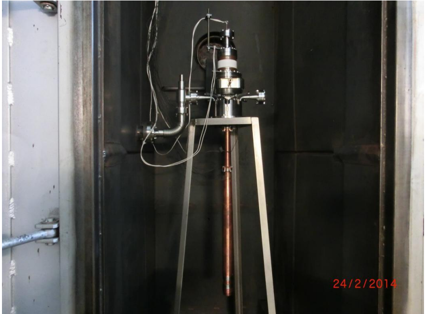
Figure 6.15: Photo of the gyrotron installed for the bake-out procedure inside the oven (at IHM)
